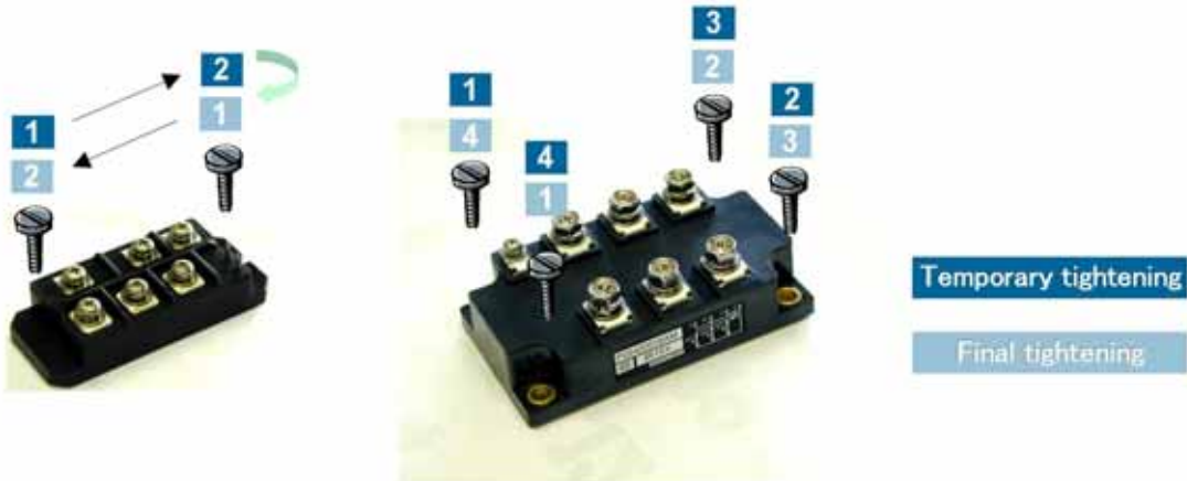
Sequence of tightening screws
