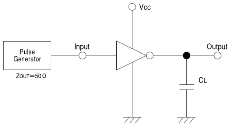
Note: Open output when measuring supply current
