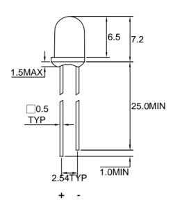
Note: 1.All dimension are in millimeter tolerance is  $\pm 0.25$ mm unless otherwise noted.
