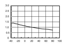
Fig.6 Relative Radiant Power vs. Temperature
