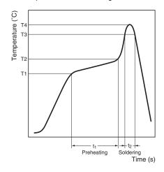
The thickness of cream solder to be applied should be within a range between 150 and 200 µm on OMRON's recommended PCB pattern.
