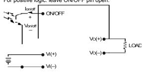
Figure 20. Circuit configuration for using Remote On/Off Implementation.
