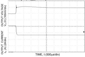
Figure 14. Typical Transient Response to Step decrease in Output Load from 8.1A to 5.3A at Room Temperature and 48 Vdc Input;  $C_{o,ext}$  = 370 µF.
