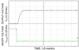
Figure 12. Typical Start-Up Using Remote On/Off,
