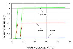
Figure 9. Typical Input Characteristic at Room
