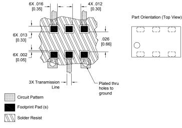
Dimensions are in Inches [Millimeters] Mounting Footprint
