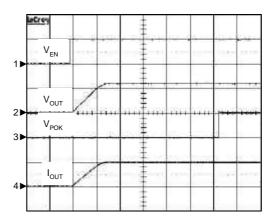
$$\begin{split} &C_{\text{OUT}} \! = \! 10 \mu \text{F}, \, C_{\text{IN}} \! = \! 10 \mu \text{F}, \, R_{\text{L}} \! = \! 1.2 \Omega \\ &\text{CH1: V}_{\text{EN}}, \, 5 \text{V/Div, DC} \\ &\text{CH2: V}_{\text{OUT}}, \, 1 \text{V/Div, DC} \\ &\text{CH3: V}_{\text{POK}}, \, 5 \text{V/Div, DC} \\ &\text{CH4: I}_{\text{OUT}}, \, 1.0 \text{A/Div, DC} \\ &\text{TIME: 0.5 ms/Div} \end{split}$$
