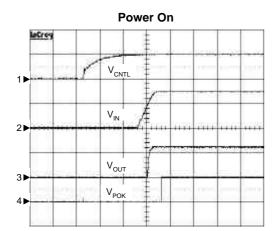
$C_{OUT}$ =10 $\mu$ F,  $C_{IN}$ =10 $\mu$ F,  $R_L$ =1.2 $\Omega$ CH1:  $V_{CNTL}$ , 5V/Div, DC CH2:  $V_{IN}$ , 1V/Div, DC CH3:  $V_{OUT}$ , 1V/Div, DC CH4:  $V_{POK}$ , 5V/Div, DC
