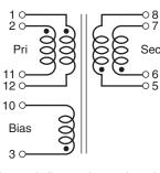
Primary windings and secondary windings to be connected in parallel on PC board.
