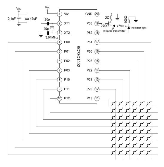
Note: 1. The connections of the two capacitors with VDD should be as close as possible to the application circuits.
