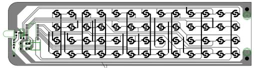
The transmitting tube ground line and IC ground line should layout separatedly or overstriking the ground line.
