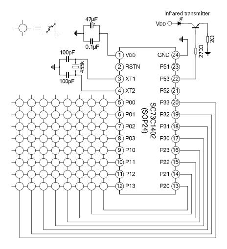
Note: 1. The connections of the two capacitors with VDD should be as close as possible to the application circuits.
