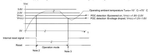
Notes1. VPOC is different in different conditions. When powered on, the VPOC value is VPOC1( VPOC1=1.8V~2.0V); when working, VPOC is approximately VPOC2 in normal conditions(VPOC2=1.2V~1.6V).
