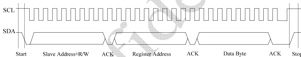
Figure 5: Serial Interface Slave Mode Protocol
