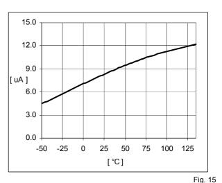
WDI Input Current Low-level I<sub>IL</sub> vs. Temperature (V<sub>DD</sub>=5.5V)
