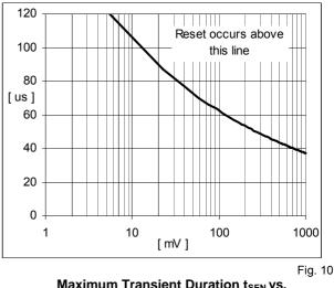
Maximum Transient Duration  $t_{SEN}$  vs. Overdrive  $V_{TH}$ - $V_D$
