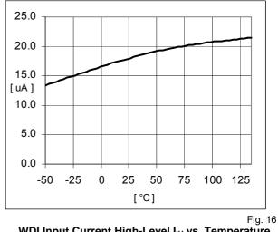
WDI Input Current High-Level I<sub>IH</sub> vs. Temperature  $(V_{DD}=5.5V)$
