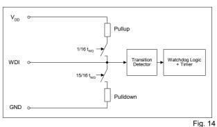
WDI Input Stage Block Schematic
