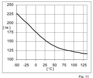
Watchdog Input Pulse Width twp vs. Temperature
