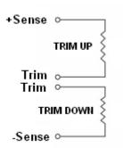
The output voltage can be adjusted by connecting trim resistors as shown.
