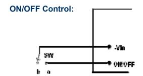
The converter output can be disabled by moving SW to position "a"—connected to –Vin with voltage level between -0.7 and 0.4V.
