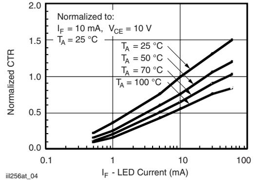
Fig. 4 - Normalized CTR vs.  $I_F$  and  $T_{amb}$
