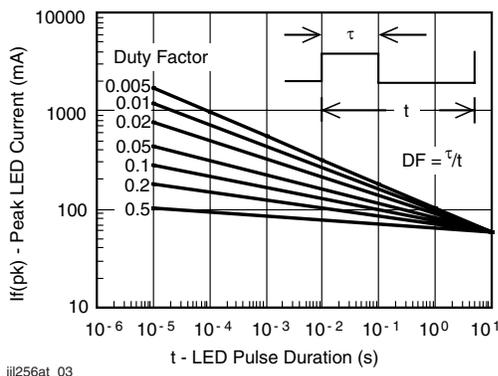
Fig. 3 - Peak LED Current vs. Duty Factor, Tau
