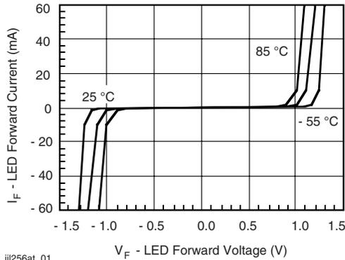
Fig. 1 - LED Forward Current vs. Forward Voltage
