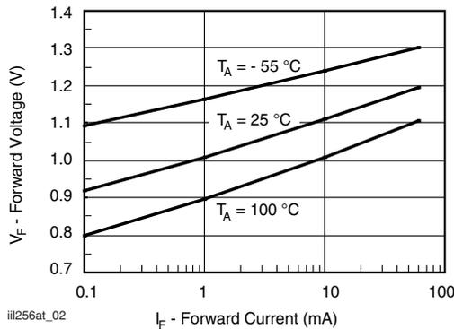
Fig. 2 - Forward Voltage vs. Forward Current
