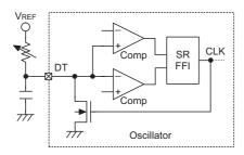
Fig.1 DT Oscillator Structure
