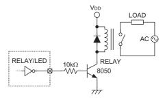
Fig.3 RELAY Pin Drive RELAY
