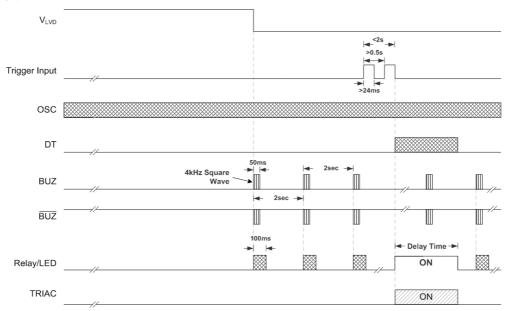
Fig.14 Trigger Timing of LVD
