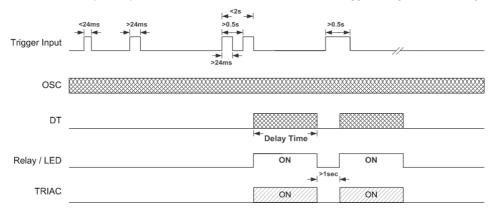
Fig.11 Trigger Timing
