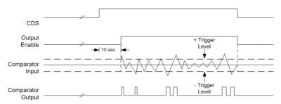
Fig.15 Trigger Timing of CDS
