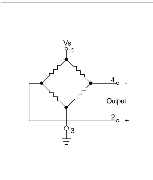
**PRESSURE SENSOR CHARACTERISTICS** $V_s = 10.0 \pm 0.01 \text{ V}$ ,  $t_{\text{amb}} = 20^\circ\text{C}$  (unless otherwise noted)
