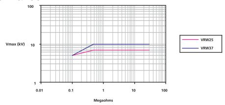
Maximum peak voltage in accordance with "IEC 60065 chapter 14.1" 50 discharges from a 1nF capacitor charged to V max. 12 discharges/minute.
