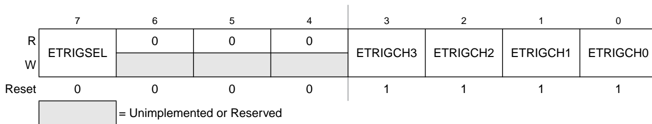
Figure 4-4. ATD Control Register 1 (ATDCTL1)
