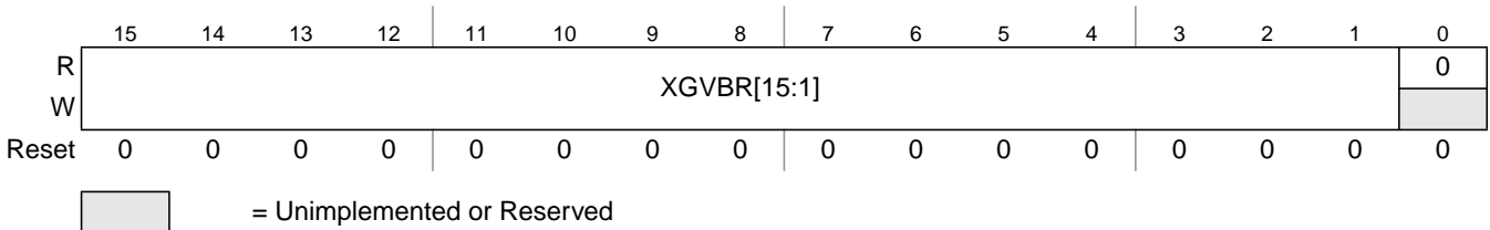
Figure 6-5. XGATE Vector Base Address Register (XGVBR)
