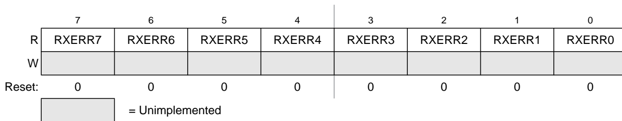
Figure 10-18. MSCAN Receive Error Counter (CANRXERR)
