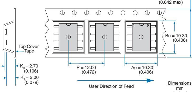
NOTE: Tape dimensions not shown comply with JEDEC Standard EIA-481-2
