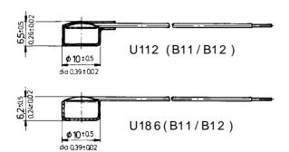
The temperature resistance of the connecting leads allows for the nominal response temperature of the cutout.
