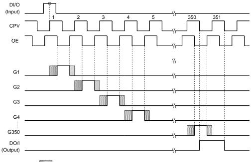
: This part is output which is controlled ( fixed to  $\mathsf{V}_{\textbf{EE}}$  ) by  $\ \overline{\mathsf{OE}}\$  pin
