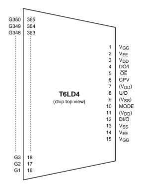
The above diagram shows the device's pin configuration only and does not necessarily correspond to the pad layout on the chip. Please contact Toshiba or our distributors for the latest COF specification.
