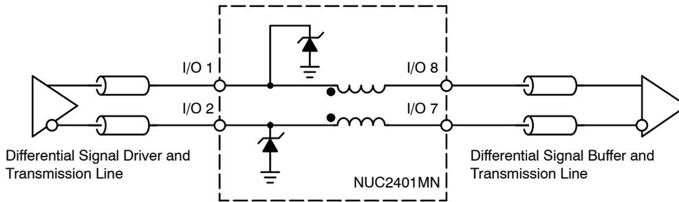
**Figure 4. Application Circuit**
