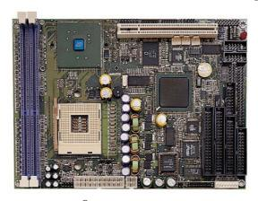
The HS-4701 is an Intel® 82845GE/82801DB chipset-based board designed for PCI Bus PGA 478 Intel® Pentium® 4 up to 2.4GHz(400MHz FSB)/3.06GHz(533MHz FSB) CPU compatibility. These features combine and make the HS-4701 an ideal all-in-one industrial single board computer. Additional features include an enhanced I/O with CRT/LVDS Panel, DIO, LAN, Audio and 4COM ports interface.
