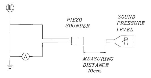
Mic : RION S.P.L meter UC30 or equivalent S.G : Hewlett Packard 33120A Function Generator or equivalent
