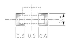
For Reflow Soldering (propose)
