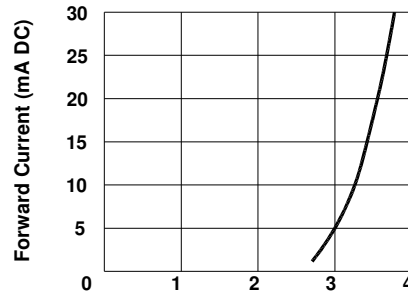
Forward Voltage VF (V) Fig 2. Forward Current Vs. Forward Voltage
