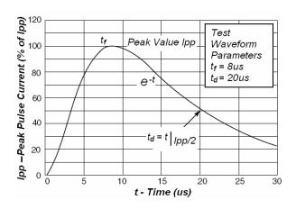
Fig2. Pulse Waveform
