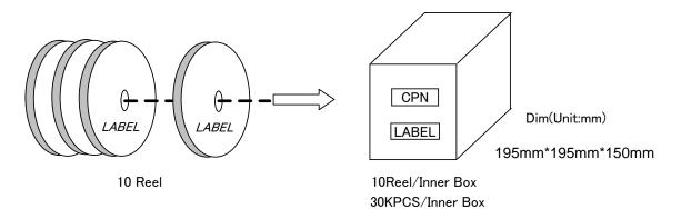
3000PCS/Reel 80KPCS/Inner Box (SOT-723,SOD-723,SOD-923) 8000PCS/Reel (SOT-723,SOD-723,SOD-923)
