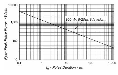
Fig1. Peak Pulse Power VS Pulse Time
