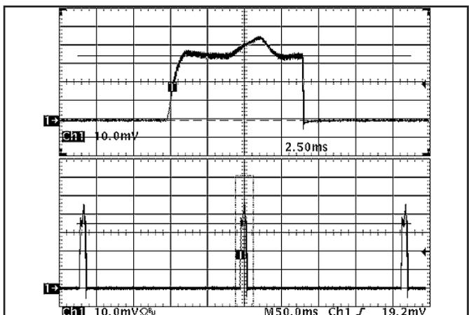
**Figure 18:** Load current (20A/div) as a function of time when the converter attempts to turn on into a  $1\ \text{m}\Omega$  short circuit. Top trace (2.5ms/div) is an expansion of the on-time portion of the bottom trace.
