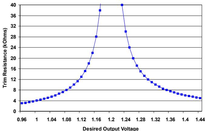
**Figure C: Trim Graph for 1.2V<sub>out</sub> module**
