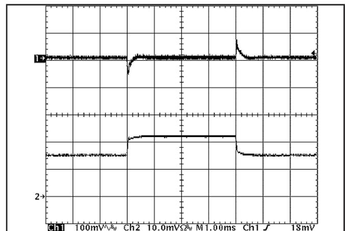
Figure 12: Output voltage response to step-change in load current (50%-75%-50% of I<sub>out</sub>(max); dI/dt = 5A/μs). Load cap: 480μF, 15 mΩ ESR tantalum capacitor and 1μF ceramic capacitor. Top trace: V<sub>out</sub> (100mV/div), Bottom trace: I<sub>out</sub> (20A/div).
