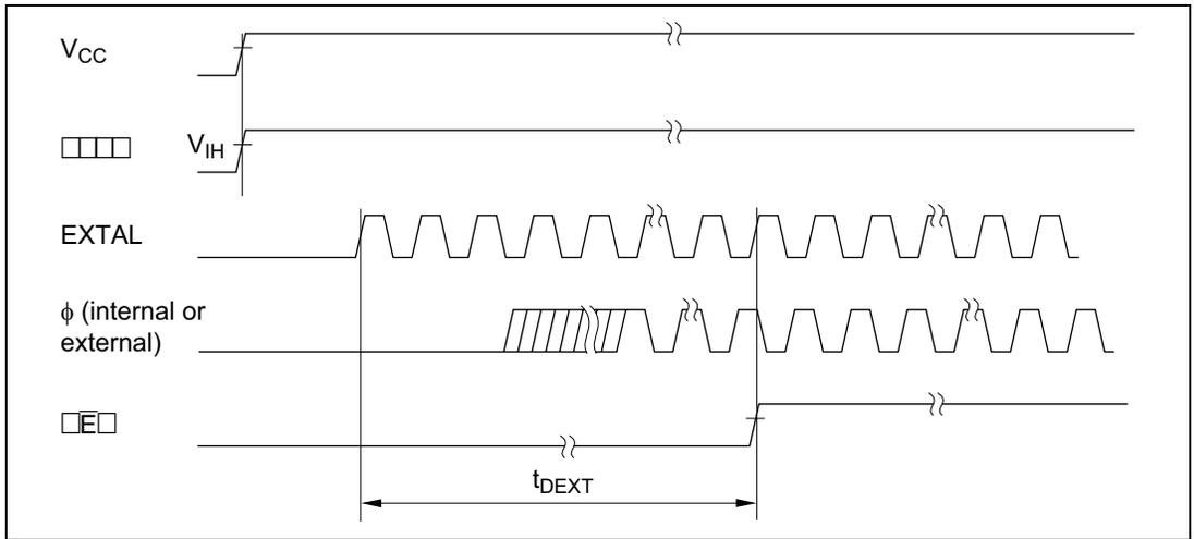
**Figure 19.7 External Clock Output Settling Delay Timing**
