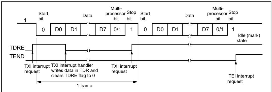
**Figure 13.11 Example of SCI Transmit Operation
