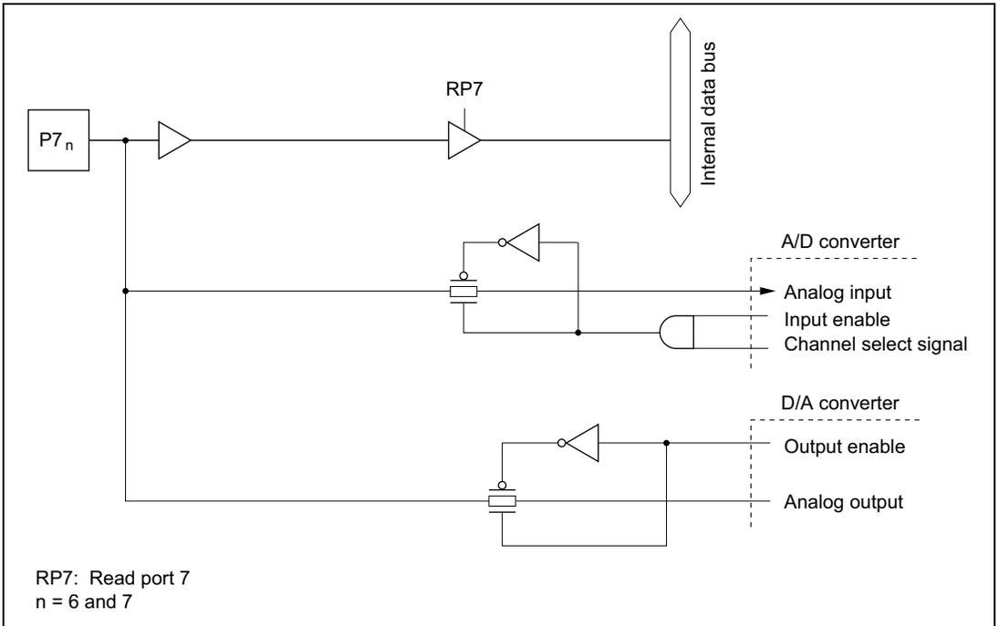
Figure C.7 (b) Port 7 Block Diagram (Pins P7<sub>6</sub> and P7<sub>7</sub>)
