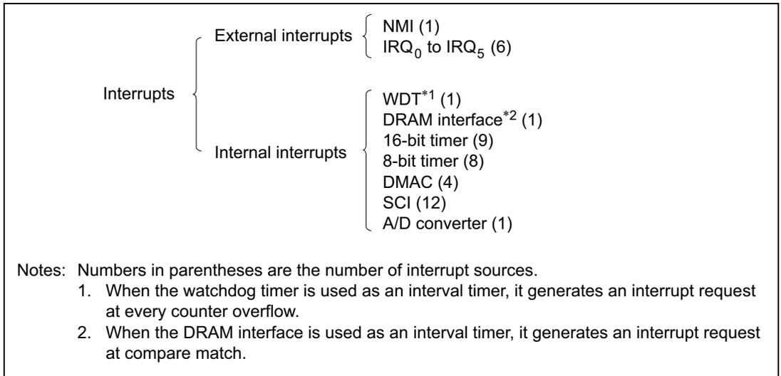
**Figure 4.5 Interrupt Sources and Number of Interrupts**
