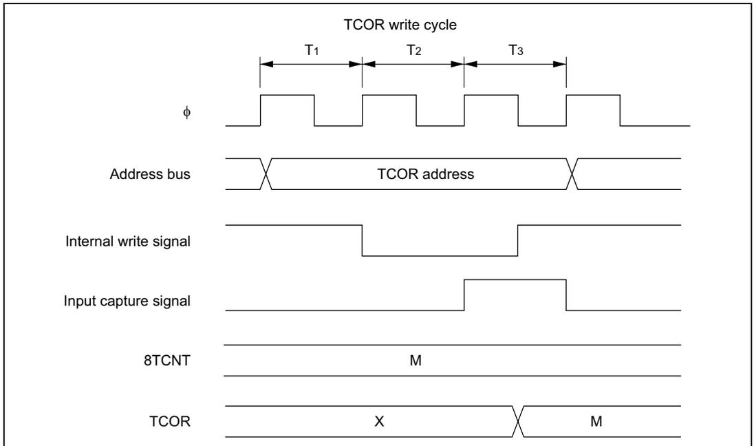
**Figure 10.23** Contention between TCOR Write and Input Capture
