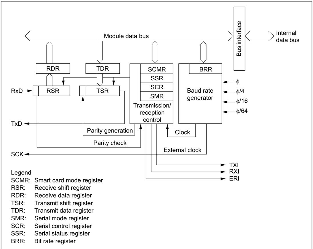
**Figure 14.1 Block Diagram of Smart Card Interface**
