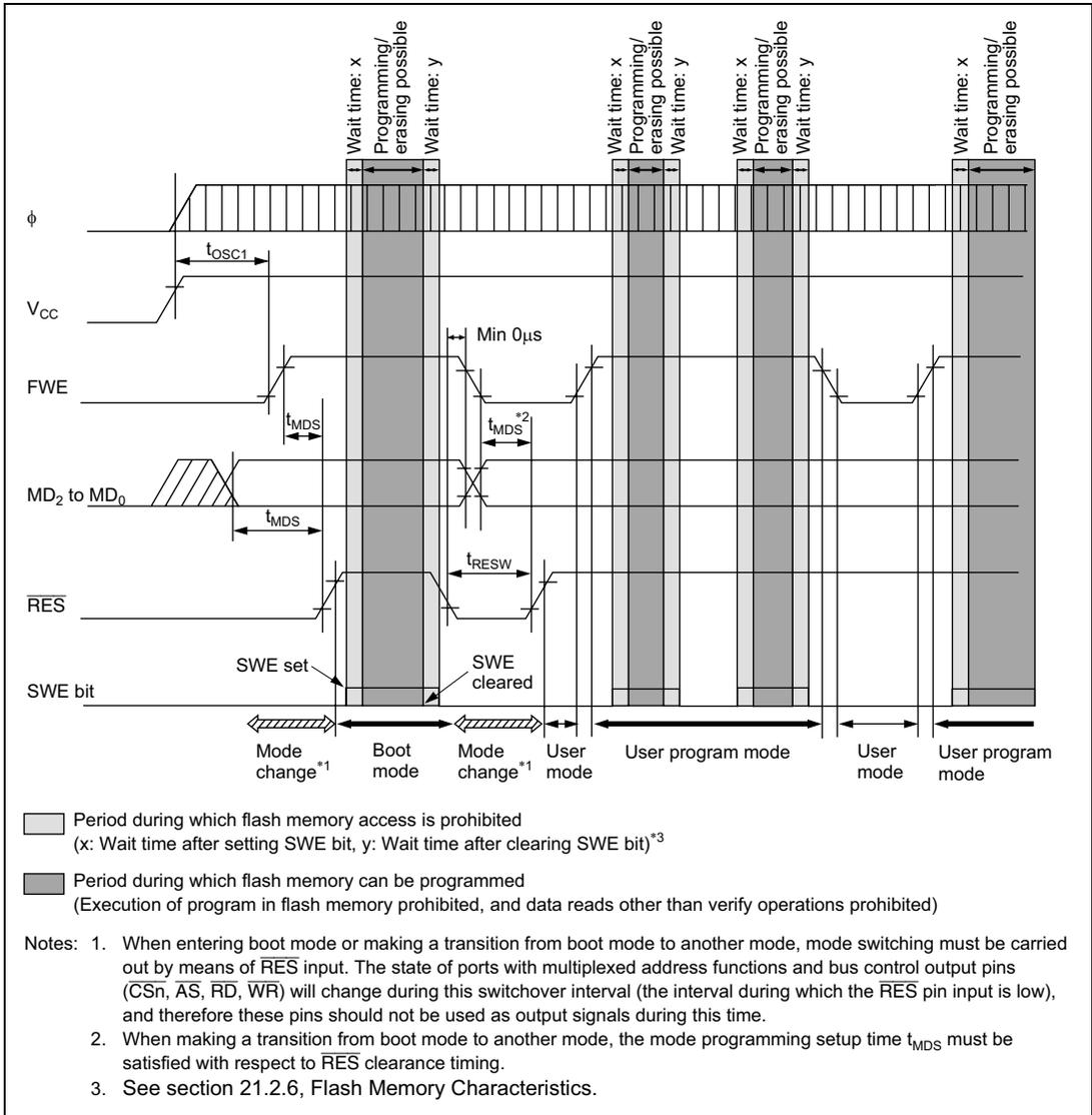
**Figure 18.18 Mode Transition Timing**
