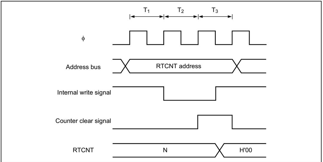
**Figure 6.39 Contention between RTCNT Write and Clear**
