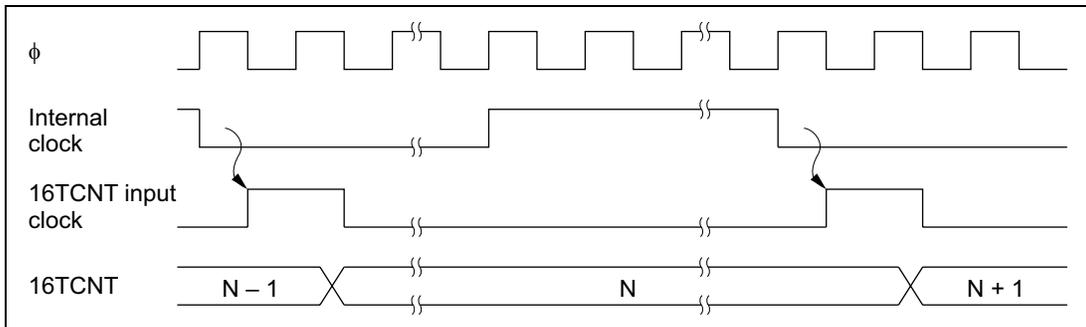
**Figure 9.15 Count Timing for Internal Clock Sources**
