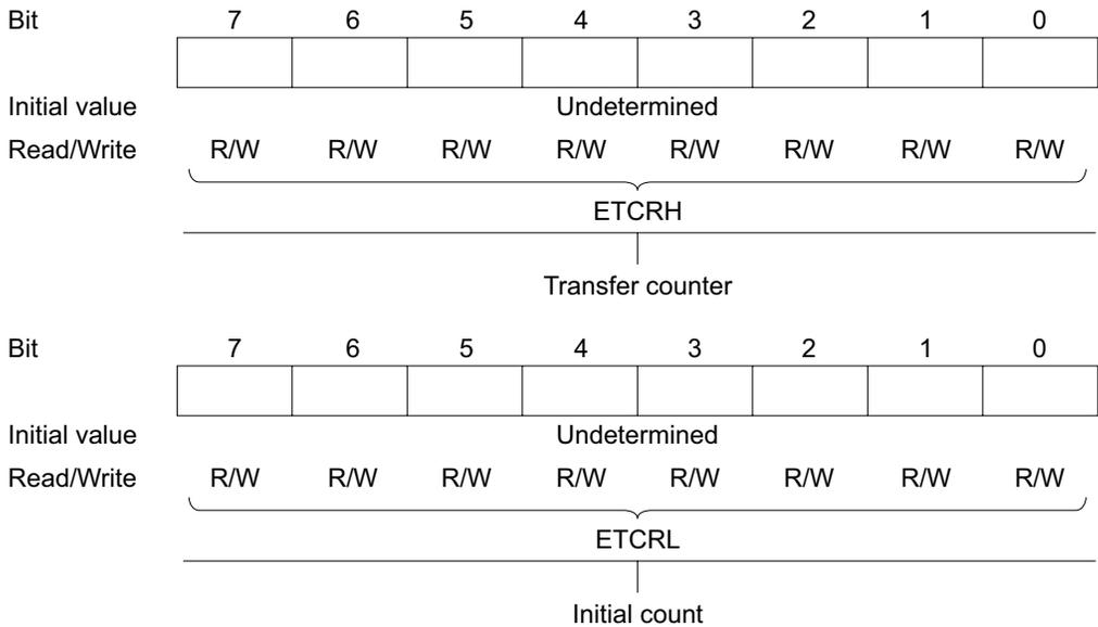
In repeat mode, ETCRH functions as an 8-bit transfer counter and ETCRL holds the initial transfer count. ETCRH is decremented by 1 each time one transfer is executed. When ETCRH reaches H'00, the value in ETCRL is reloaded into ETCRH and the same operation is repeated.
