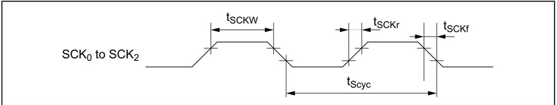
**Figure 21.23 SCI Input Clock Timing**
