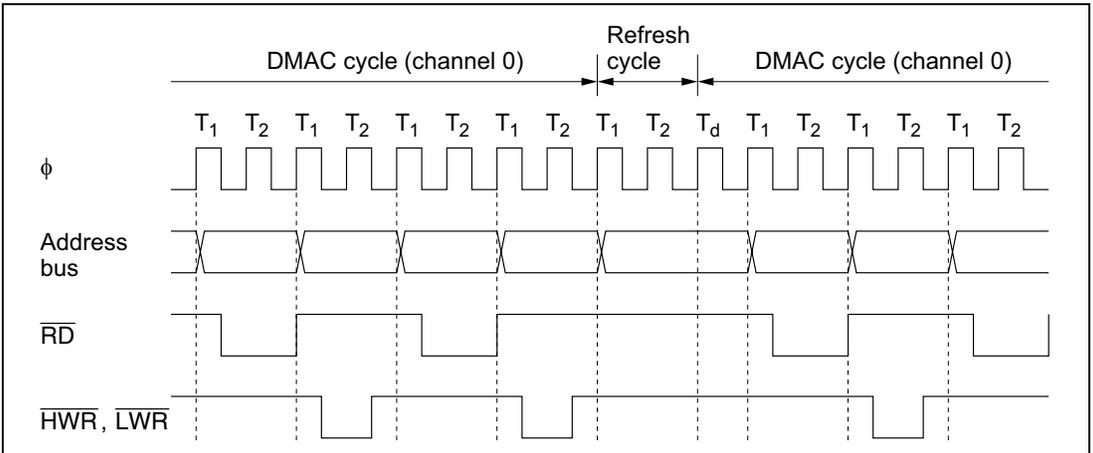
**Figure 7.20 Bus Timing of DRAM Interface, and DMAC**
