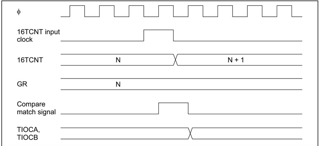
**Figure 9.20 Output Compare Output Timing**
