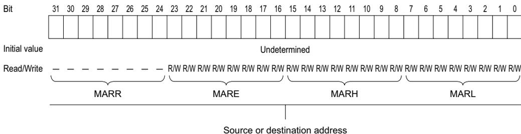
The MAR value is incremented or decremented each time one byte or word is transferred, automatically updating the source or destination memory address. For details, see section 7.3.4, Data Transfer Control Registers (DTCR).
