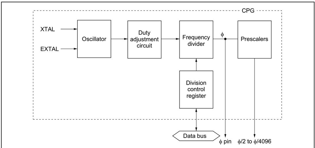
Figure 19.1 Block Diagram of Clock Pulse Generator
