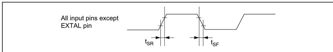
**Figure 21.28 Input Signal Rise and Fall Timing**
