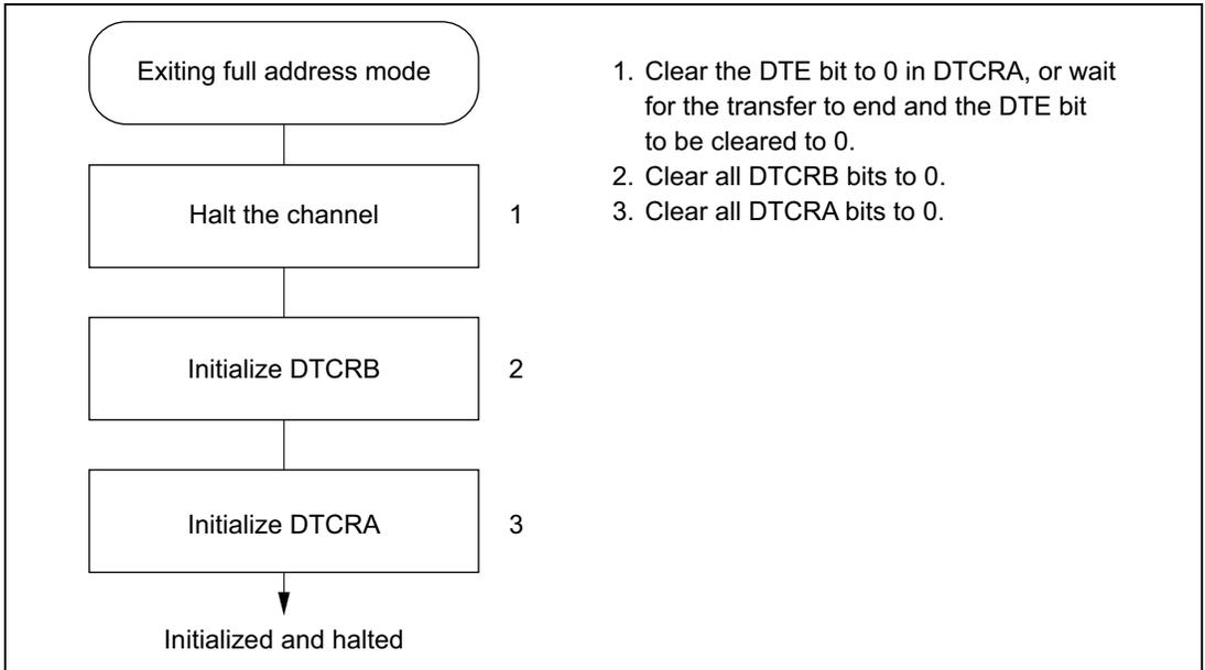
**Figure 7.23 Procedure for Exiting Full Address Mode (Example)**
