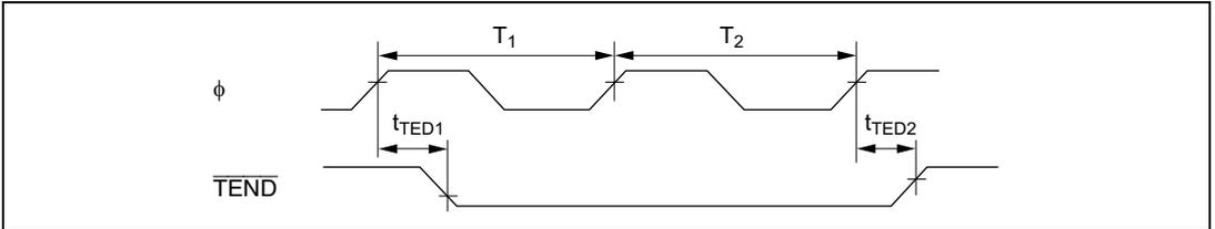
Figure 21.25 DMAC  $\overline{\text{TEND}}$  Output Timing for 2-State Access
