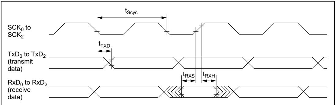
**Figure 21.24 SCI Input/Output Timing in Synchronous Mode**
