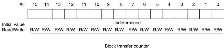
**IOAR0B—I/O Address Register 0B****H'FFF2E****DMAC0**
