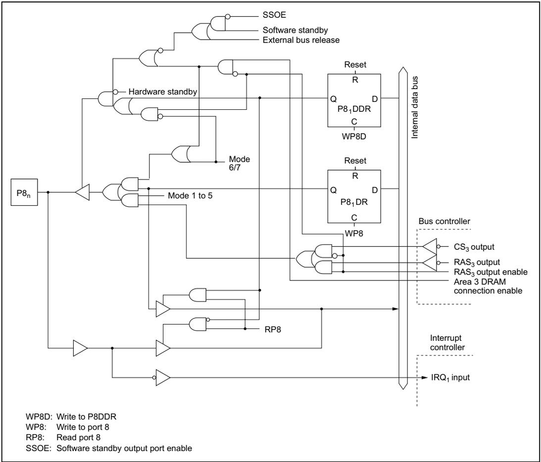
**Figure C.8 (b) Port 8 Block Diagram (Pin P8<sub>1</sub>)**
