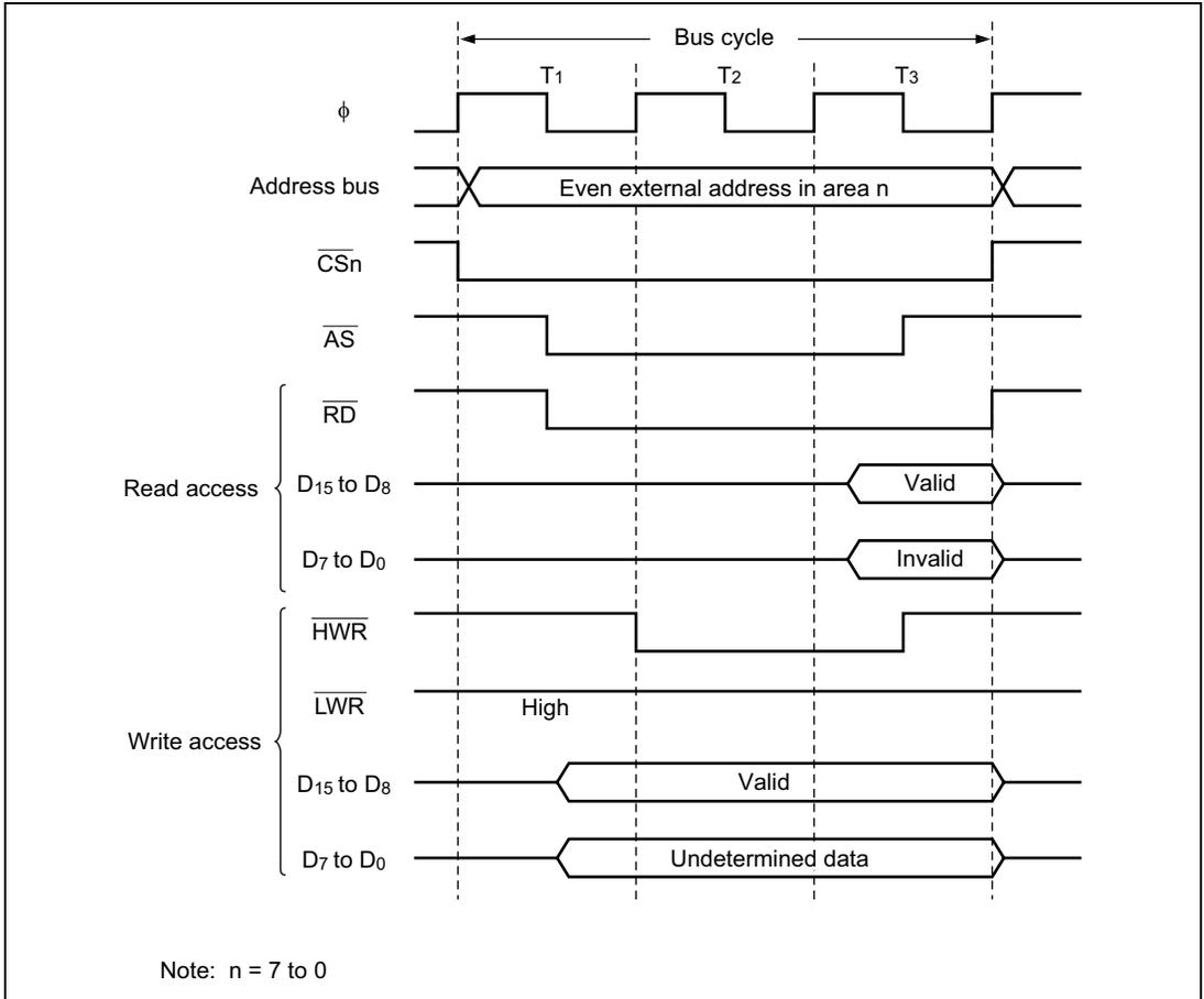
**Figure 6.11 Bus Control Signal Timing for 16-Bit, Three-State-Access Area (1)
