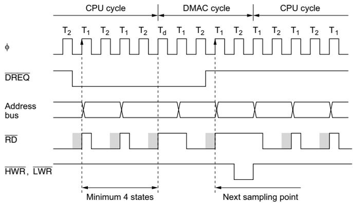
Figure 7.18 Timing of DMAC Activation by Falling Edge of  $\overline{\text{DREQ}}$  in Block Transfer Mode 234 Figure amended
