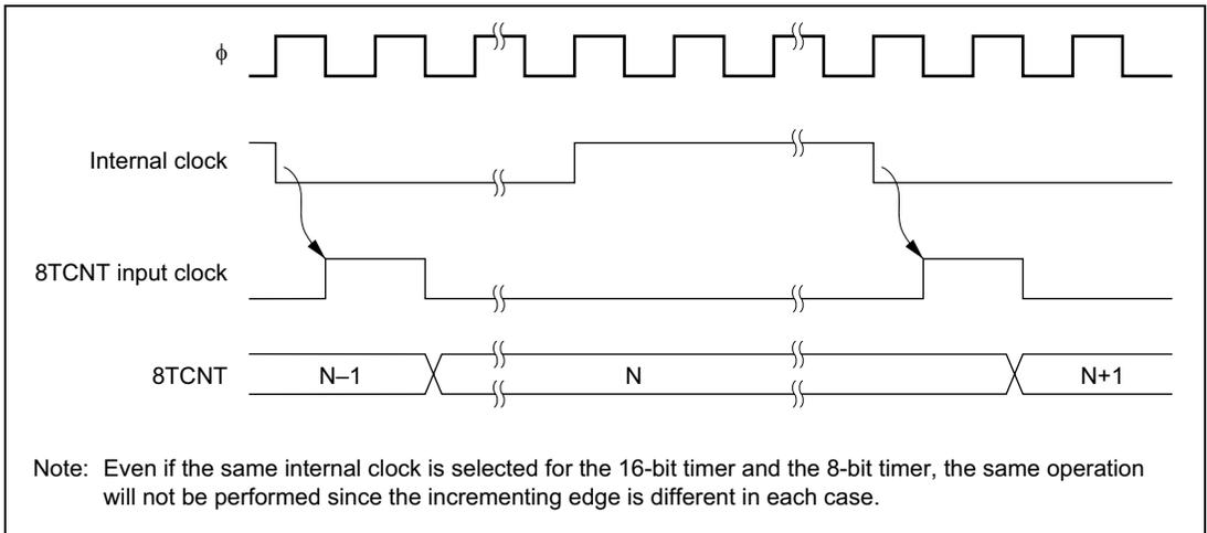
**Figure 10.8 Count Timing for Internal Clock Input**
