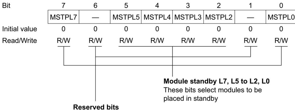
MSTCRL is initialized to H'00 by a reset and in hardware standby mode. It is not initialized in software standby mode.
