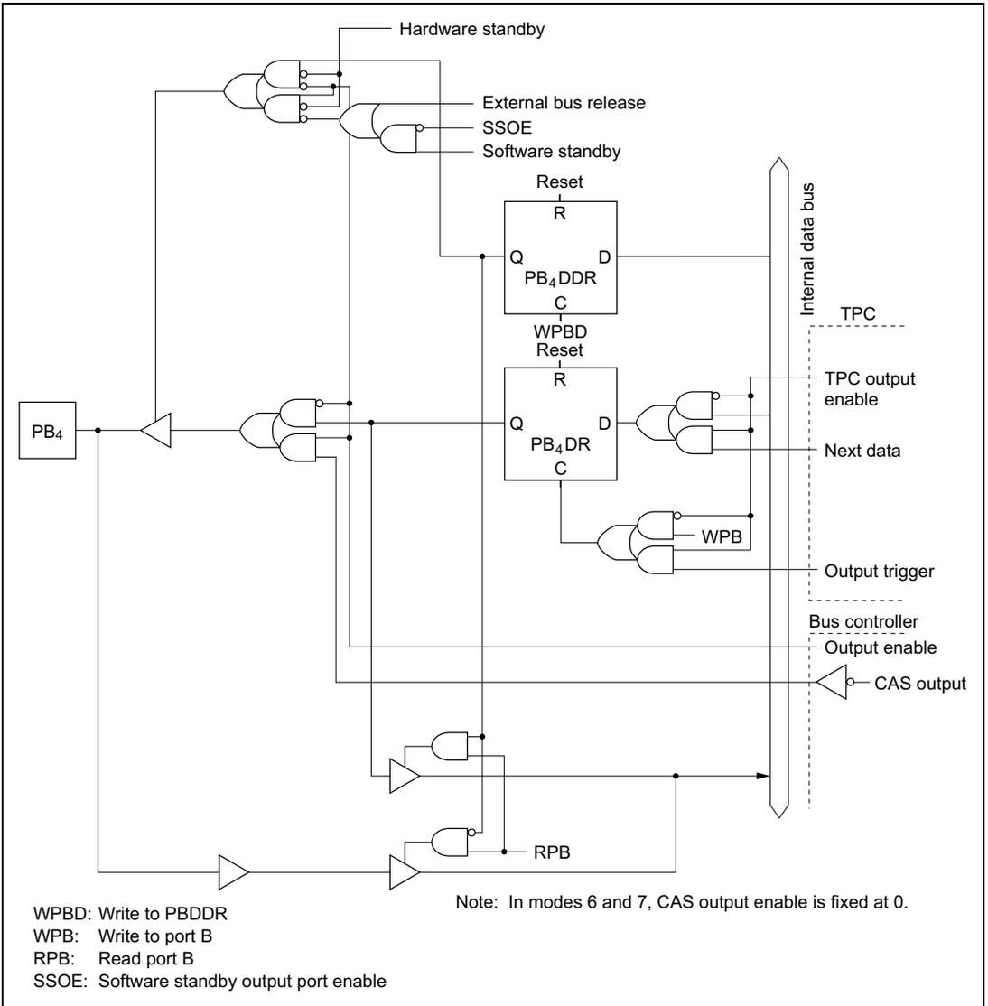
Figure C.11 (e) Port B Block Diagram (Pin PB<sub>4</sub>)
