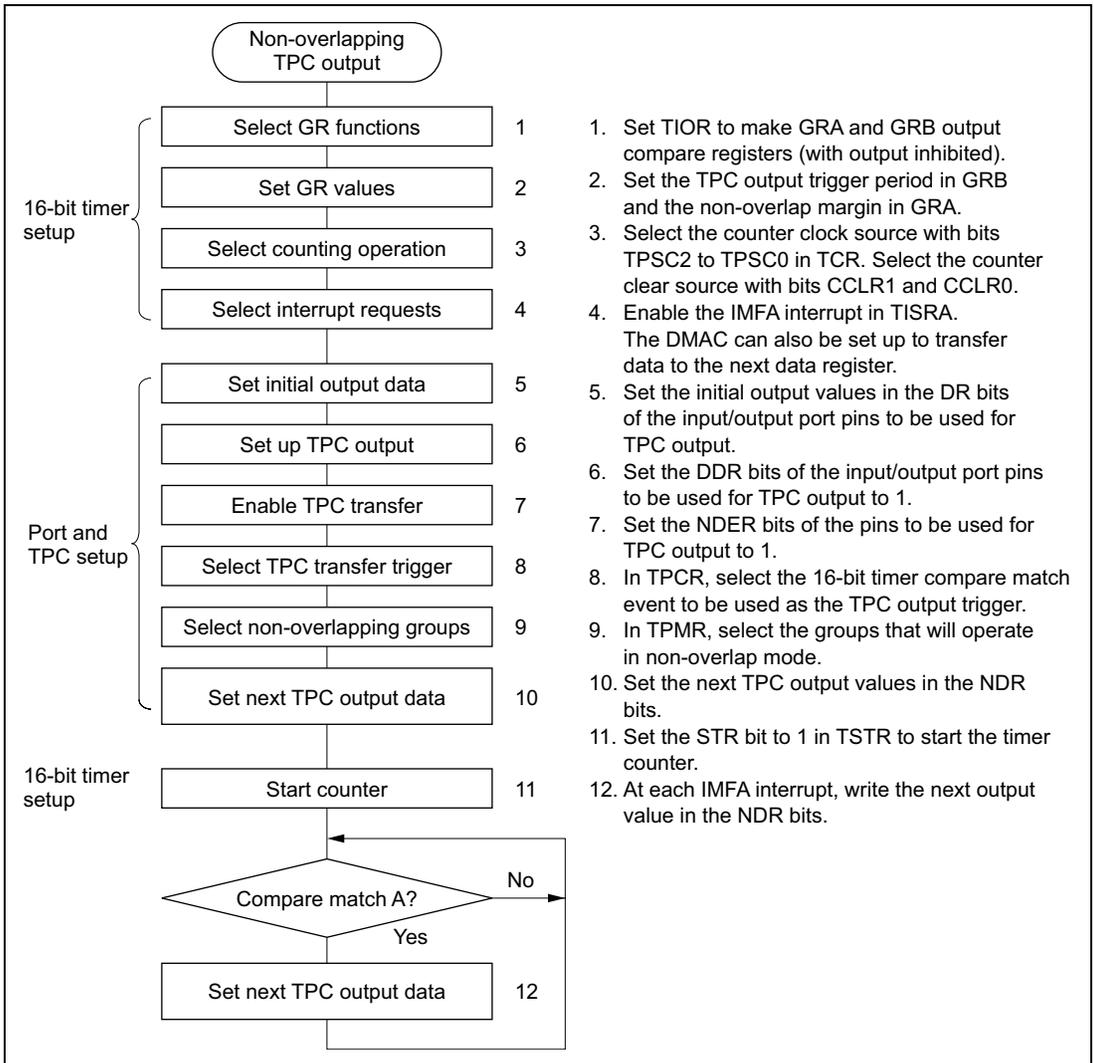
**Figure 11.6 Setup Procedure for Non-Overlapping TPC Output (Example)**
