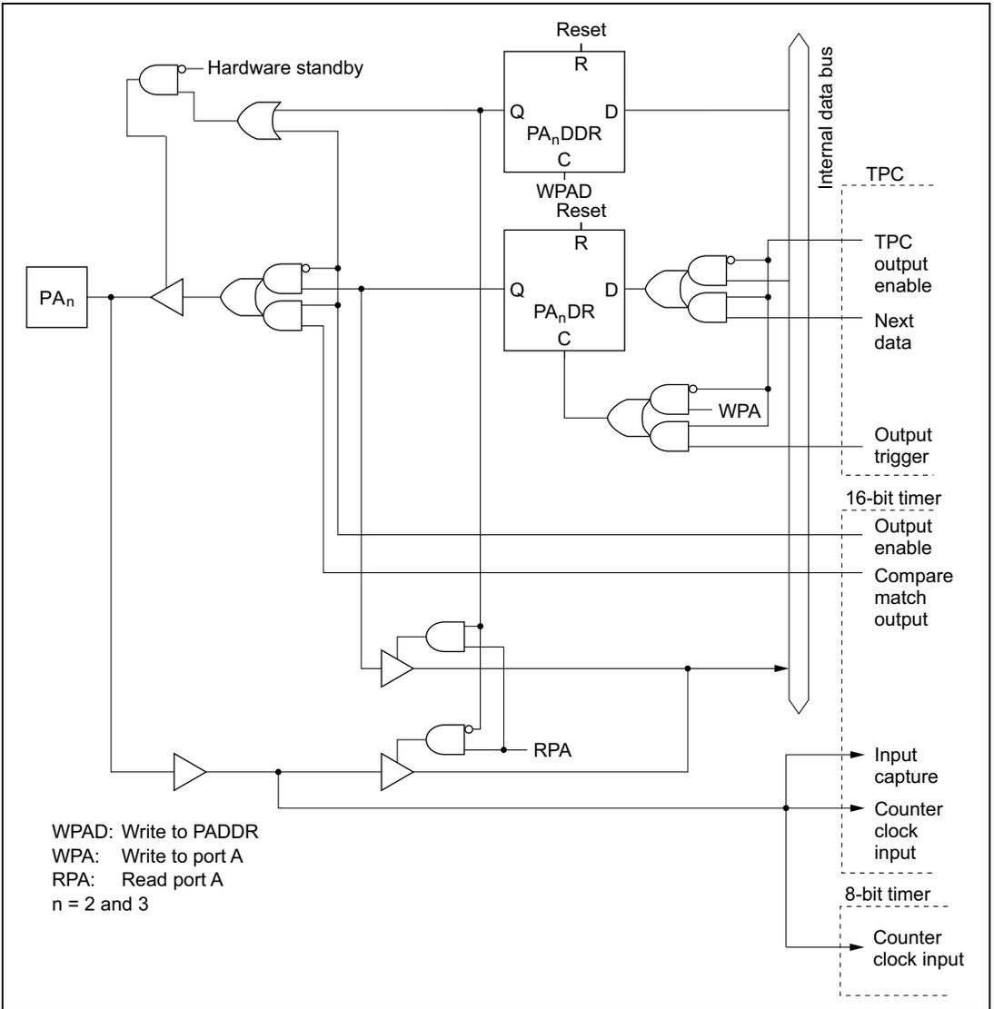
Figure C.10 (b) Port A Block Diagram (Pins PA<sub>2</sub>, PA<sub>3</sub>)
