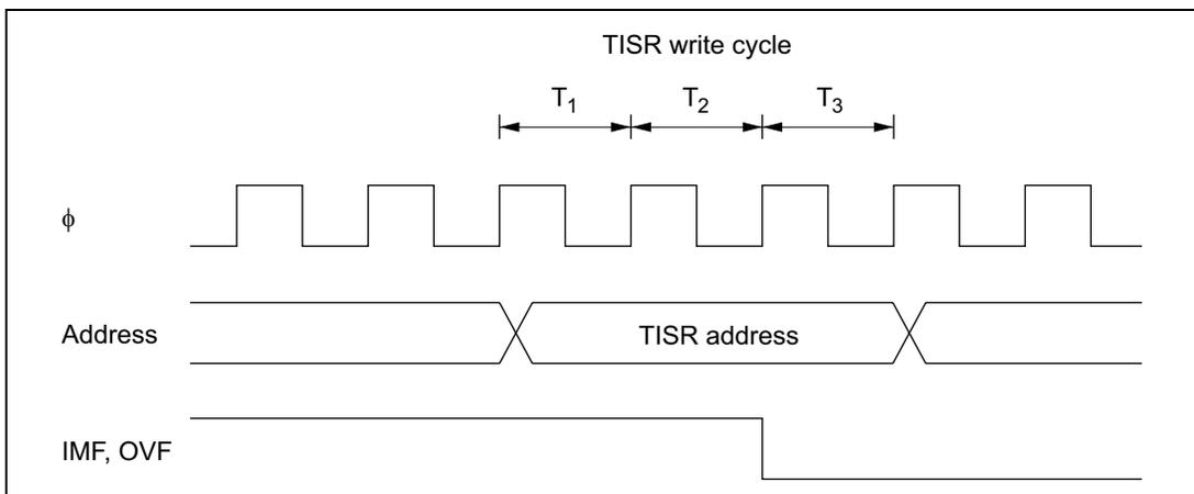
**Figure 9.36 Timing of Clearing of Status Flags**
