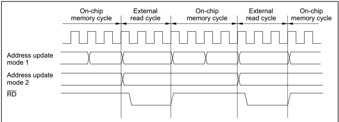
**Figure 6.5 Sample Address Output in Each Address Update Mode
