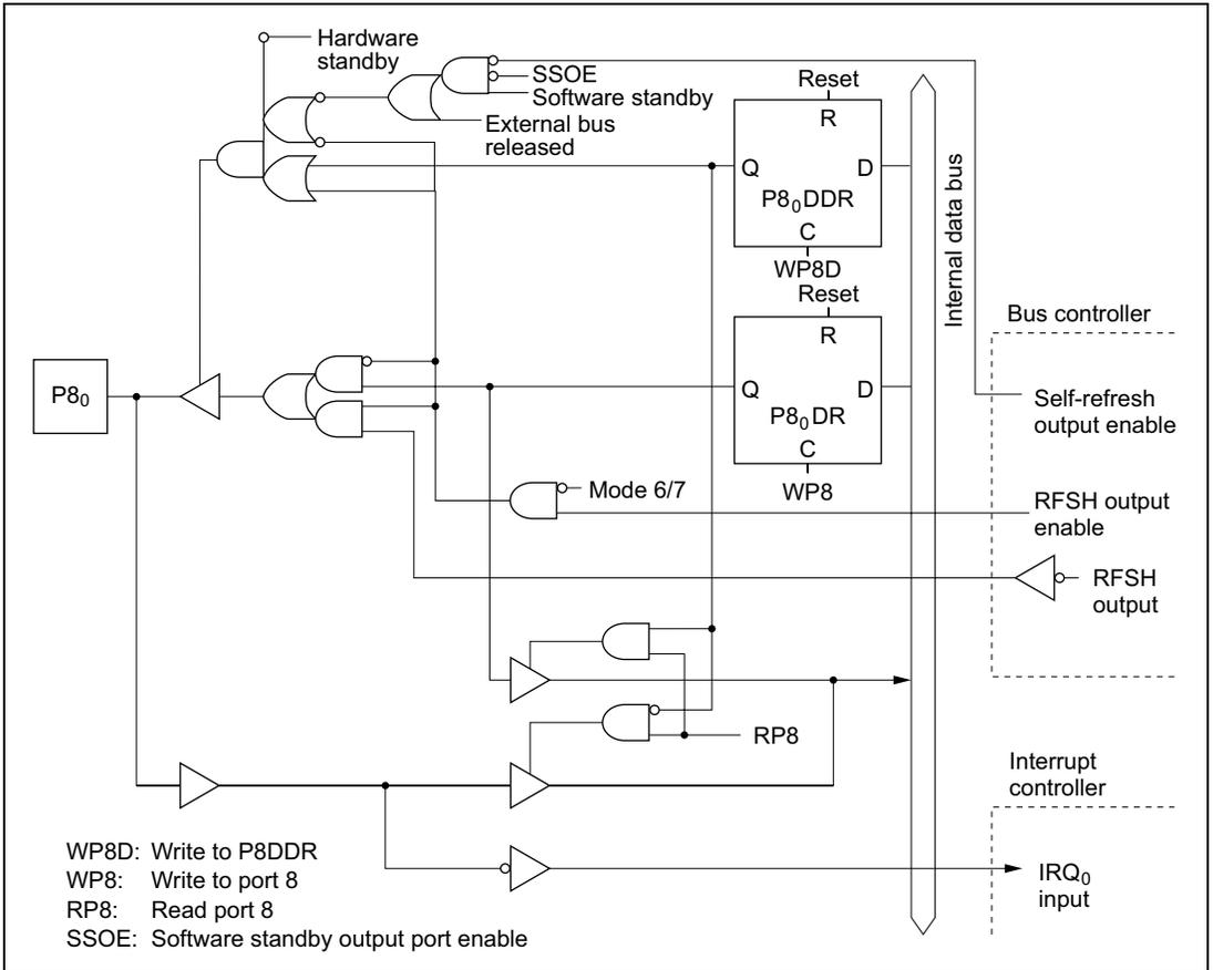
Figure C.8 (a) Port 8 Block Diagram (Pin P80)
