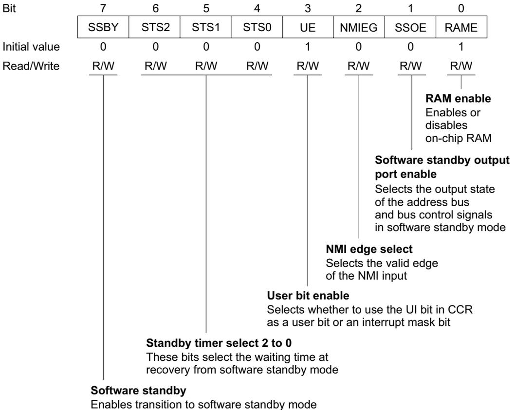
**Bit 7—Software Standby (SSBY):** Enables transition to software standby mode. (For further information about software standby mode see section 20, Power-Down State.)
