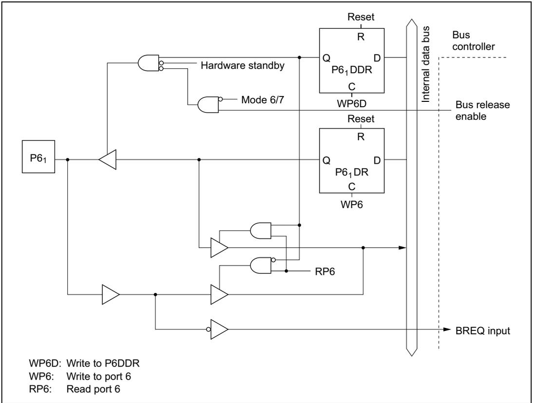
Figure C.6 (b) Port 6 Block Diagram (Pin P6<sub>1</sub>)
