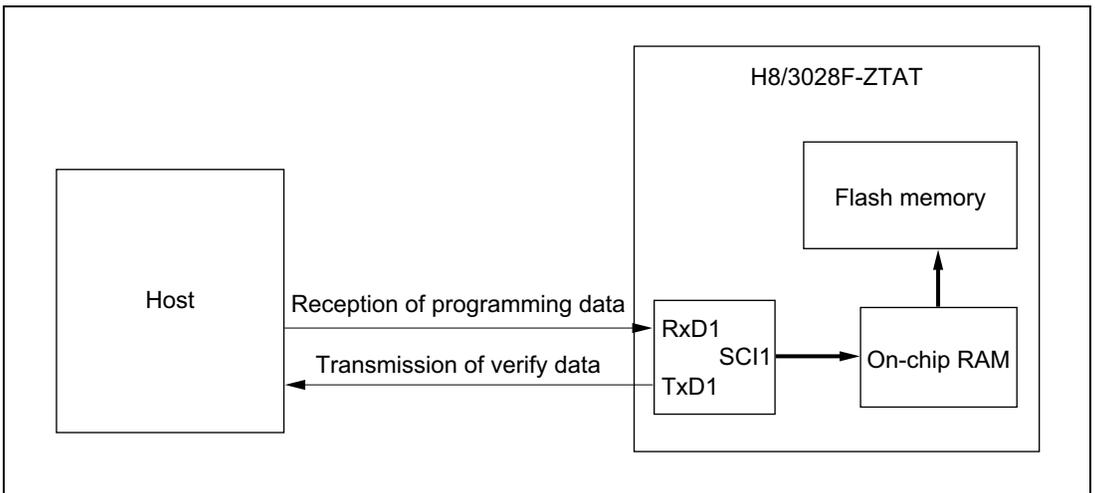
**Figure 18.5 System Configuration When Using Boot Mode**
