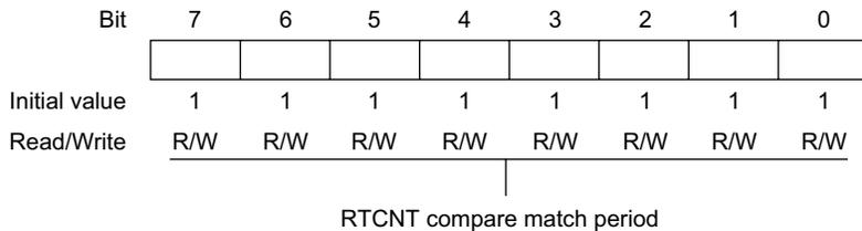
Note: Only byte access can be used on this register.
