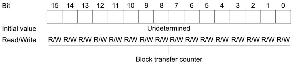
In block transfer mode, ETCRAH functions as an 8-bit block size counter. ETCRAL holds the initial block size. ETCRAH is decremented by 1 each time one byte or word is transferred. When the count reaches H'00, ETCRAH is reloaded from ETCRAL. Blocks consisting of an arbitrary number of bytes or words can be transferred repeatedly by setting the same initial block size value in ETCRAH and ETCRAL.
