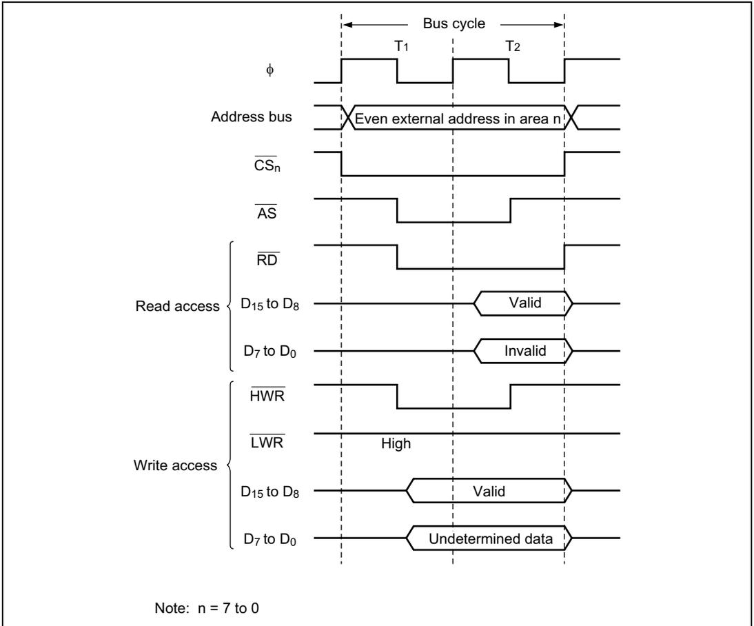
**Figure 6.14 Bus Control Signal Timing for 16-Bit, Two-State-Access Area (1)
