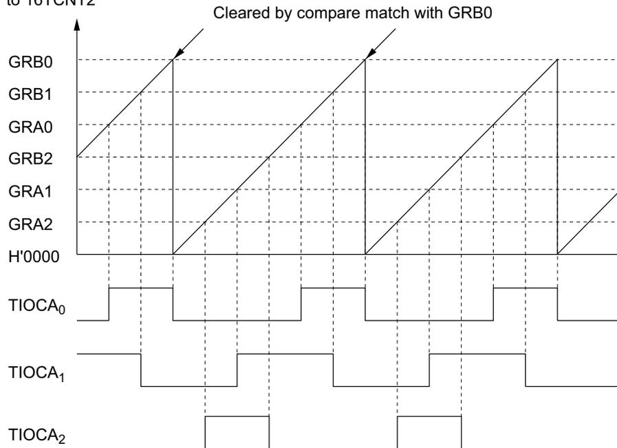
**Figure 9.25 Synchronization (Example)**
