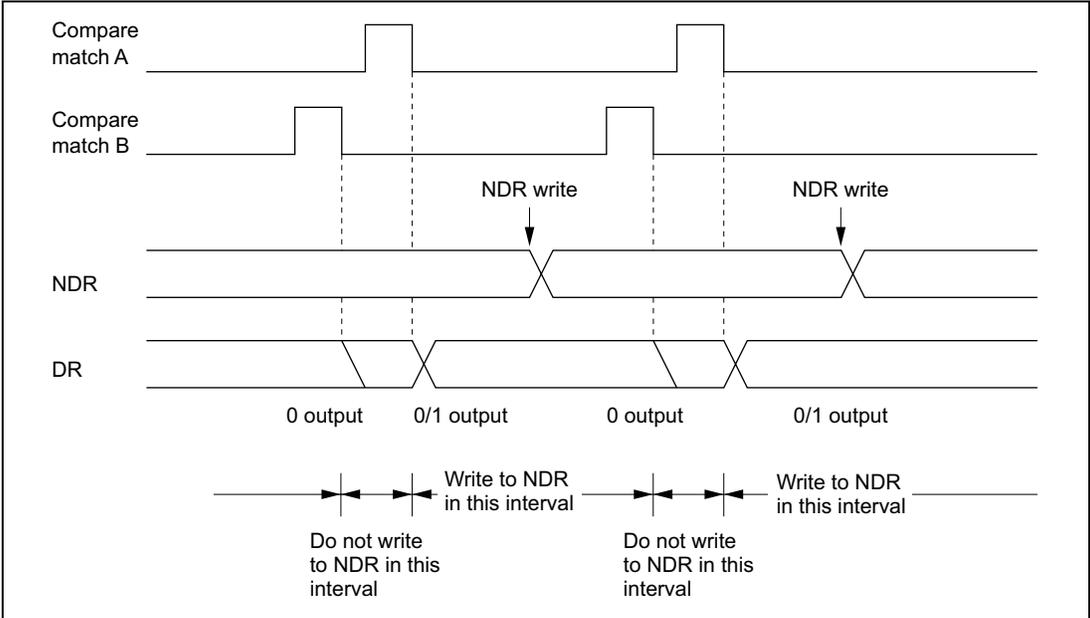
**Figure 11.10 Non-Overlapping Operation and NDR Write Timing**
