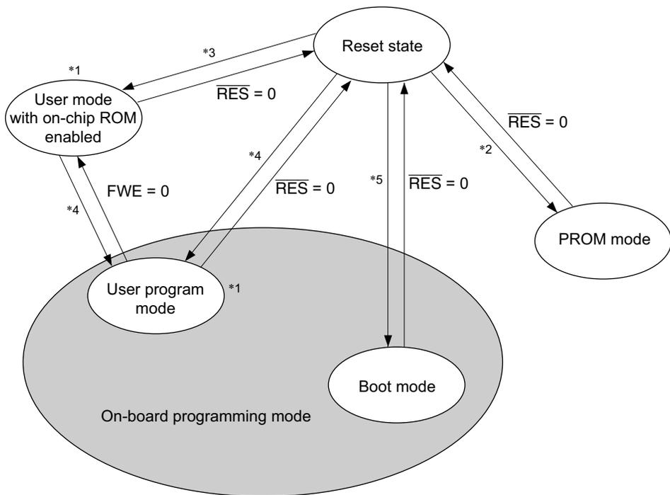
Notes: Only make a transition between user mode and user program mode when the CPU is not accessing the flash memory.
