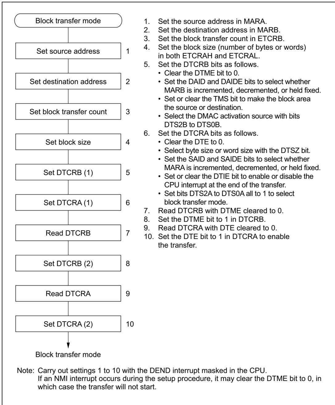
**Figure 7.12 Block Transfer Mode Setup Procedure (Example)**
