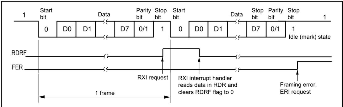
**Figure 13.8 Example of SCI Receive Operation
