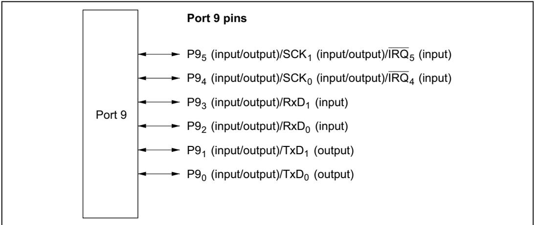
**Figure 8.9 Port 9 Pin Configuration**
