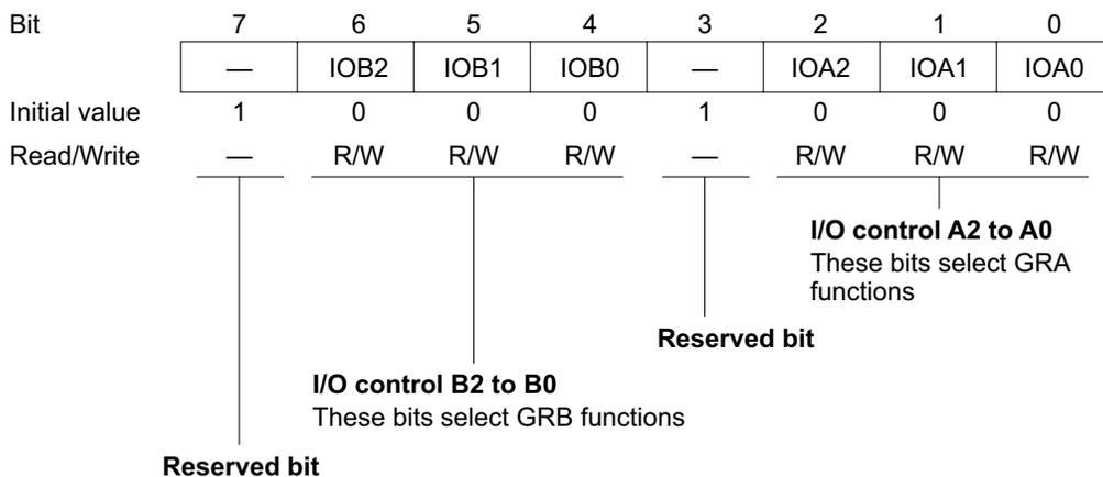
Each TIOR is an 8-bit readable/writable register that selects the output compare or input capture function for GRA and GRB, and specifies the functions of the TIORA and TIORB pins. If the output compare function is selected, TIOR also selects the type of output. If input capture is selected, TIOR also selects the edges of the input capture signal.
