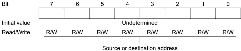
An IOAR functions as a source or destination address register depending on how the DMAC is activated: as a destination address register if activation is by a receive-data-full interrupt from serial communication interface (SCI) channel 0 or by an A/D converter conversion-end interrupt, and as a source address register otherwise.
