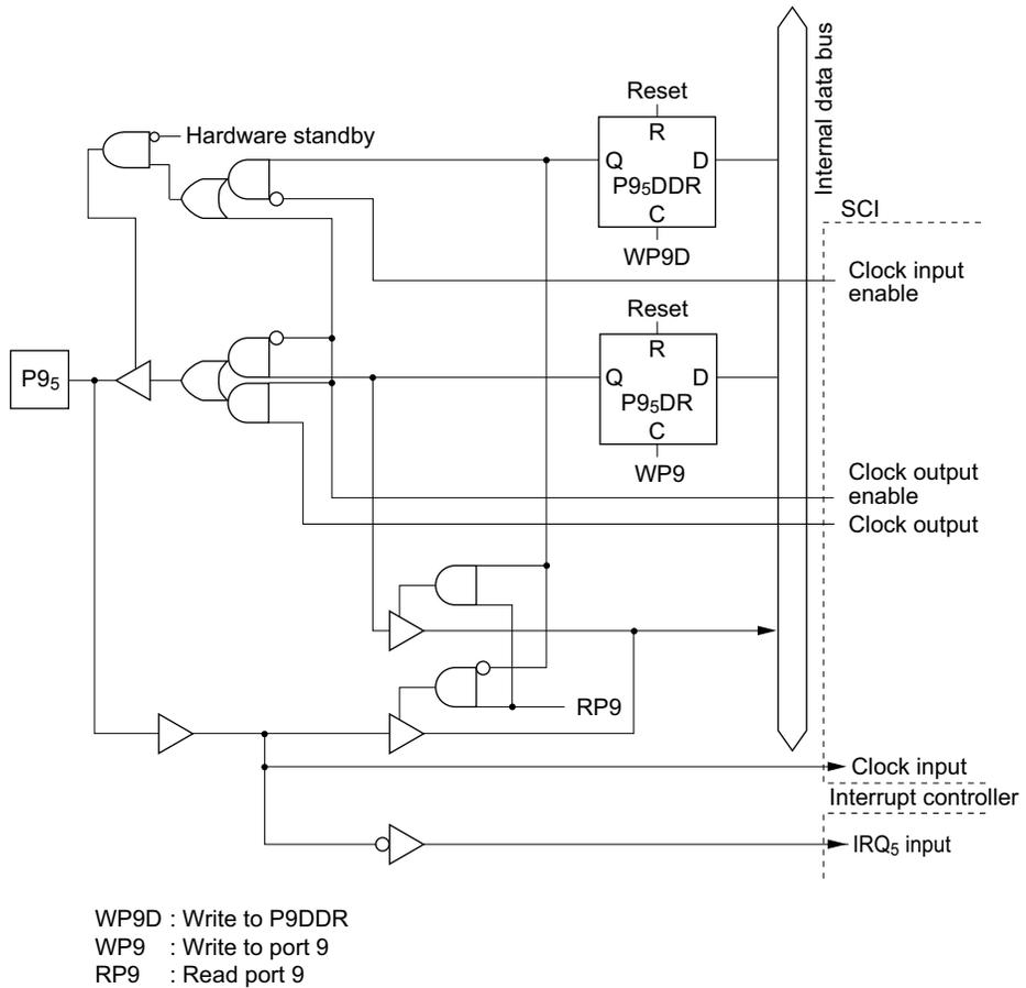
Figure C.9 (f) Port 9 Block Diagram (Pin P9<sub>5</sub>)
