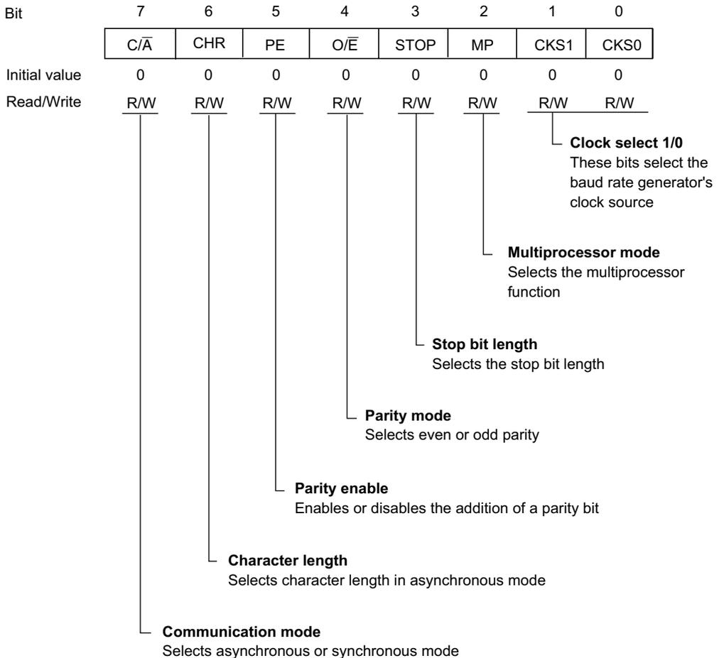
The CPU can always read and write SMR. SMR is initialized to H'00 by a reset and in standby mode.
