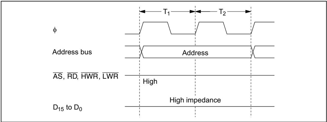
**Figure 2.16 Pin States during On-Chip Memory Access**
