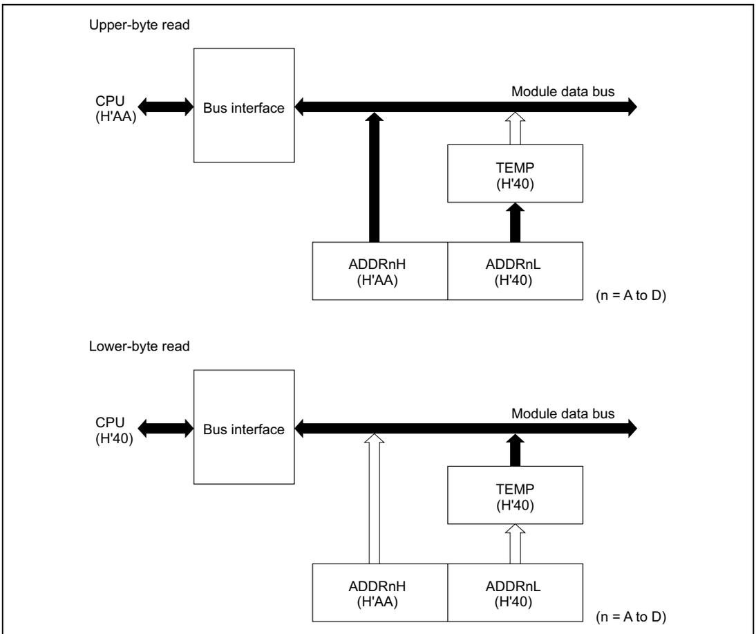
Figure 15.2 A/D Data Register Access Operation (Reading H'AA40)
