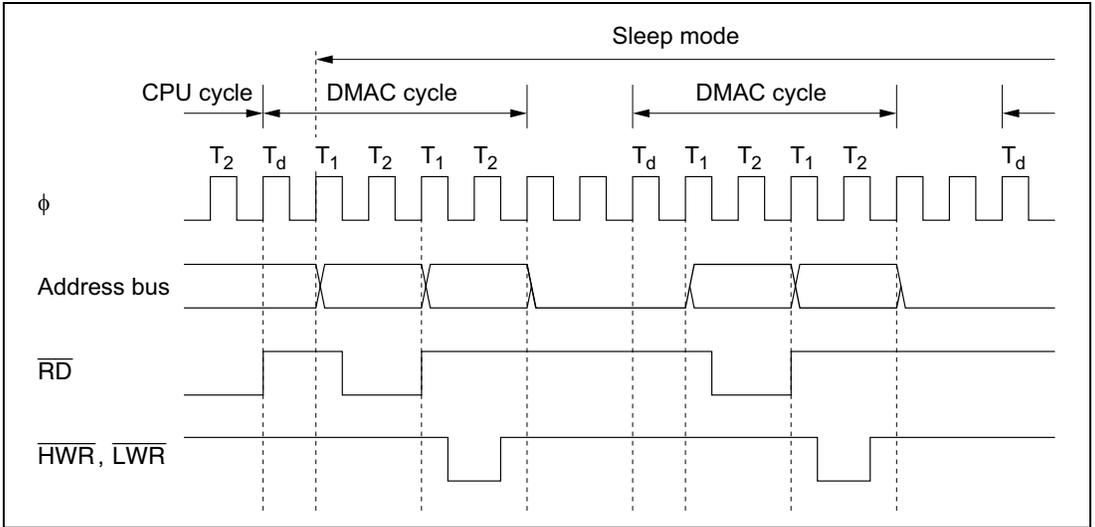
Figure 7.24 Timing of Cycle-Steal Transfer in Sleep Mode
