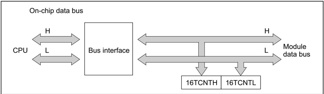
**Figure 9.4 16TCNT Access Operation [CPU → 16TCNT (Word)]**
