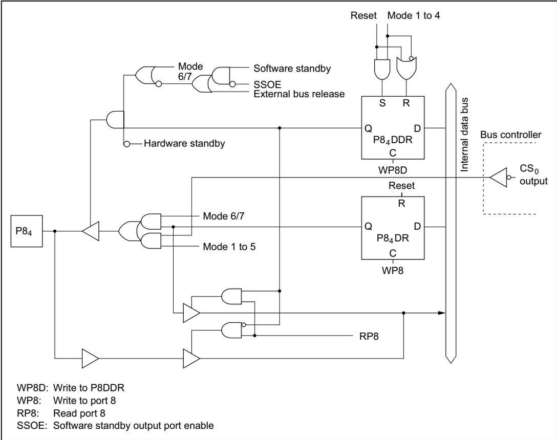
**Figure C.8 (e) Port 8 Block Diagram (Pin P84)**
