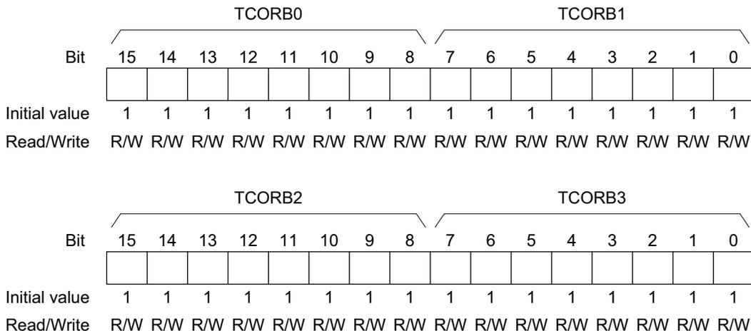
TCORB0 to TCORB3 are 8-bit readable/writable registers. The TCORB0 and TCORB1 pair, and the TCORB2 and TCORB3 pair, can each be accessed as a 16-bit register by word access.
