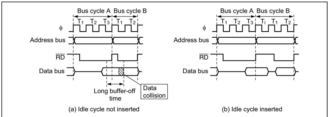
**Figure 6.43 Example of Idle Cycle Operation (1) (ICIS1 = 1)**
