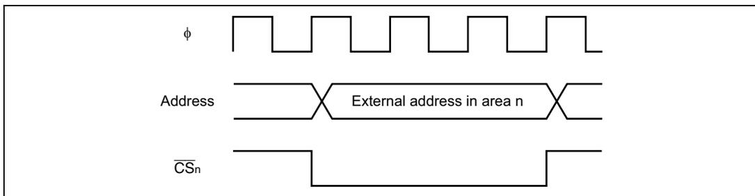
**Figure 6.4  $\overline{CS}_n$  Signal Output Timing (n = 0 to 7)**
