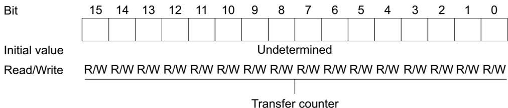
In I/O mode and idle mode, ETCR functions as a 16-bit counter. The count is decremented by 1 each time one transfer is executed. The transfer ends when the count reaches H'0000.
