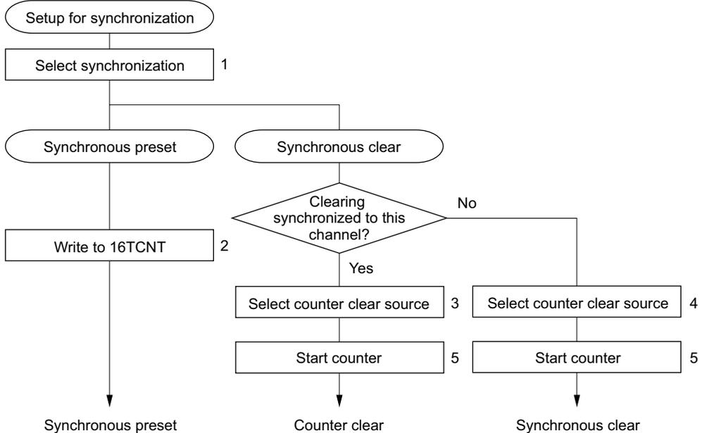
1. Set the SYNC bits to 1 in TSNC for the channels to be synchronized.
