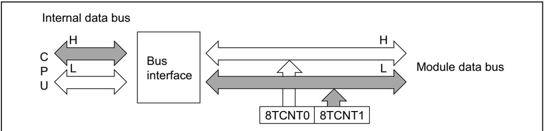
**Figure 10.7 8TCNT1 Access Operation (CPU Reads 8TCNT1, Lower Byte)**
