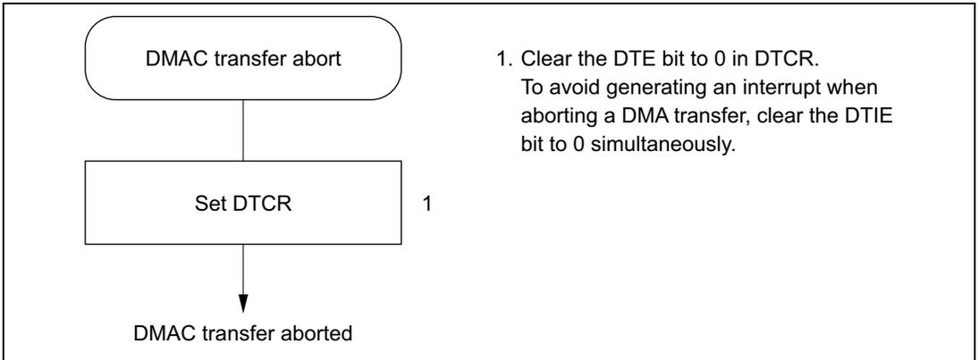
**Figure 7.22 Procedure for Aborting a DMAC Transfer**
