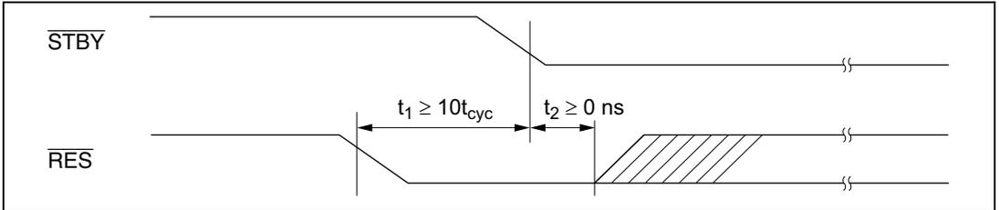
2. To retain RAM contents with the RAME bit cleared to 0 in SYSCR,  $\overline{\text{RES}}$  does not have to be driven low as in (1).
