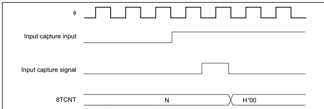
**Figure 10.12 Timing of Clear by Input Capture**
