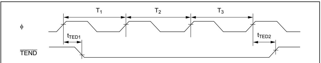
Figure 21.26 DMAC  $\overline{\text{TEND}}$  Output Timing for 3-State Access
