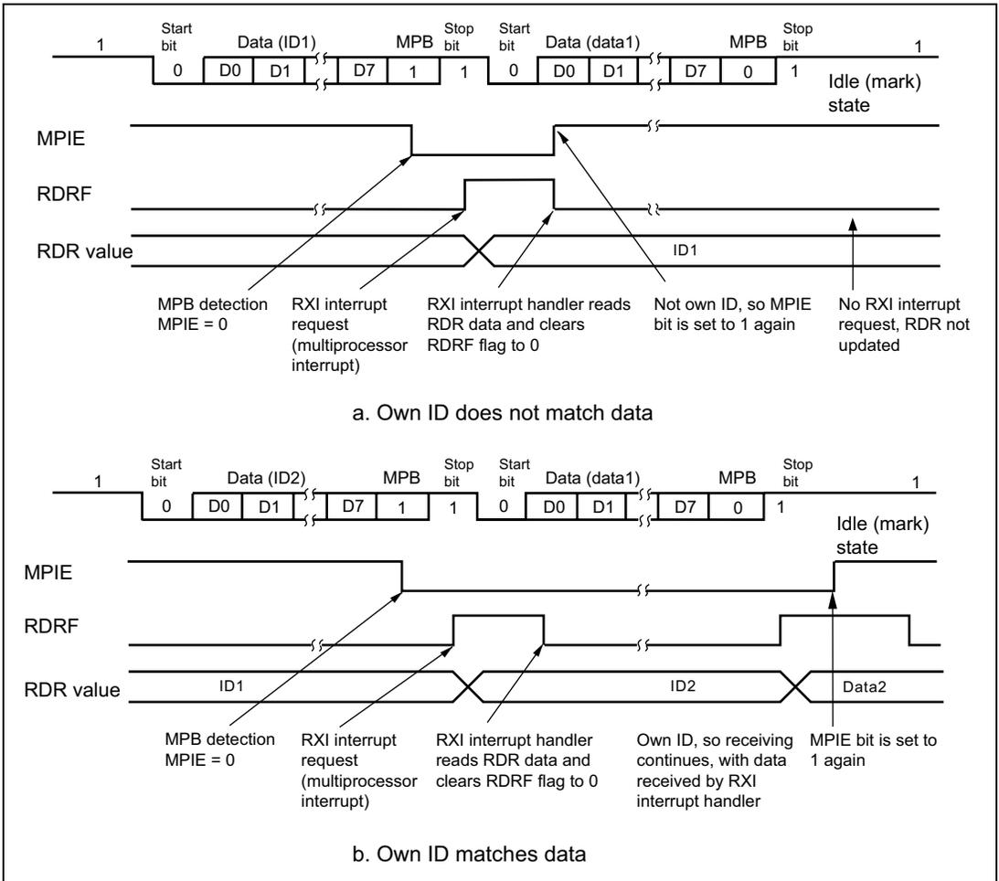
**Figure 13.13 Example of SCI Receive Operation
