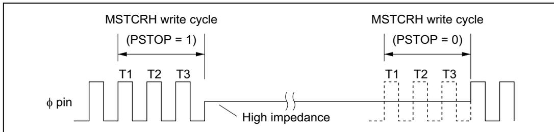
**Figure 20.3 Starting and Stopping of System Clock Output**
