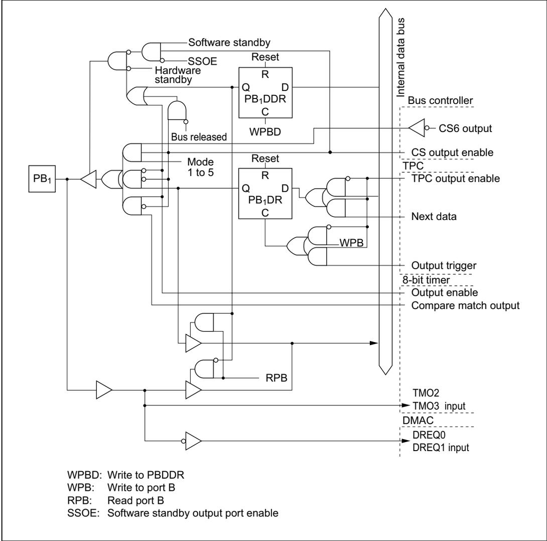
Figure C.11 (b) Port B Block Diagram (Pin PB<sub>1</sub>)
