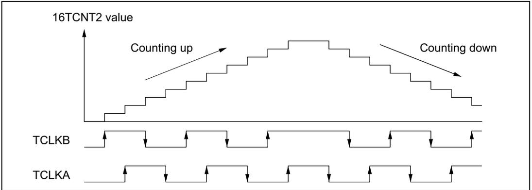
**Figure 9.30 Operation in Phase Counting Mode (Example)**
