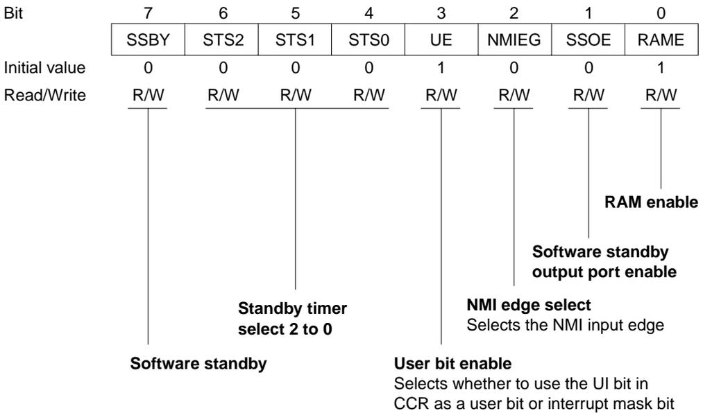
**Bit 3—User Bit Enable (UE):** Selects whether to use the UI bit in CCR as a user bit or an interrupt mask bit.
