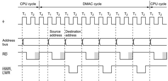
Figure 7.16 Timing of DMAC Activation by Falling Edge of DREQ in Normal Mode
