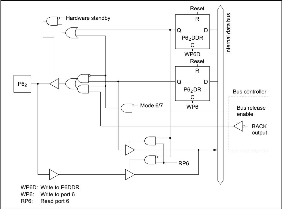
**Figure C.6 (c) Port 6 Block Diagram (Pin P6<sub>2</sub>)**
