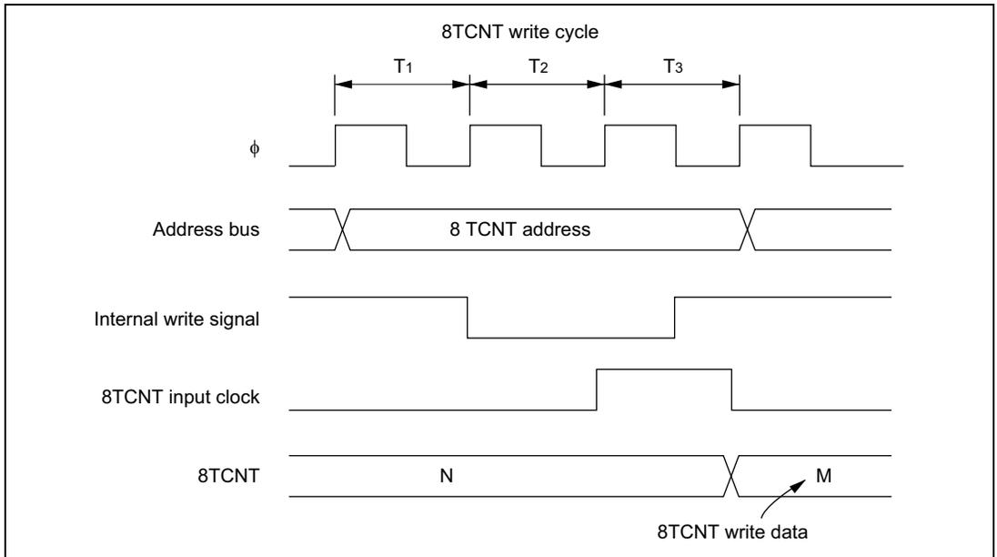
**Figure 10.19 Contention between 8TCNT Write and Increment**
