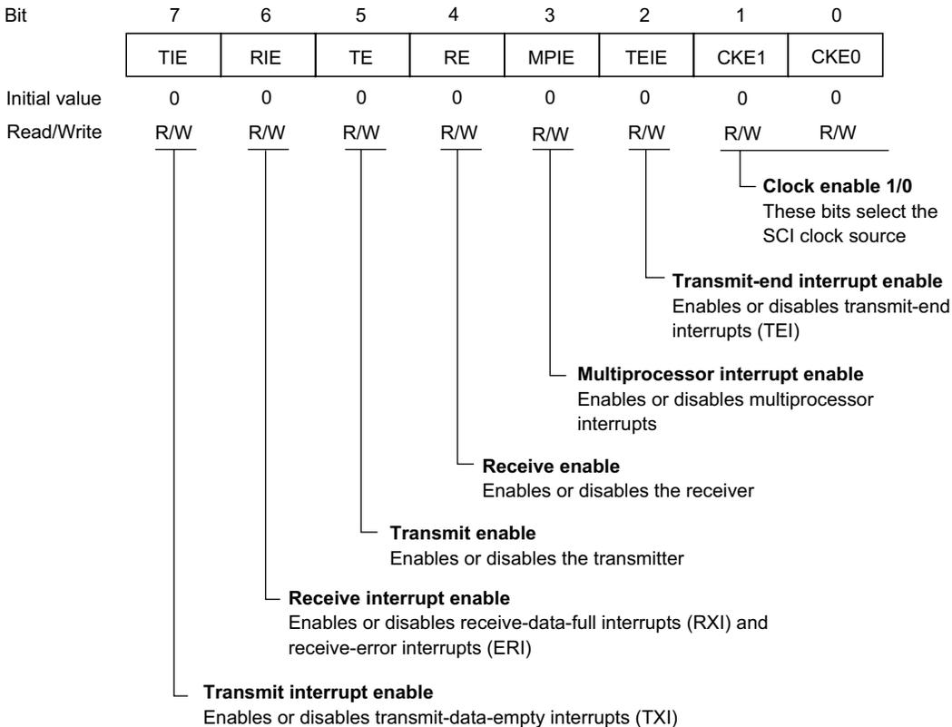
The CPU can always read and write SCR. SCR is initialized to H'00 by a reset and in standby mode.
