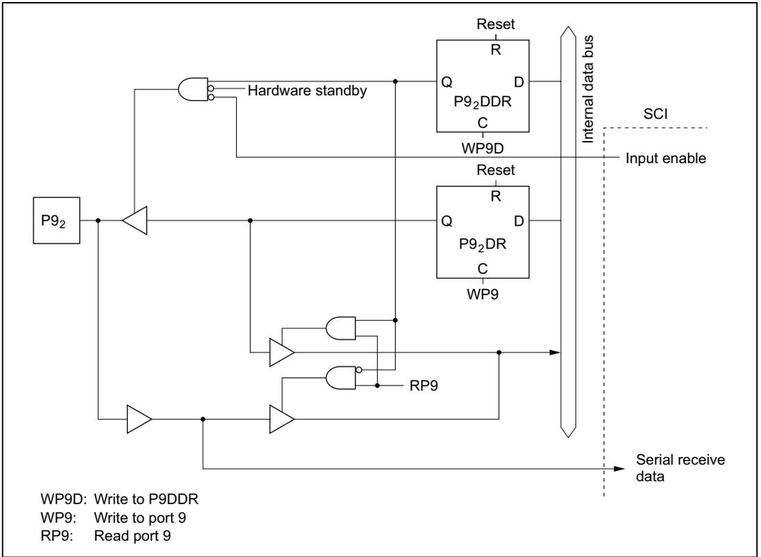
**Figure C.9 (c) Port 9 Block Diagram (Pin P9<sub>2</sub>)**
