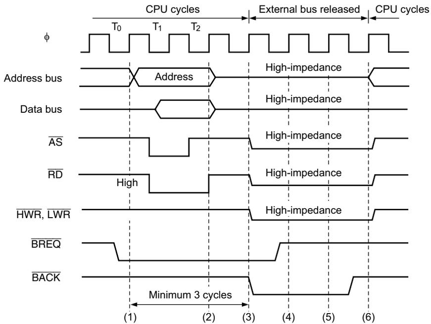
**Figure 6.48 Example of External Bus Master Operation**
