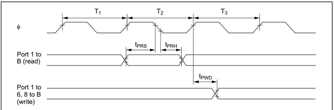
**Figure 21.20 TPC and I/O Port Input/Output Timing**
