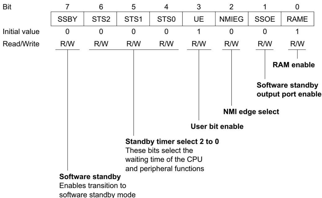
SYSCR is an 8-bit readable/writable register. Bit 7 (SSBY), bits 6 to 4 (STS2 to STS0), and bit 1 (SSOE) control the power-down state. For information on the other SYSCR bits, see section 3.3, System Control Register (SYSCR).
