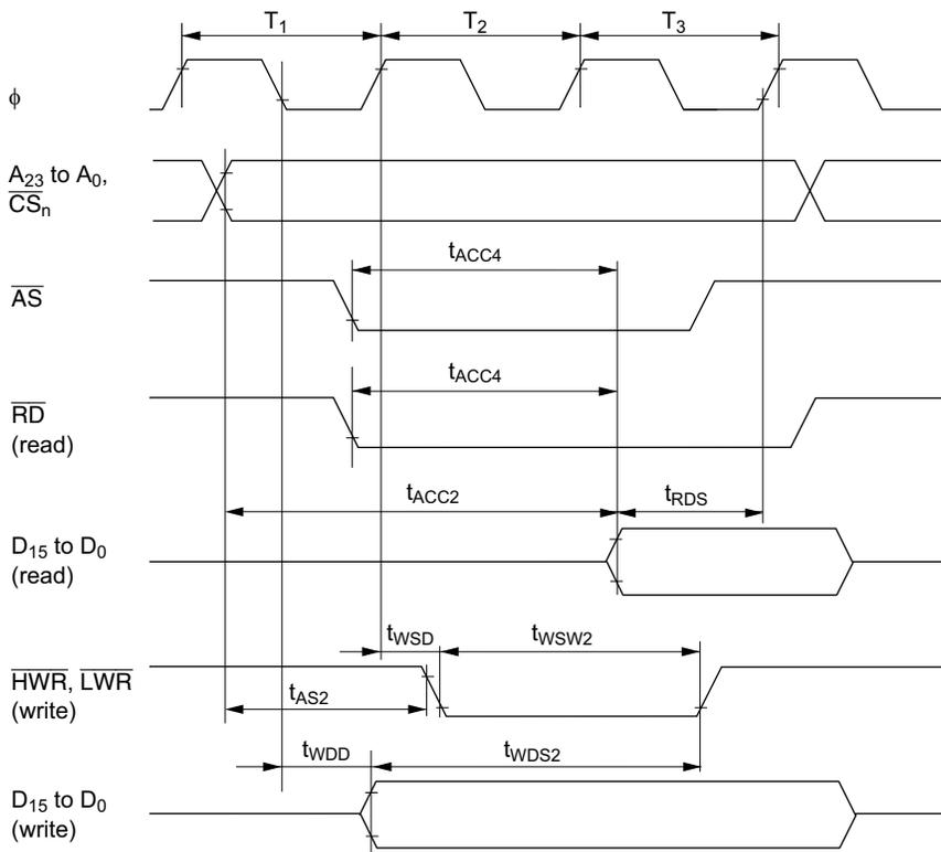
**Figure 21.12 Basic Bus Cycle: Three-State Access**
