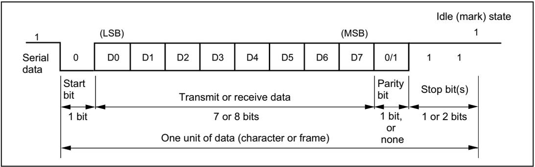
**Figure 13.2 Data Format in Asynchronous Communication
