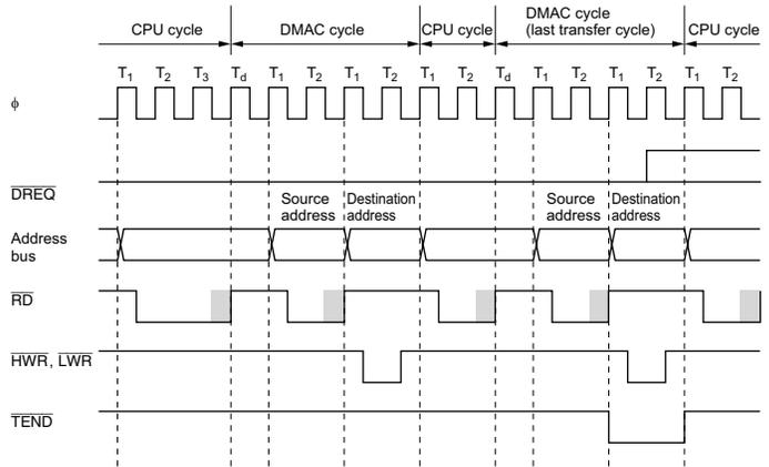
Figure 7.15 Burst DMA Bus Timing
