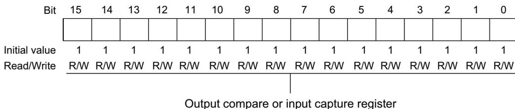
**TCR1 Timer Control Register 1****H'FFF70****16-bit timer channel 1**
