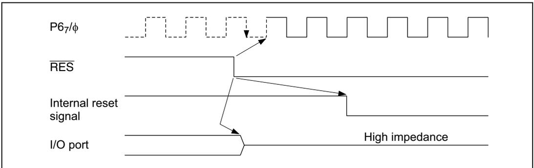
**Figure D.4 Reset during Operation (Modes 6 and 7)**
