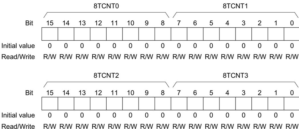
The timer counters (8TCNT) are 8-bit readable/writable up-counters that increment on pulses generated from an internal or external clock source. The clock source is selected by clock select bits 2 to 0 (CKS2 to CKS0) in the timer control register (8TCR). The CPU can always read or write to the timer counters.
