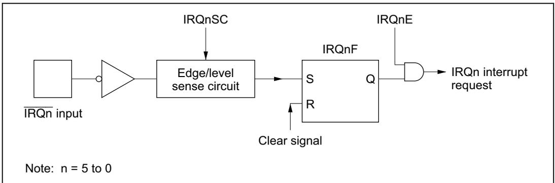
Figure 5.2 Block Diagram of Interrupts IRQ<sub>0</sub> to IRQ<sub>5</sub>
