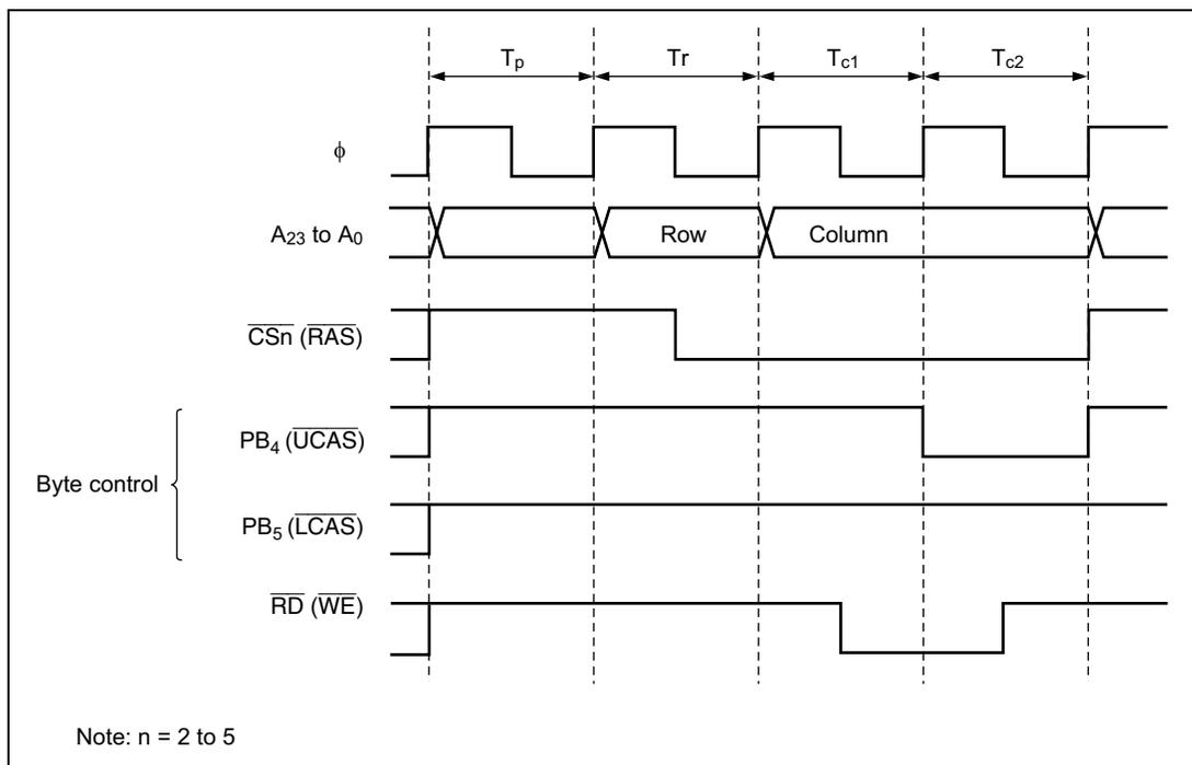
**Figure 6.21 Control Timing (Upper-Byte Write Access When  $CSEL = 0$ )**
