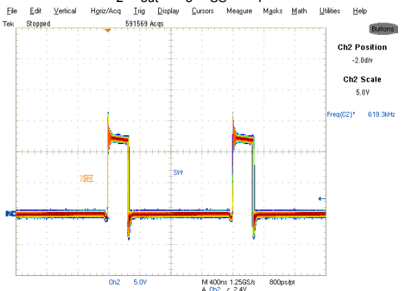
Fig. 25: Inductor node at 25A load Ch 2 :SW
