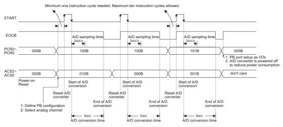
Note: A/D clock must be fsys/2, fsys/8 or fsys/32 tabcs=32tab tabc=80tab
