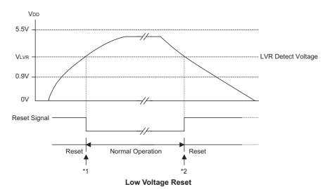
Note: \*1: To make sure that the system oscillator has stabilised, the SST provides an extra delay of 1024 system clock pulses before beginning normal operation.
