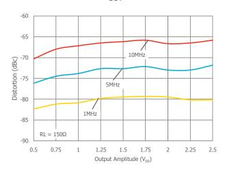
3rd Harmonic Distortion vs. V<sub>OUT</sub>
