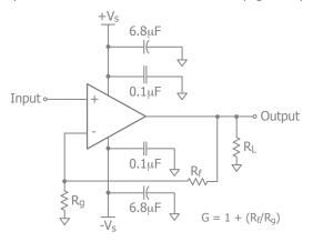
Figure 3. Typical Non-Inverting Gain Circuit
