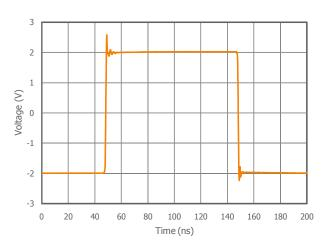
Large Signal Pulse Response at  $V_S = 5V$
