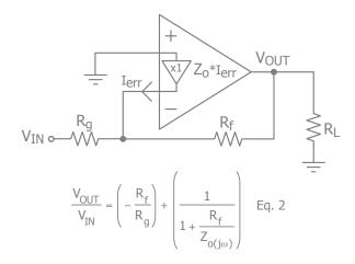
Figure 2. Inverting Gain Configuration with First Order
