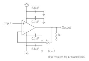
Figure 5. Typical Unity Gain (G=1) Circuit
