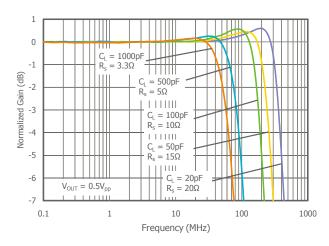
Frequency Response vs.  $V_{OUT}$  at  $V_S = 5V$
