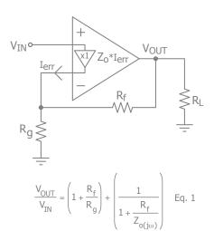
Figure 1. Non-Inverting Gain Configuration with First Order Transfer Function
