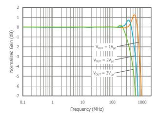
Inverting Frequency Response at  $V_S = 5V$
