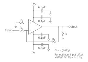
Figure 4. Typical Inverting Gain Circuit
