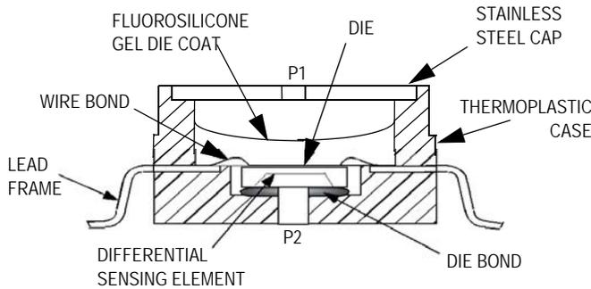
Figure 3. Cross-Sectional Diagram SOP (not to scale)
