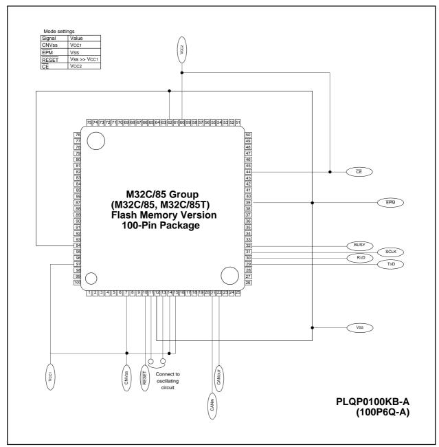
Figure 25.15 Pin Connections in Standard Serial I/O Mode (2)
