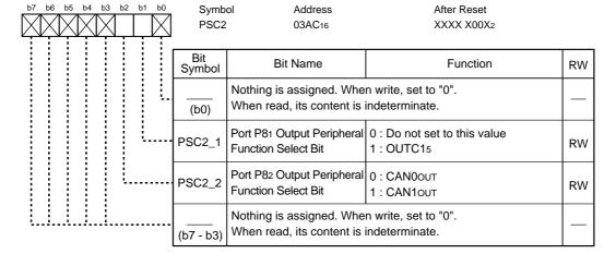
Figure 24.13 PSC Register and PSC2 Register
