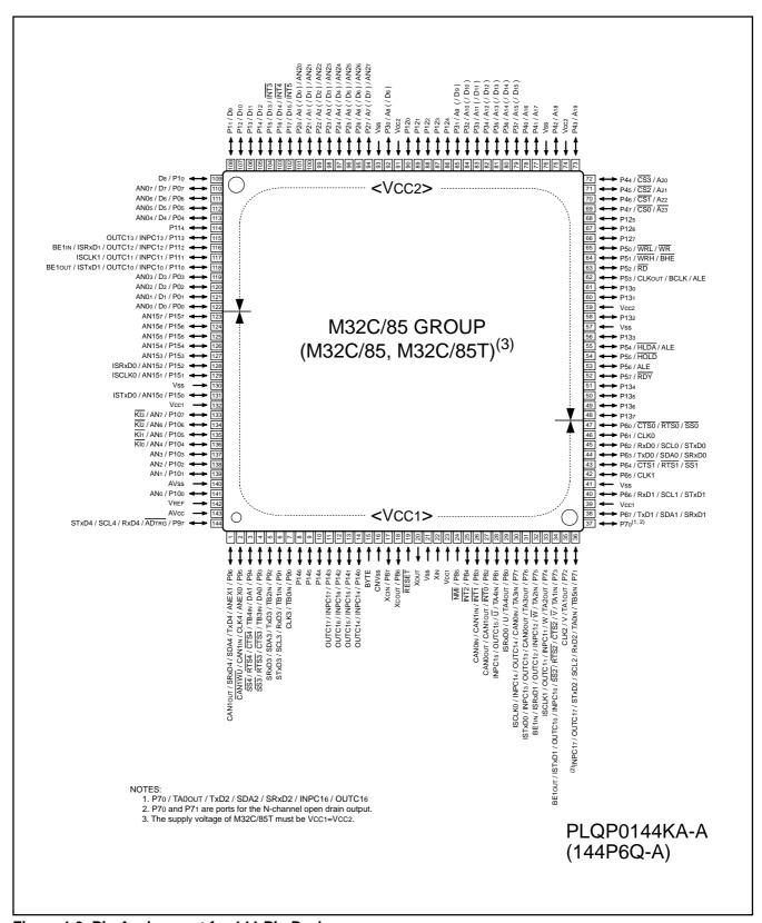
Figure 1.3 Pin Assignment for 144-Pin Package
