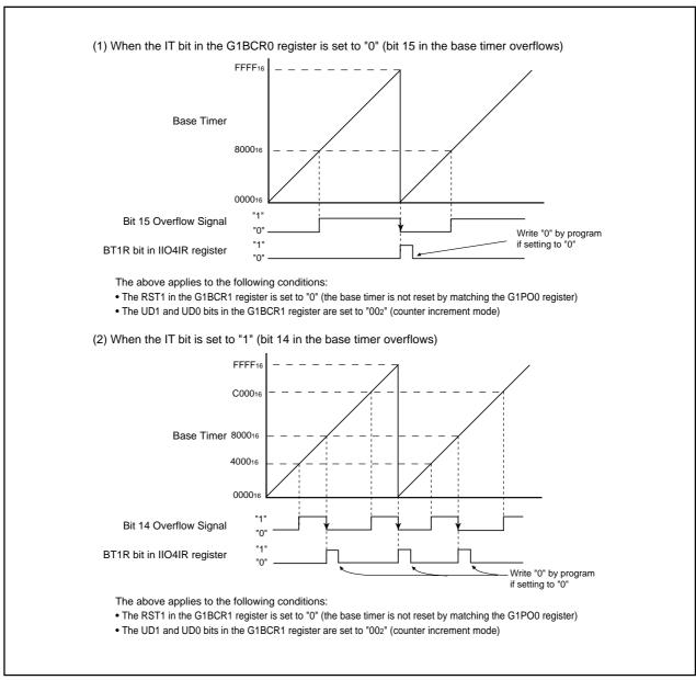
Figure 22.10 Counter Increment Mode
