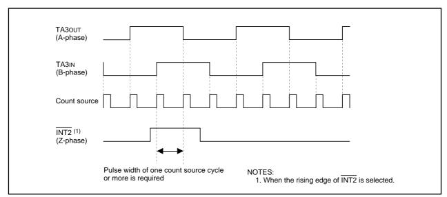
Figure 15.10 Two-Phase Pulse (A-phase and B-phase) and Z-phase
