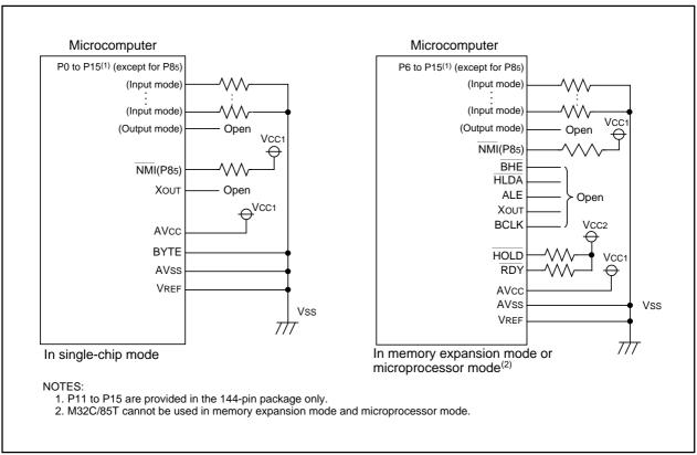
Figure 24.19 Unassigned Pin Handling
