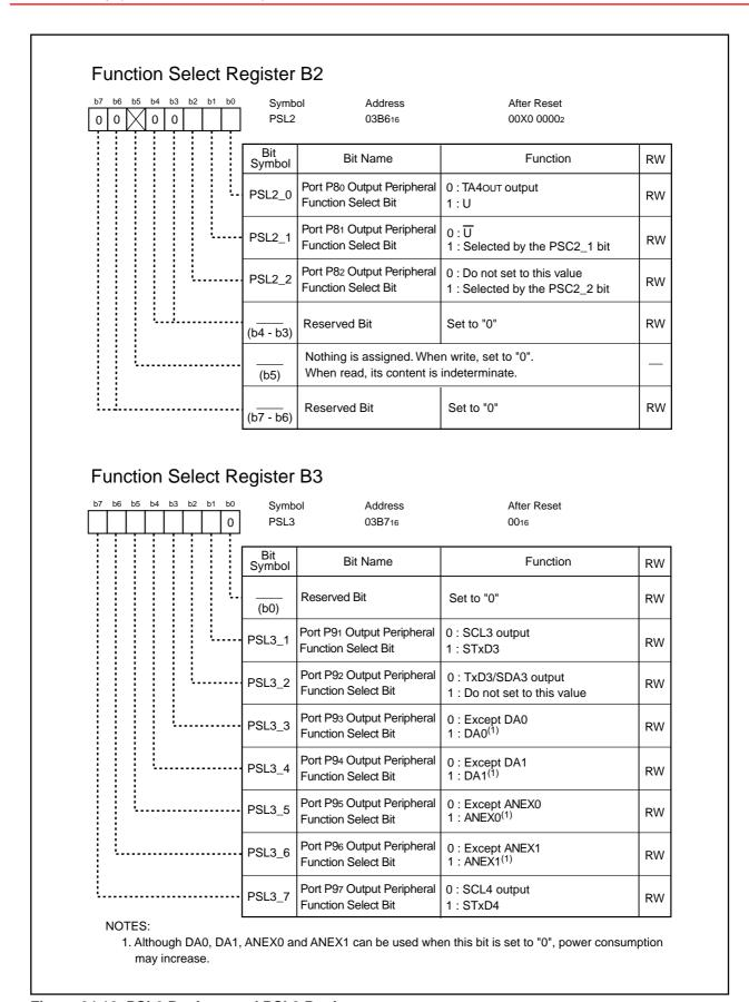
Figure 24.12 PSL2 Register and PSL3 Register
