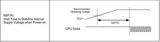
Figure 26.11 Power Supply Timing Diagram
