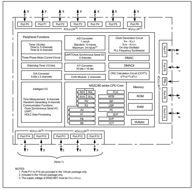
Figure 1.1 M32C/85 Group (M32C/85, M32C/85T) Block Diagram
