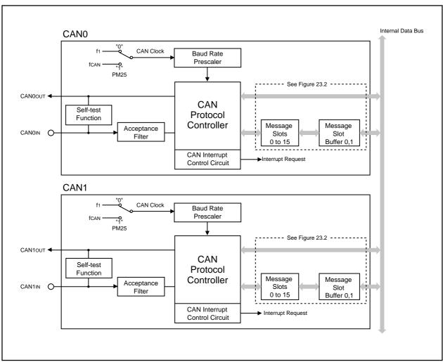
Figure 23.1 CAN Module Block Diagram
