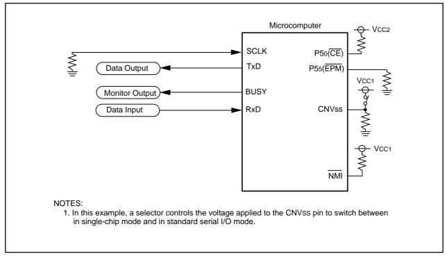
Figure 25.18 Circuit Application in Standard Serial I/O Mode 2
