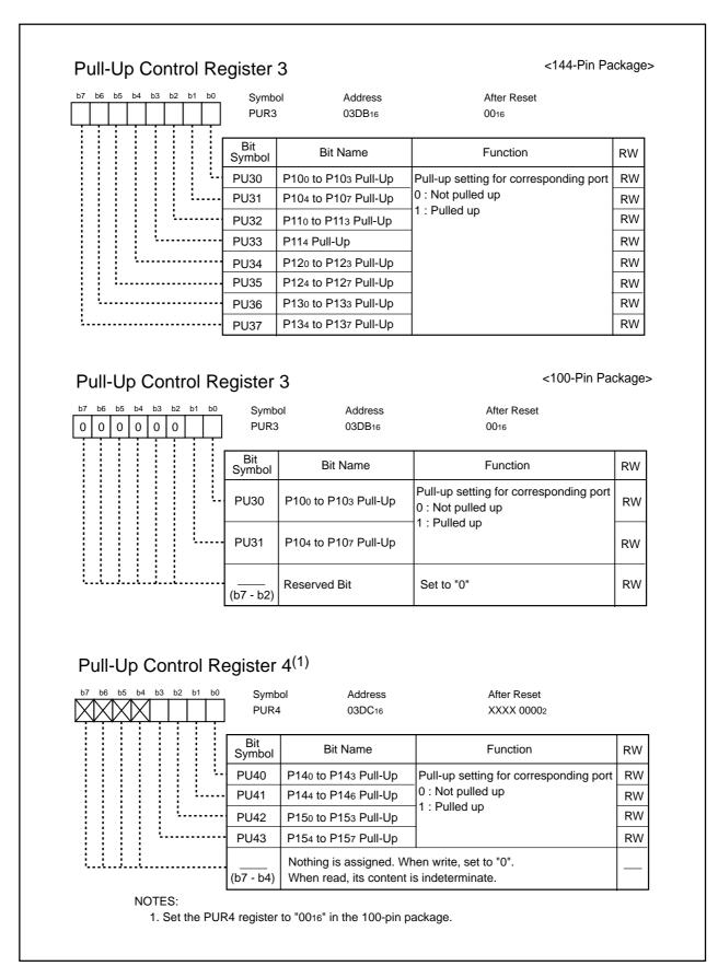
Figure 24.16 PUR3 Register and PUR4 Register
