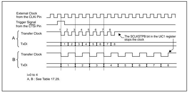
Figure 17.27 Clock-Divided Synchronous Function
