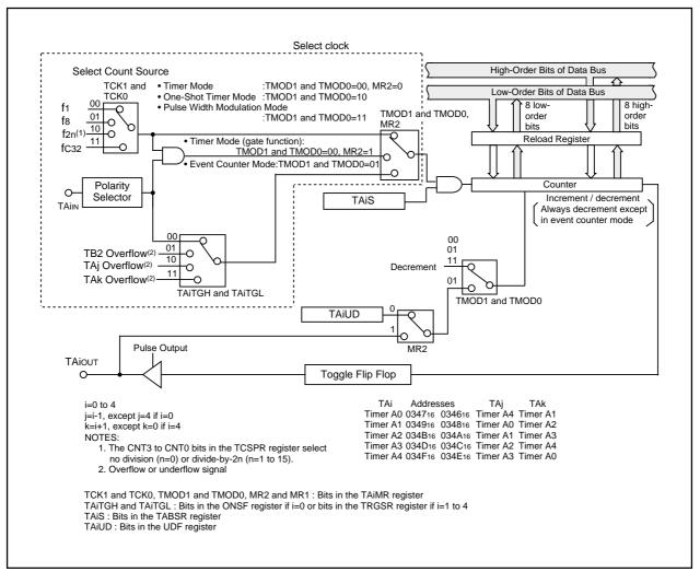
Figure 15.3 Timer A Block Diagram
