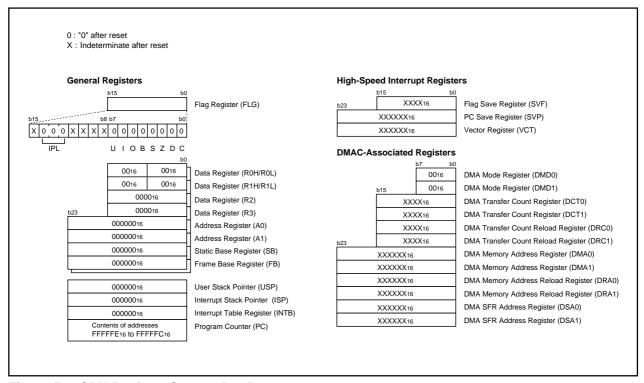
Figure 5.4 CPU Register States after Reset
