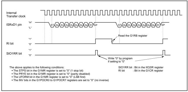
Figure 22.32 Receive Operation
