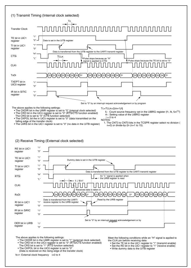
Figure 17.10 Transmit and Receive Operation
