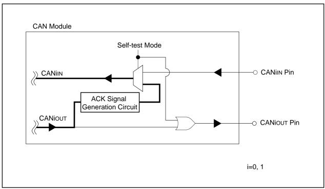
Figure 23.19 Self-Test Mode
