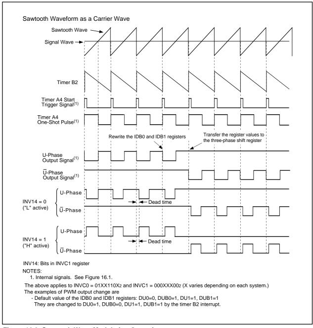
Figure 16.9 Sawtooth Wave Modulation Operation
