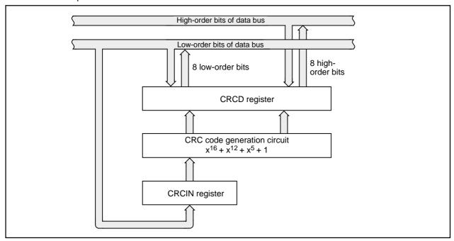
Figure 20.1 CRC Calculation Block Diagram
