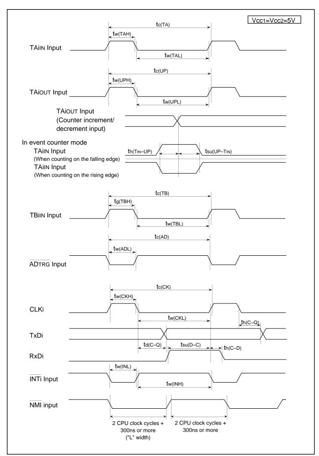
Figure 26.5 VCC1=VCC2=5V Timing Diagram (3)
