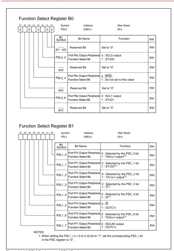
Figure 24.11 PSL0 Register and PSL1 Register
