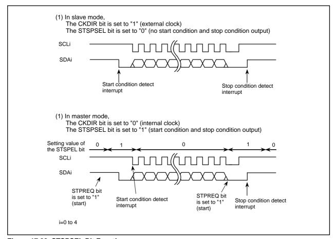
Figure 17.22 STSPSEL Bit Function
