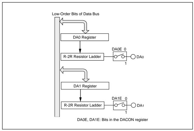
Figure 19.1 D/A Converter
