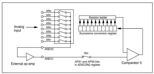
Figure 18.7 External Op-Amp Connection
