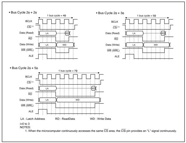
Figure 8.7 Bus Cycle with Multiplexed Bus (1)
