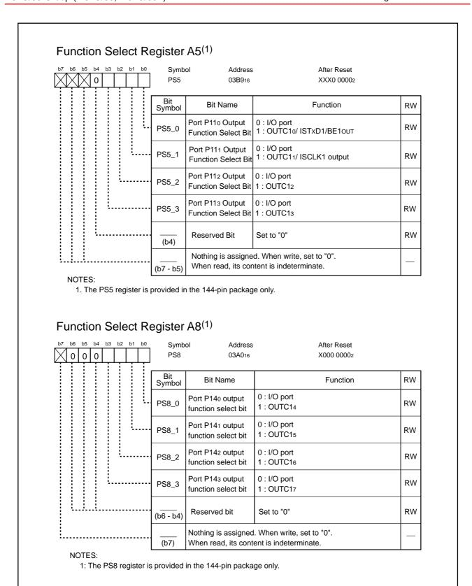
Figure 24.9 PS5 Register and PS8 Register
