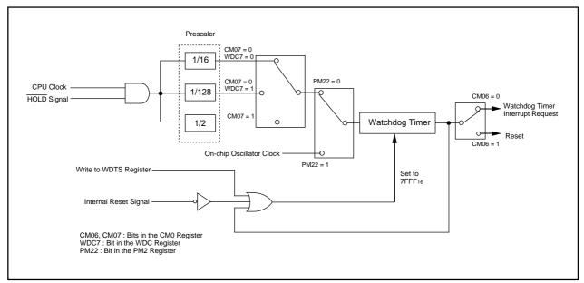
Figure 12.1 Watchdog Timer Block Diagram
