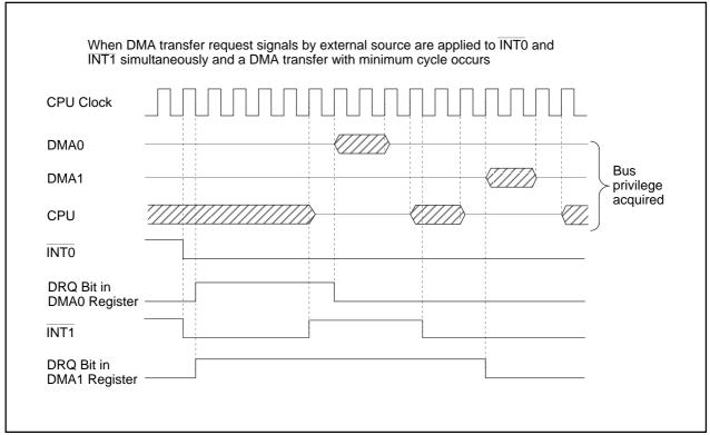
Figure 13.7 DMA Transfer by External Source
