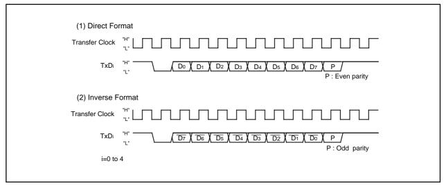
Figure 17.32 SIM Interface Format
