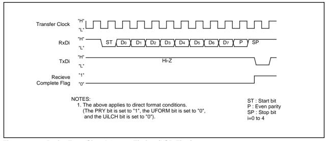
Figure 17.31 Parity Error Signal Output Timing (LSB First)
