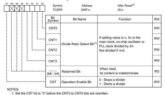
Figure 15.7 TRGSR Register and TCSPR Register
