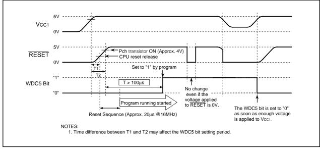
Figure 6.8 Cold Start-up/Warm Start-up Determine Function Operation
