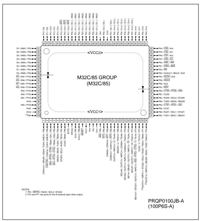
Figure 1.5 Pin Assignment for 100-Pin Package
