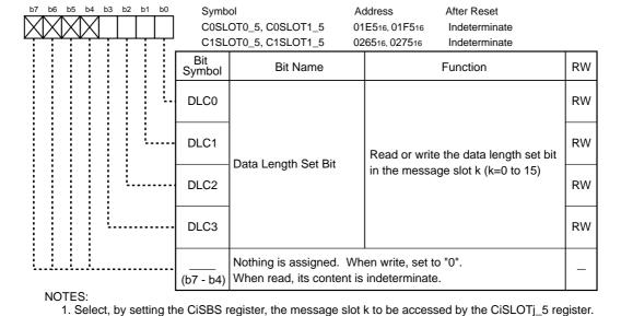
Figure 23.33 C0SLOT0\_4, C0SLOT1\_4, C0SLOT0\_5 and C0SLOT1\_5 Registers C1SLOT0\_4, C1SLOT1\_4, C1SLOT0\_5 and C1SLOT1\_5 Registers
