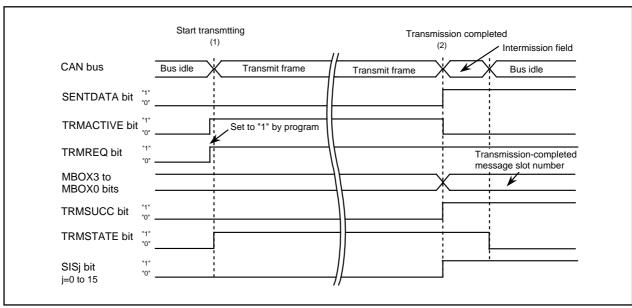
Figure 23.38 Example of CAN Data Frame Transmit Operation
