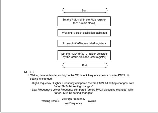
Figure 23.36 Accessing Procedure for CAN-Associated Registers
