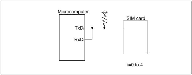
Figure 17.30 SIM Interface Connection
