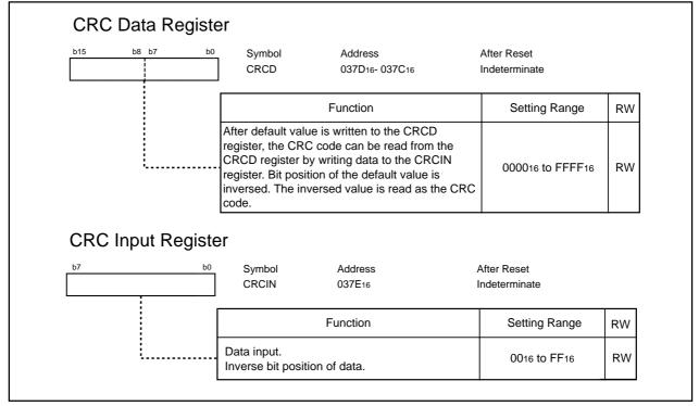
Figure 20.2 CRCD Register and CRCIN Register
