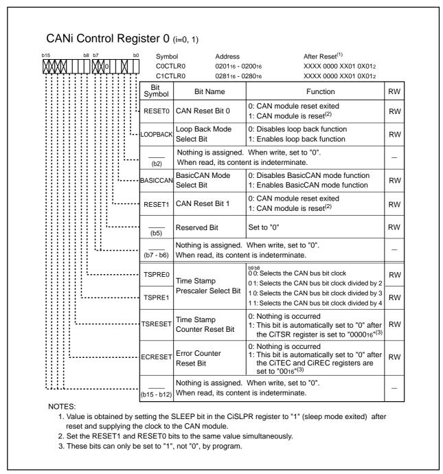
Figure 23.3 C0CTLR0 and C1CTLR0 Registers
