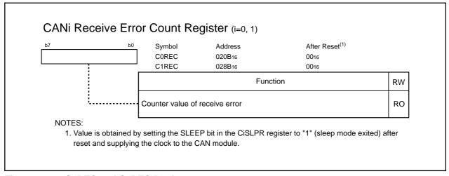
Figure 23.12 COREC and C1REC Registers
