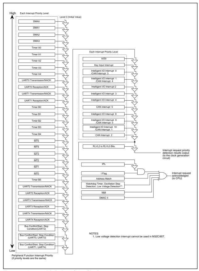
Figure 11.9 Interrupt Priority Level Select Circuit
