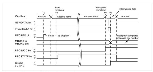
Figure 23.39 Example of CAN Data Frame Receive Operation
