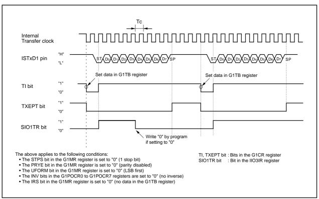
Figure 22.31 Transmit Operation
