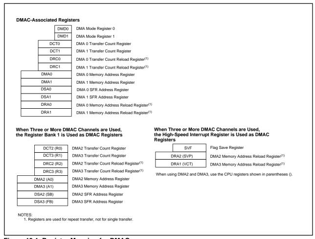
Figure 13.1 Register Mapping for DMAC
