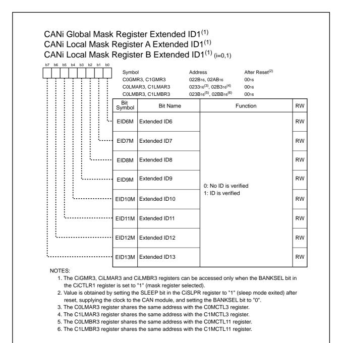
Figure 23.25 C0GMR3, C0LMAR3 and C0LMBR3 Registers C1GMR3, C1LMAR3 and C1LMBR3 Registers
