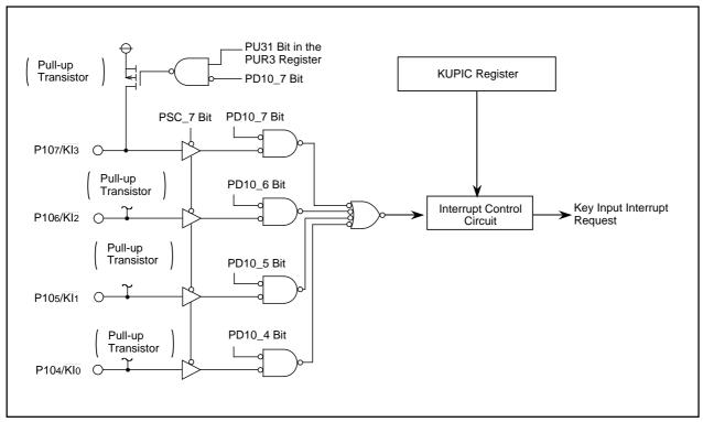
Figure 11.11 Key Input Interrupt
