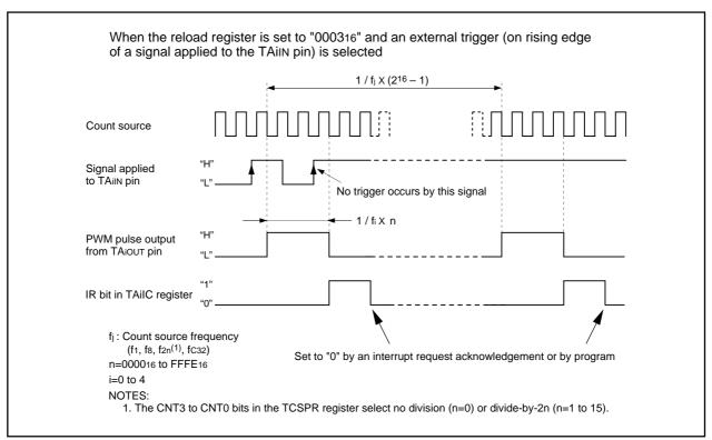
Figure 15.14 16-bit Pulse Width Modulator Operation
