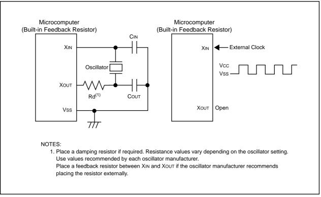
Figure 9.9 Main Clock Circuit Connection
