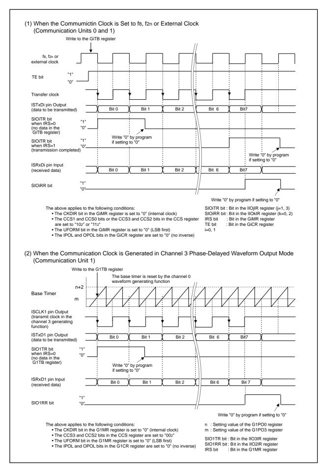
Figure 22.30 Transmit and Receive Operation
