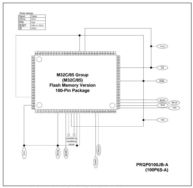
Figure 25.14 Pin Connections in Standard Serial I/O Mode (1)
