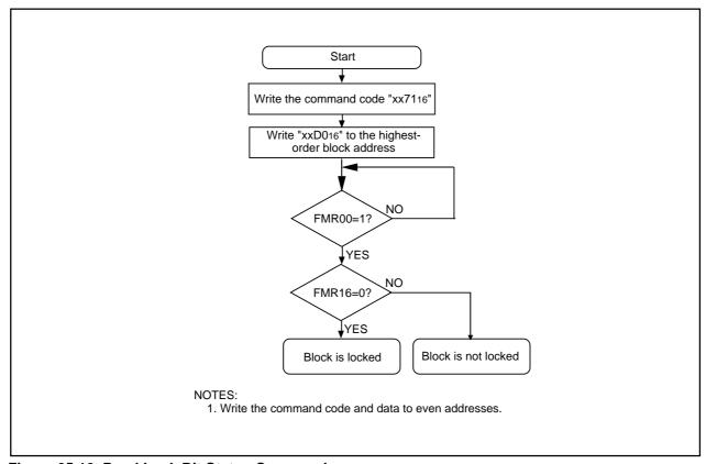
Figure 25.12 Read Lock Bit Status Command
