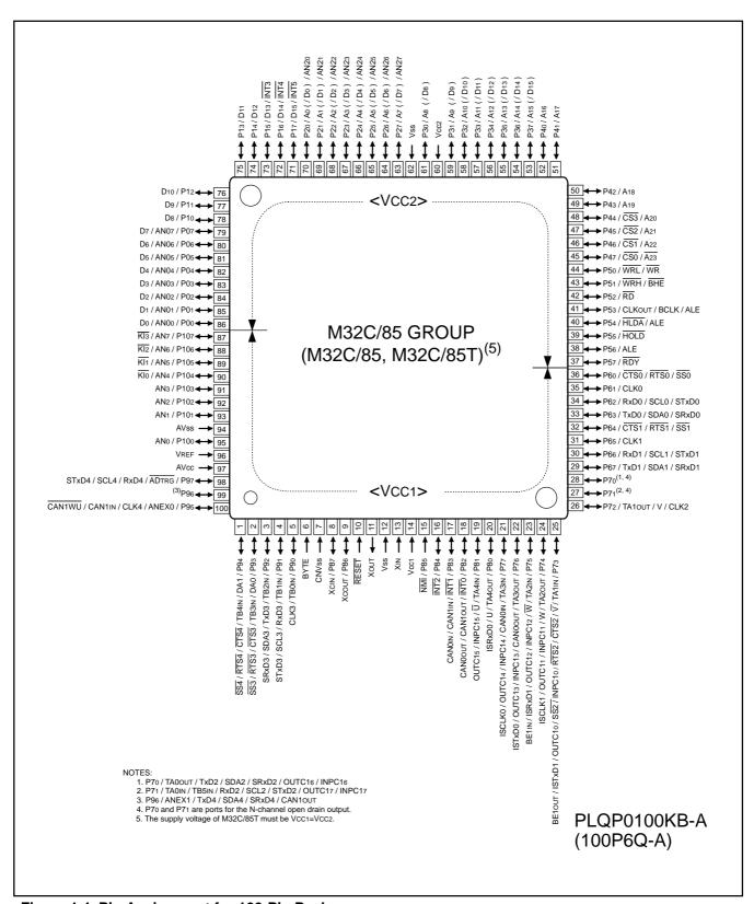
Figure 1.4 Pin Assignment for 100-Pin Package
