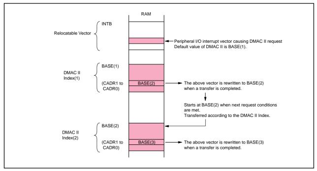
Figure 14.4 Relocatable Vector and DMAC II Index
