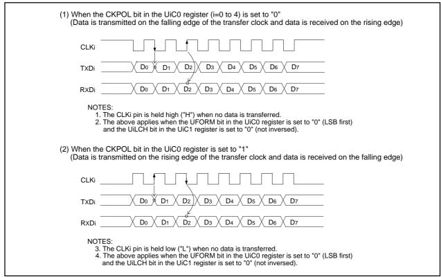
Figure 17.11 Transfer Clock Polarity
