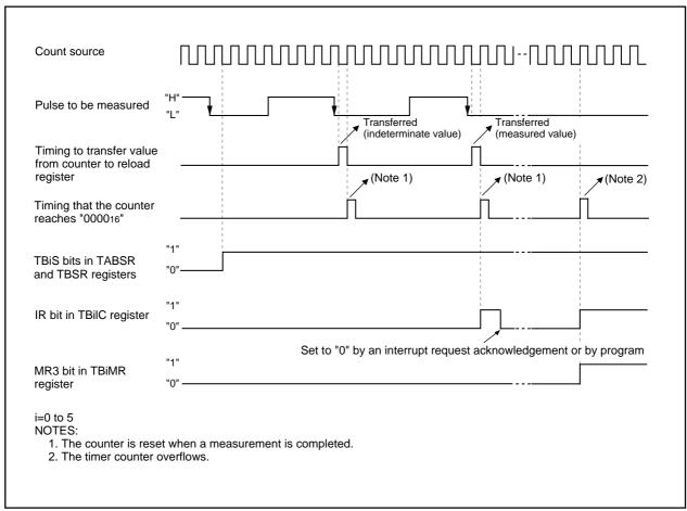
Figure 15.23 Operation Example in Pulse Period Measurement Mode
