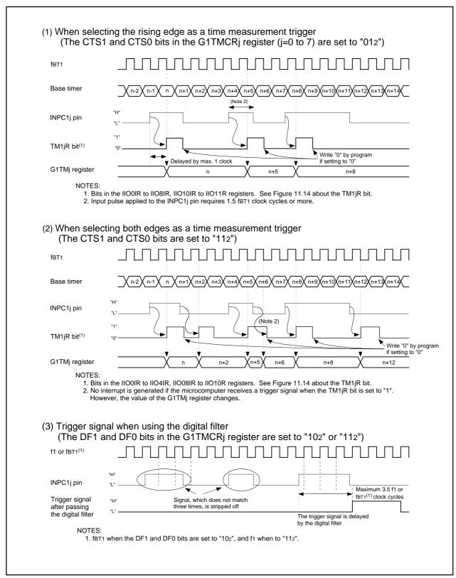
Figure 22.14 Time Measurement Function (2)
