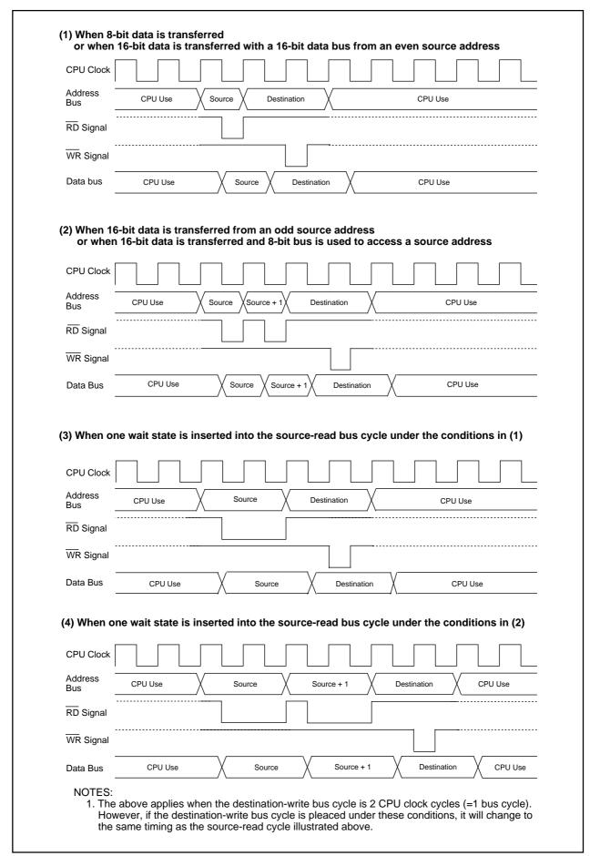
Figure 13.6 Transfer Cycle Examples with the Source-Read Bus Cycle
