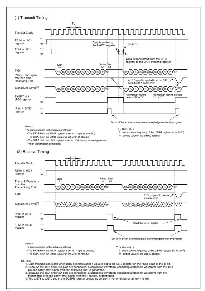
Figure 17.29 SIM Interface Operation
