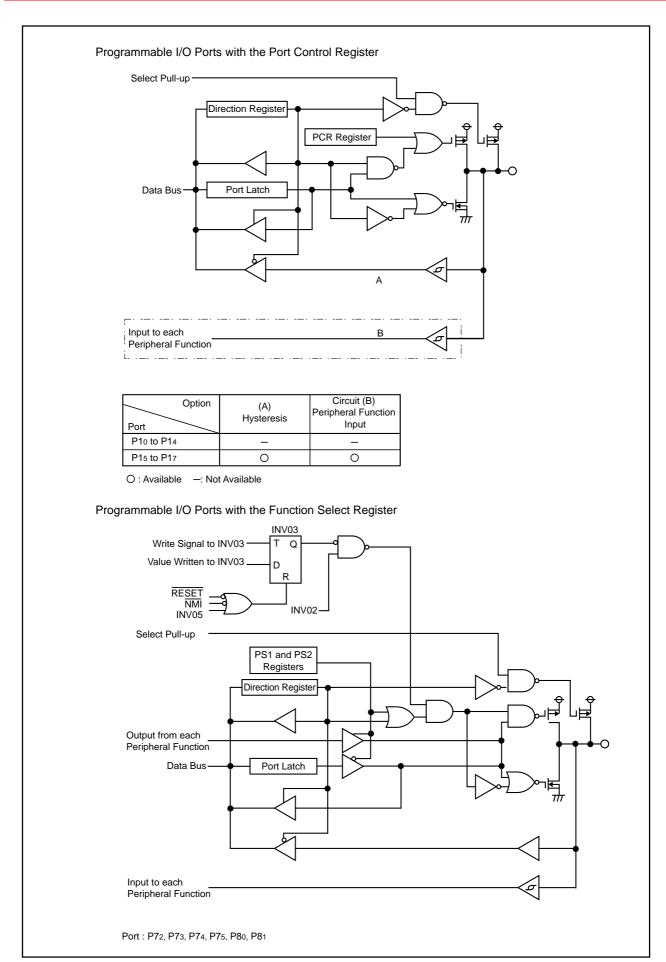
Figure 24.2 Programmable I/O Ports (2)
