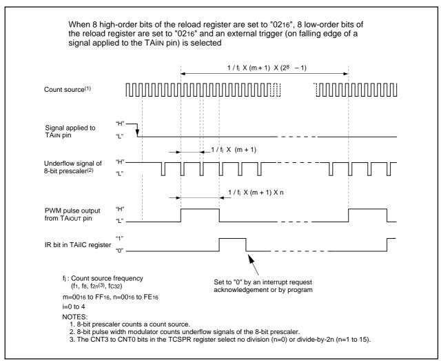
Figure 15.15 8-bit Pulse Width Modulator Operation
