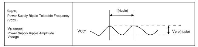
Figure 27.2 Power Supply Fluctuation Timing
