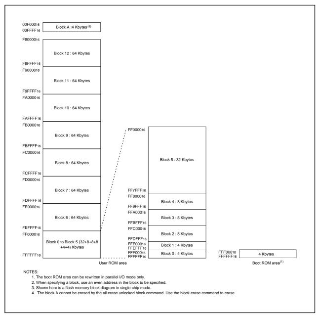
Figure 25.1 Flash Memory Block Diagram
