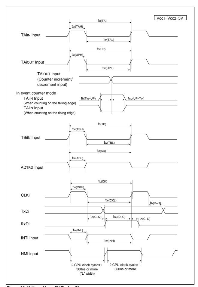
Figure 26.13 VCC1=VCC2=5V Timing Diagram
