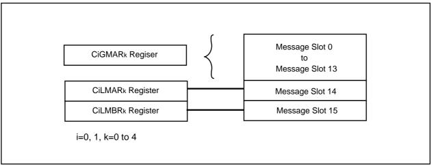
Figure 23.27 Mask Registers and Message Slots
