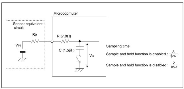
Figure 18.8 Analog Input Pin and External Sensor Equivalent Circuit
