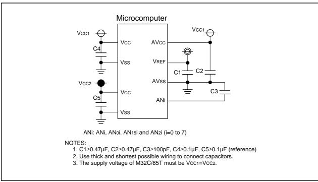
Figure 27.4 Use of Capacitors to Reduce Noise
