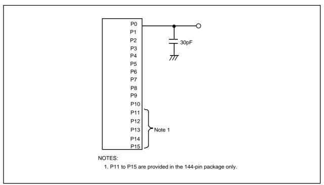
Figure 26.2 P0 to P15 Measurement Circuit
