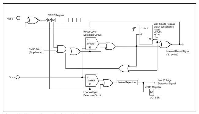
Figure 6.1 Voltage Detection Circuit Block Diagram
