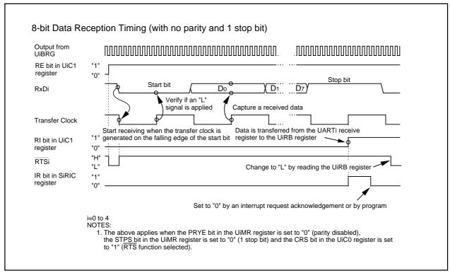
Figure 17.15 Receive Operation
