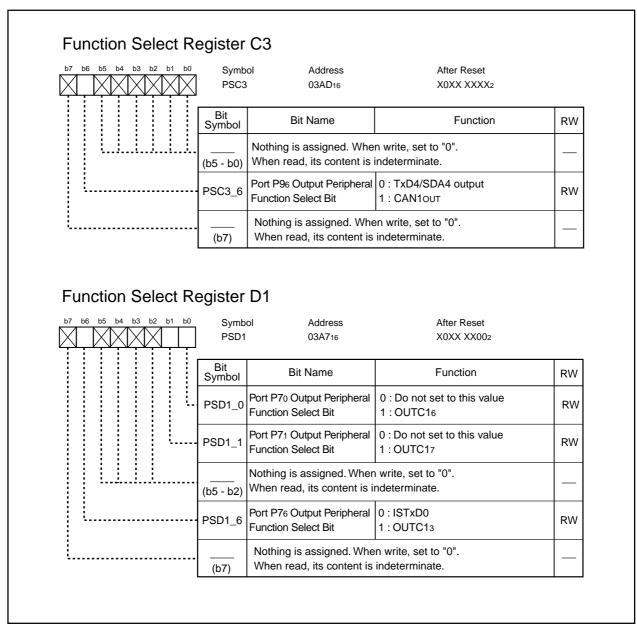
Figure 24.14 PSC3 Register and PSD1 Register
