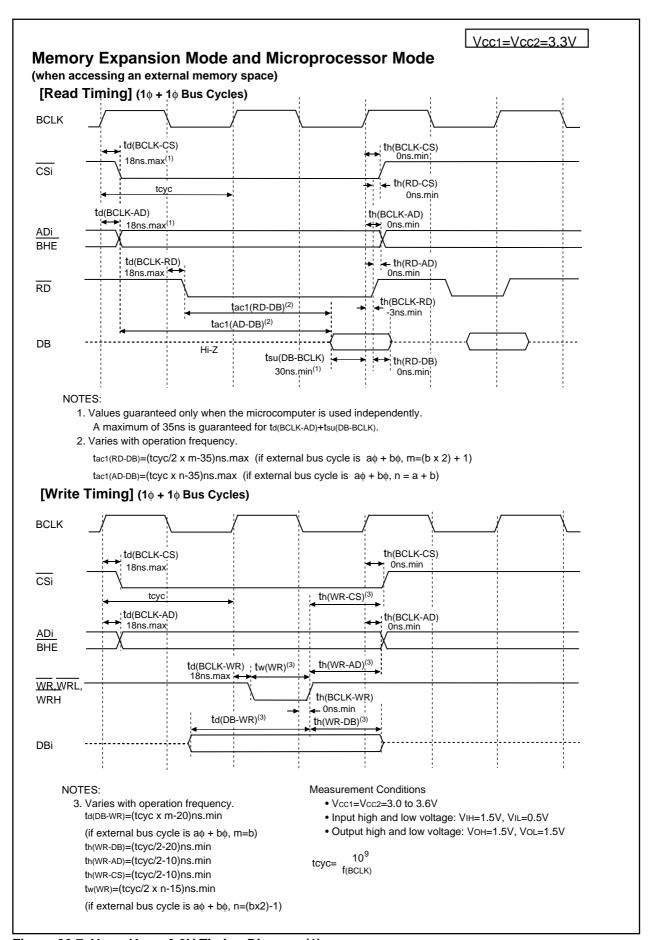
Figure 26.7 Vcc1=Vcc2=3.3V Timing Diagram (1)
