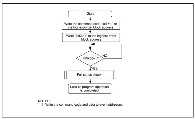
Figure 25.11 Lock Bit Program Command
