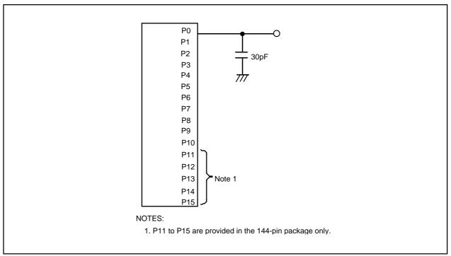
Figure 26.12 P0 to P15 Measurement Circuit
