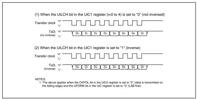
Figure 17.13 Serial Data Logic Inverse
