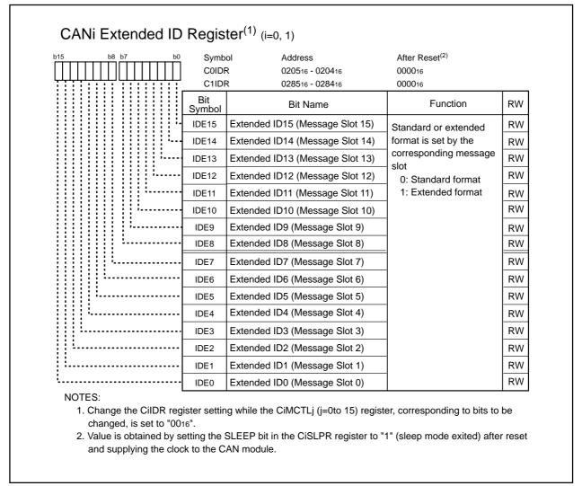
Figure 23.7 C0IDR and C1IDR Registers
