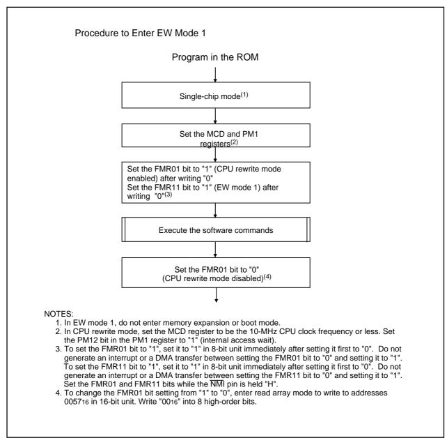
Figure 25.7 How to Enter and Exit EW Mode 1
