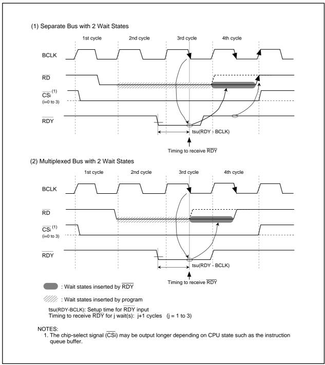
Figure 8.11 RD Signal Output Extended by RDY Signal
