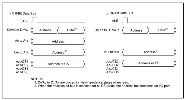
Figure 8.10 ALE Signal and Address/Data Bus
