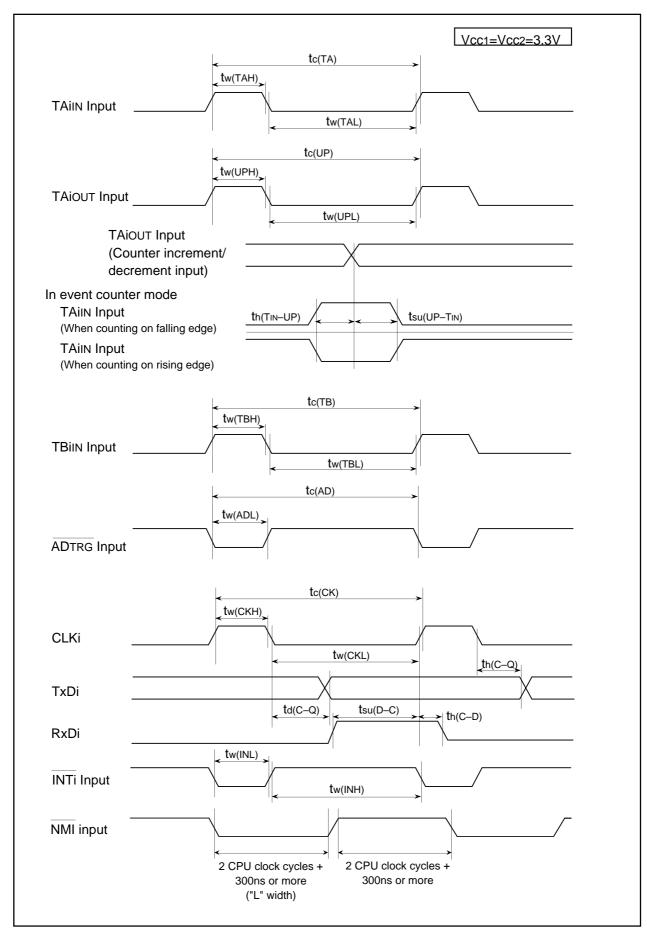
Figure 26.9 Vcc1=Vcc2=3.3V Timing Diagram (3)
