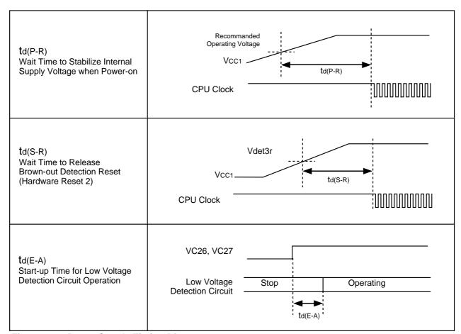
Figure 26.1 Power Supply Timing Diagram
