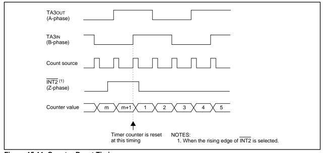
Figure 15.11 Counter Reset Timing
