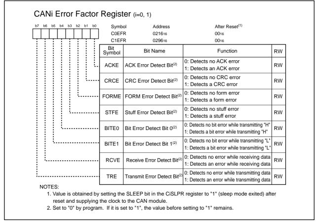
Figure 23.17 C0EFR and C1EFR Registers
