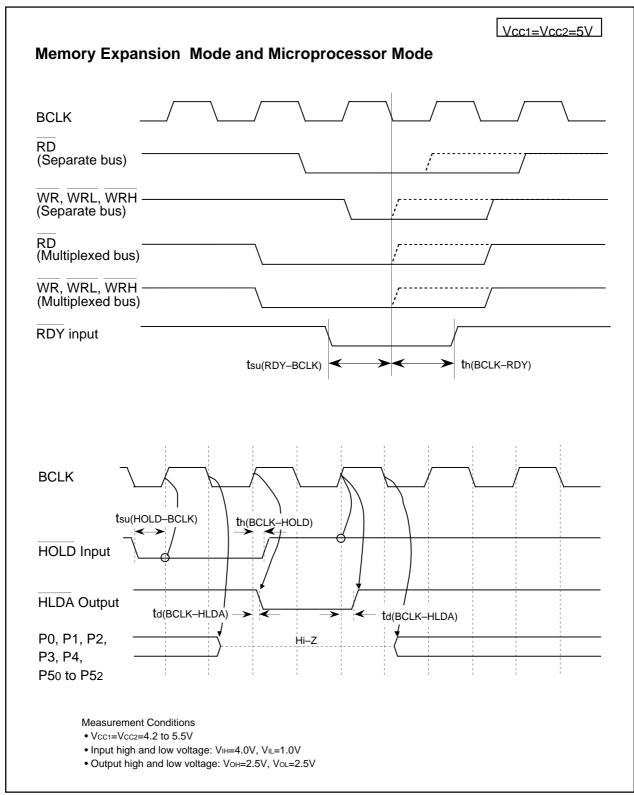
Figure 26.6 Vcc1=Vcc2=5V Timing Diagram (4)
