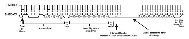
Figure 2. Inadvertent 8-Bit Read from 16-Bit Register where D7 is Zero
