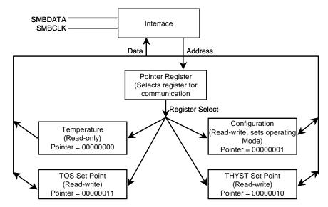
There are four data registers in the G751, selected by the Pointer register. At power-up the Pointer is set to "00"; the location for the Temperature Register. The Pointer register latches whatever the last location it was set to. In Interrupt Mode, a read from the G751, or placing the device in shutdown mode, resets the O.S. output. All registers are read and write, except the Temperature register which is read only.
