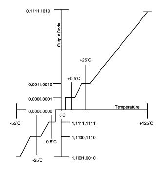
Temperature-to-Digital Transfer Function (Non-linear scale for clarity)
