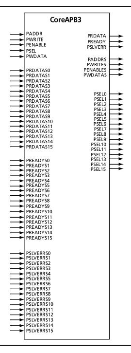
Figure 2 • CoreAPB3 Pinout
