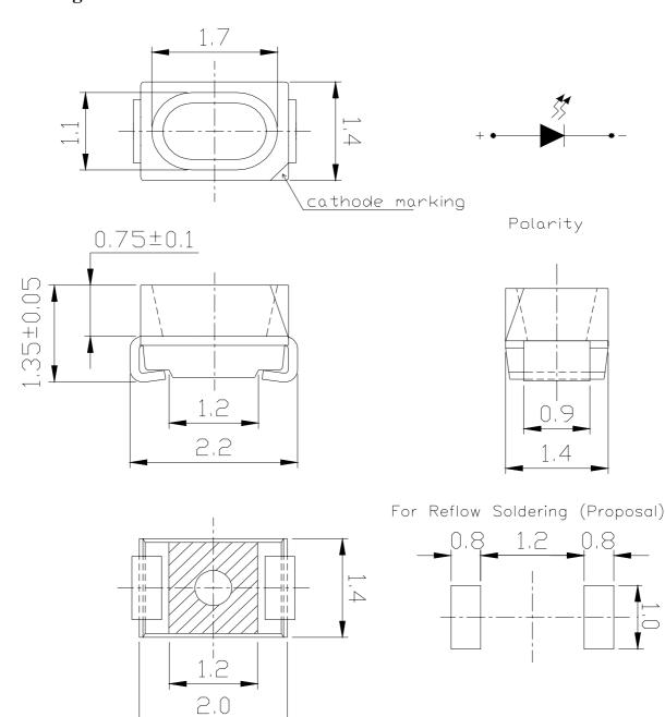
Notes: Tolerance of Dimension : ±0.1mm. Unit = mm
