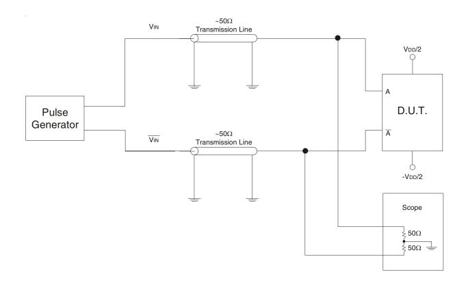
Test Circuit for Differential Input
