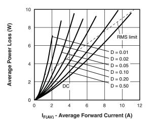
Fig. 6 - Forward Power Loss Characteristics
