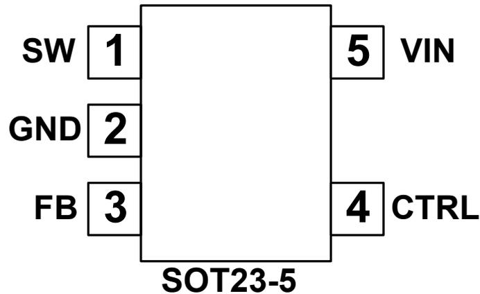
Figure 2: Pin Configuration
