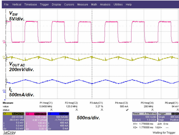
Steady State Operation V_{IN} = 5V, 39 LEDs, 260mA
