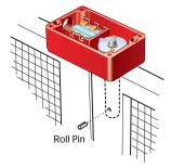
Solid Shaft The solid actuator shaft can be used as the hinge pin on certain guards.
