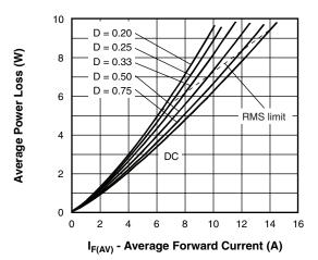
Fig. 6 - Forward Power Loss Characteristics (Per Leg)
