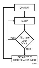
Figure 1. LTC2484 State Transition Diagram
