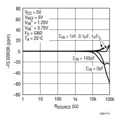
Figure 14. -FS Error vs R<sub>SOURCE</sub> at IN+ or IN-
