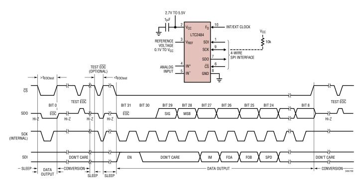
Figure 9. Internal Serial Clock, Reduce Data Output Length
