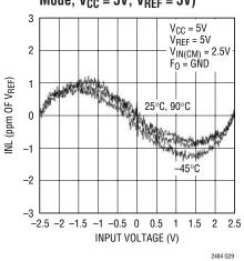
Integral Nonlinearity (2x Speed Mode;  $V_{CC} = 5V$ ,  $V_{REF} = 2.5V$ )
