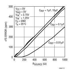
Figure 17. +FS Error vs R<sub>SOURCE</sub> at V<sub>REF</sub> (Large C<sub>REF</sub>)
