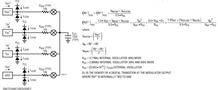
Figure 11. LTC2484 Equivalent Analog Input Circuit
