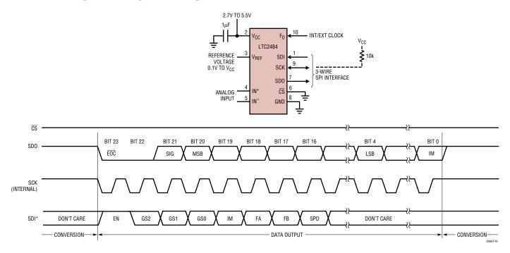
Figure 10. Internal Serial Clock,  $\overline{CS} = 0$  Continuous Operation
