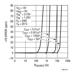
Figure 15. +FS Error vs R<sub>SOURCE</sub> at V<sub>REF</sub> (Small C<sub>REF</sub>)
