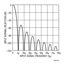
Figure 39. Input Normal Mode Rejection 2x Speed Mode
