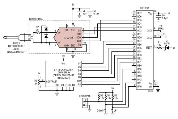
Figure 44. Complete Type K Thermocouple Meter
