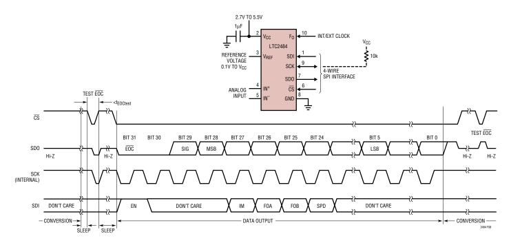
Figure 8. Internal Serial Clock, Single Cycle Operation
