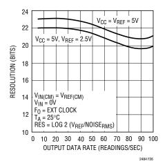
Figure 26. Resolution (Noise<sub>RMS</sub> ≤ 1LSB) vs Output Data Rate and Reference Voltage
