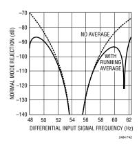
Figure 42. Input Normal Mode Rejection 2x Speed Mode
