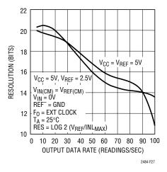
Figure 27. Resolution (INL $_{MAX} \le$  1LSB) vs Output Data Rate and Reference Voltage
