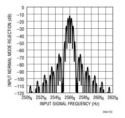
Figure 33. Input Normal Mode Rejection at f<sub>S</sub> = 256f<sub>N</sub>
