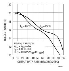
Figure 24. Resolution (INL $_{MAX} \le 1LSB$ ) vs Output Data Rate and Temperature
