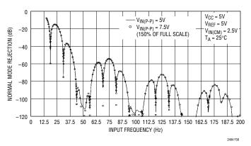
Figure 38. Measured Input Normal Mode Rejection vs Input Frequency with Input Perturbation of 150% Full Scale (50Hz Notch)
