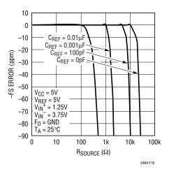
Figure 16. –FS Error vs  $R_{SOURCE}$  at  $V_{REF}$  (Small  $C_{REF}$ )
