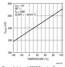
Figure 4. Internal PTAT Signal vs Temperature
