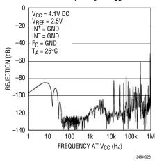
PSRR vs Frequency at V<sub>CC</sub>
