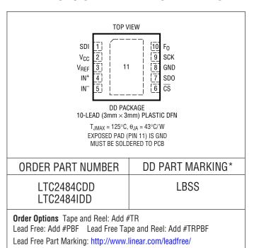
Consult LTC Marketing for parts specified with wider operating temperature ranges. \*The temperature grade is indicated by a label on the shipping container.
