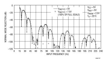
Figure 37. Measured Input Normal Mode Rejection vs Input Frequency with Input Perturbation of 150% Full Scale (60Hz Notch)
