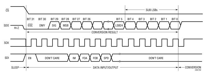
Figure 2. Input/Output Data Timing
