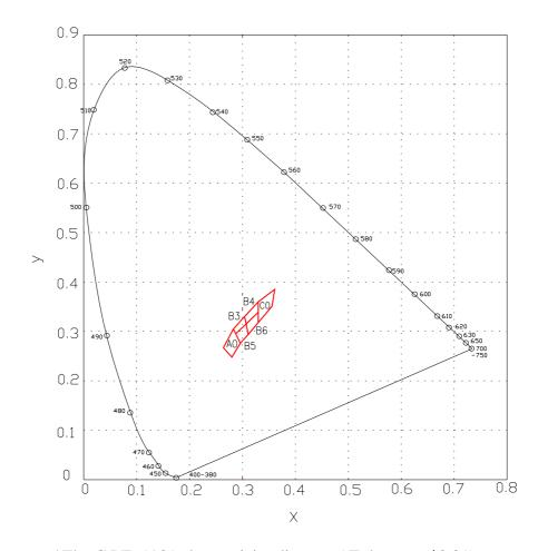
\*The C.I.E. 1931 chromaticity diagram (Tolerance ±0.01).
