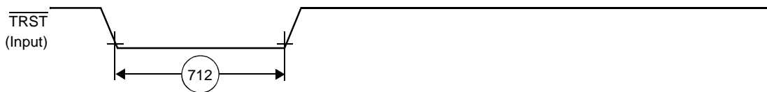
Figure 29. TRST Timing Diagram
