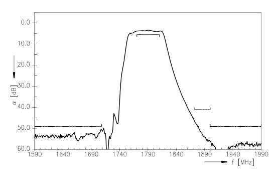
Transfer function  $S_{21} \left( \text{passband} \right)$  with matching network
