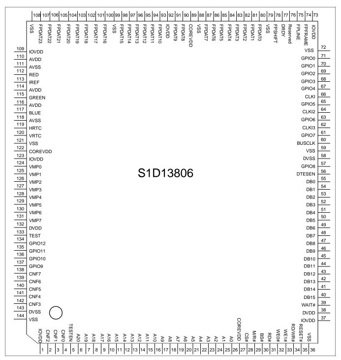
Figure 4-1: Pinout Diagram 144-Pin QFP20 Surface Mount Packages
