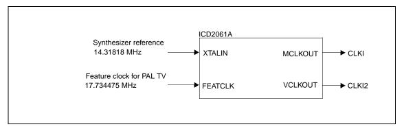
Figure 8-1: Symbolic Clock Synthesizer Connections
