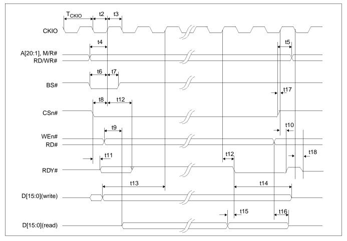
Figure 6-3: Hitachi SH-4 Interface Timing
