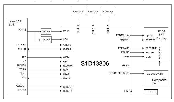
Figure 3-6: Typical System Diagram (Motorola Power PC Bus)
