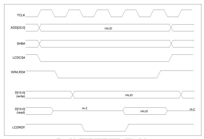
Figure 2-1: NEC VR4102/VR4111 Read/Write Cycles
