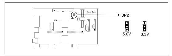
Figure 3-3: Configuration Jumper (JP2) Location
