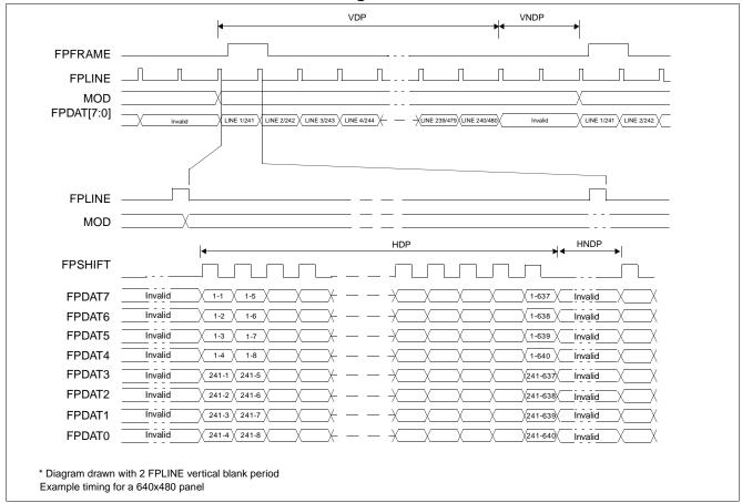
Figure 6-26: Dual Monochrome 8-Bit Panel Timing
