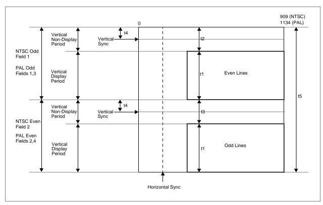
Figure 6-39: Vertical Timing for NTSC/PAL
