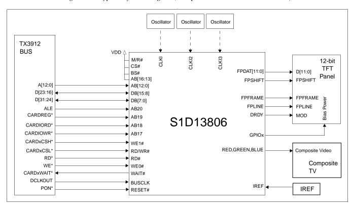
Figure 3-10: Typical System Diagram (Toshiba MIPS TX39xx Bus)
