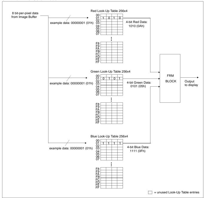
Figure 12-4: 8 Bit-Per-Pixel Color Mode Data Output Path
