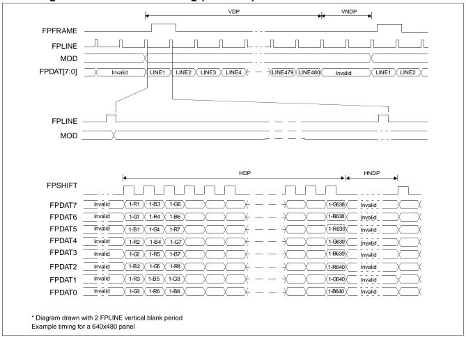
Figure 6-22: Single Color 8-Bit Panel Timing (Format 2)
