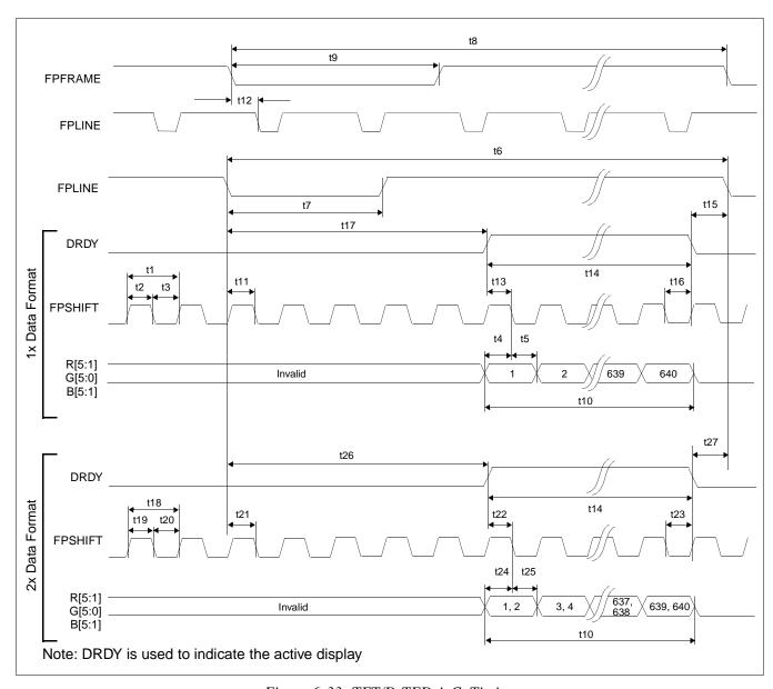
Figure 6-33: TFT/D-TFD A.C. Timing
