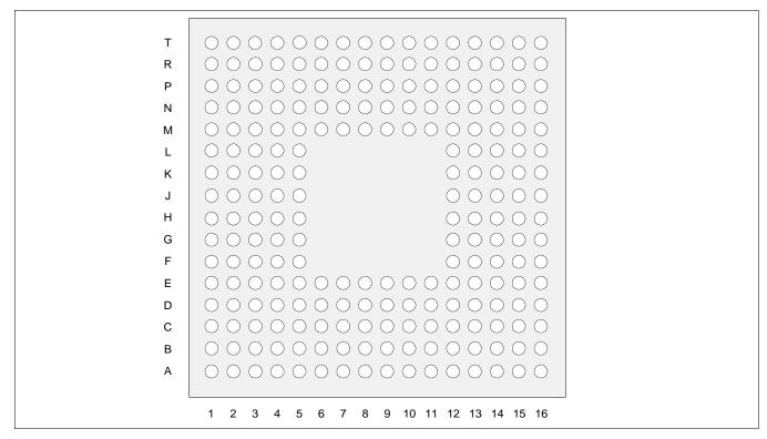
Figure 4-2: Pinout Diagram 220-Pin PFBGA Surface Mount Package
