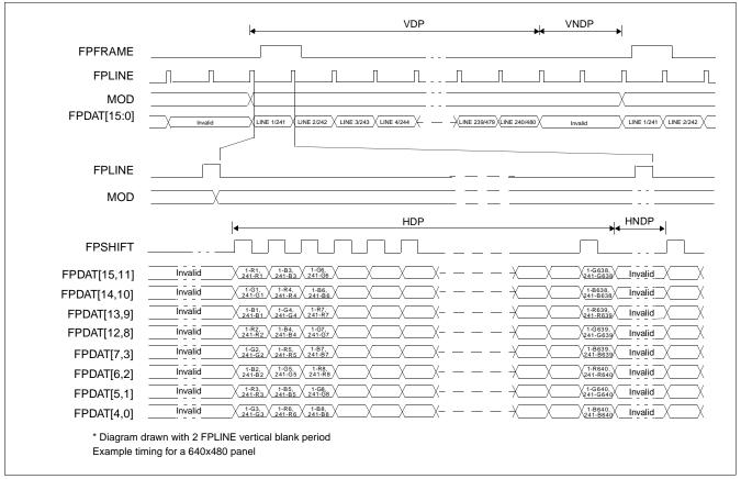
Figure 6-30: Dual Color 16-Bit Panel Timing
