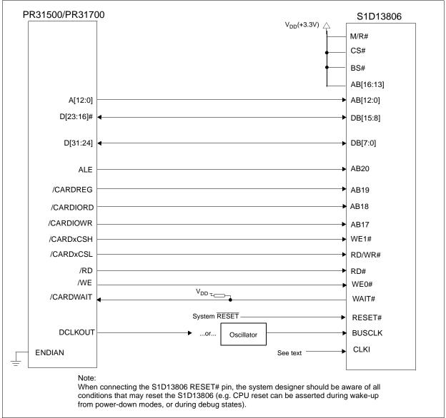
Figure 4-1: Typical Implementation of Direct Connection
