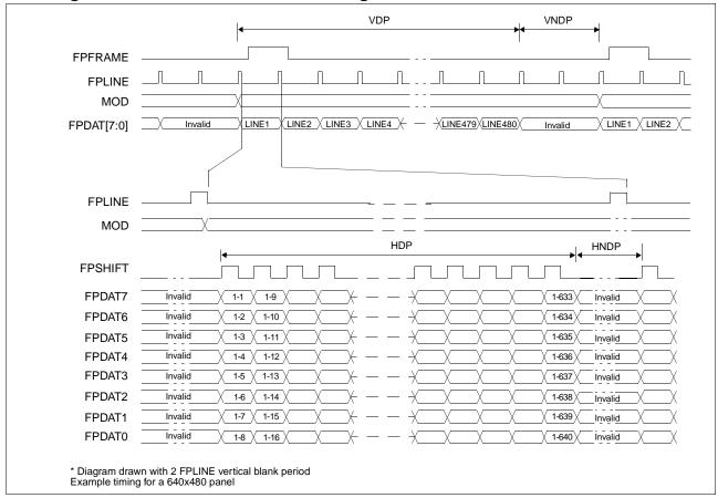
Figure 6-16: Single Monochrome 8-Bit Panel Timing
