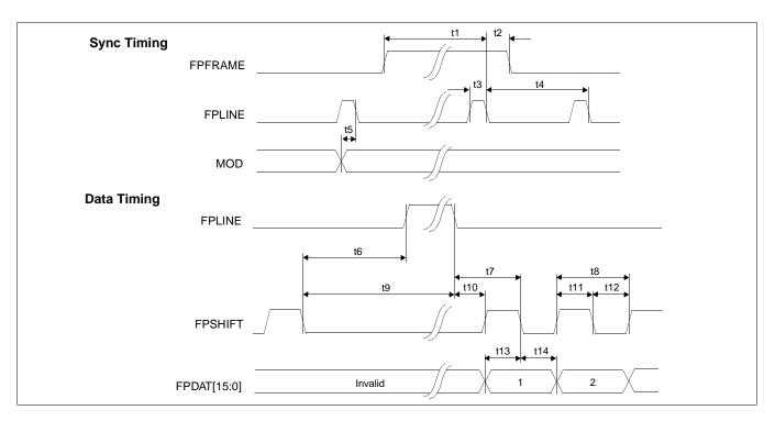
Figure 6-31: Dual Color 16-Bit Panel A.C. Timing
