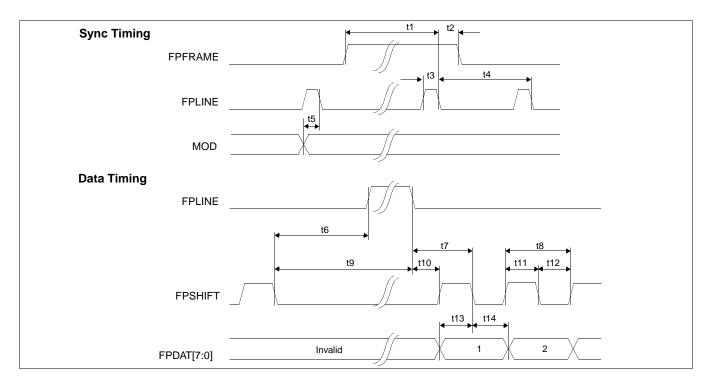
Figure 6-23: Single Color 8-Bit Panel A.C. Timing (Format 2)
