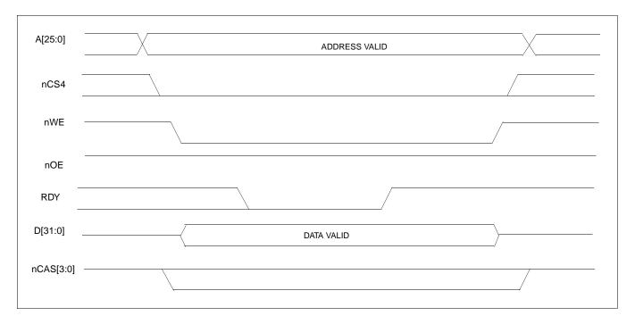
Figure 2-2: SA-1110 Variable-Latency IO Write Cycle
