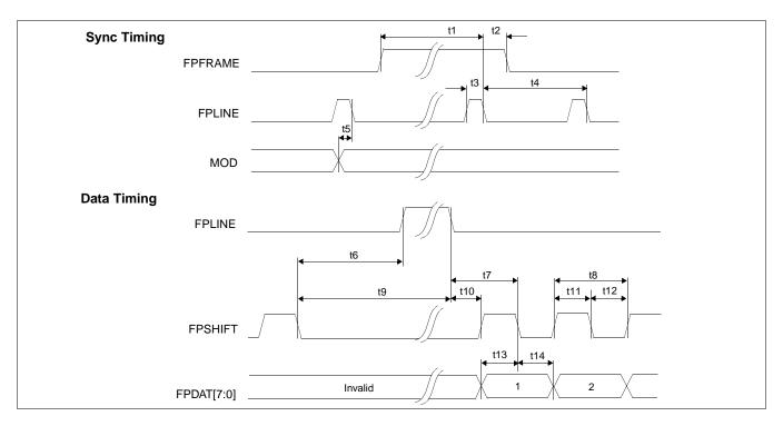
Figure 6-27: Dual Monochrome 8-Bit Panel A.C. Timing
