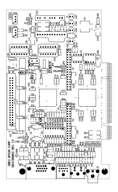
Figure 12-1: PCB Layout
