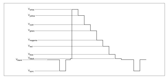
Figure 13-1: NTSC/PAL SVideo-Y (Luminance) Output Levels
