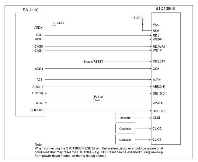
Figure 4-1: Typical Implementation of SA-1110 to S1D13806 Interface
