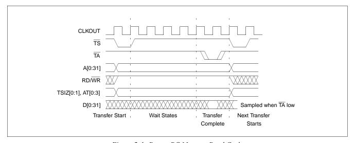
Figure 2-1: Power PC Memory Read Cycle
