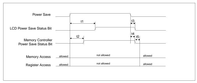
Figure 6-13: Power Save Status Bits and Local Bus Memory Access Relative to Power Save Mode
