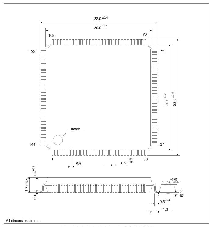
Figure 20-1: Mechanical Drawing 144-pin QFP20
