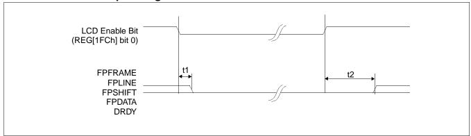
Figure 6-12: LCD Panel Power-off/Power-on Timing
