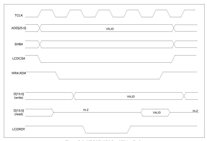
Figure 2-1: NEC VR4121 Read/Write Cycles
