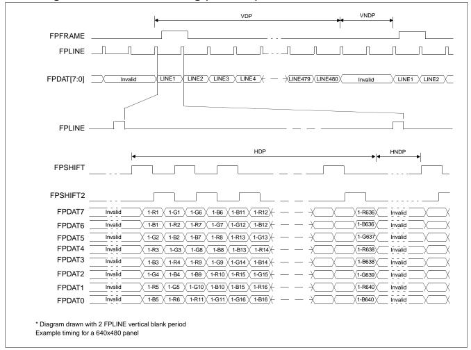
Figure 6-20: Single Color 8-Bit Panel Timing (Format 1)
