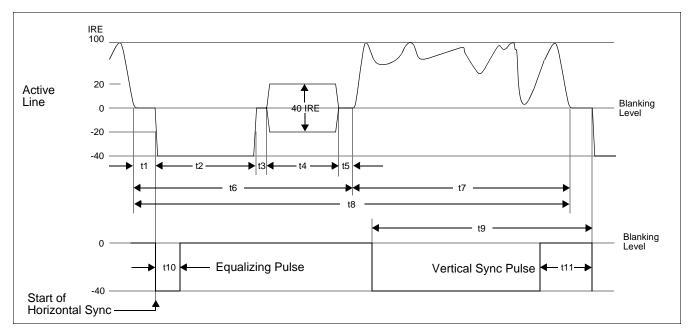
Figure 6-38: Horizontal Timing for NTSC/PAL
