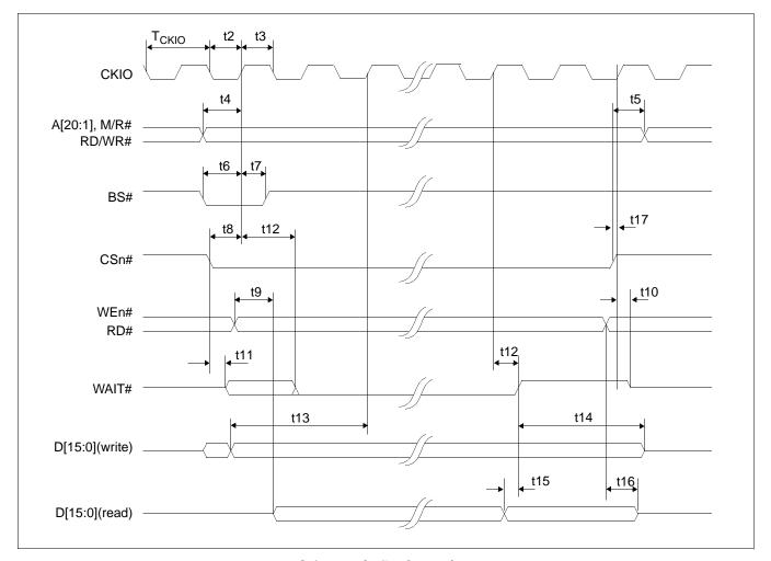
Figure 6-4: Hitachi SH-3 Interface Timing
