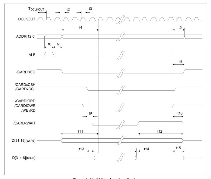
Figure 6-10: Philips Interface Timing
