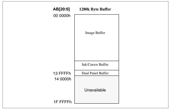
Figure 10-1: Display Buffer Addressing
