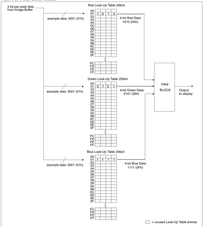
Figure 12-3: 4 Bit-Per-Pixel Color Mode Data Output Path
