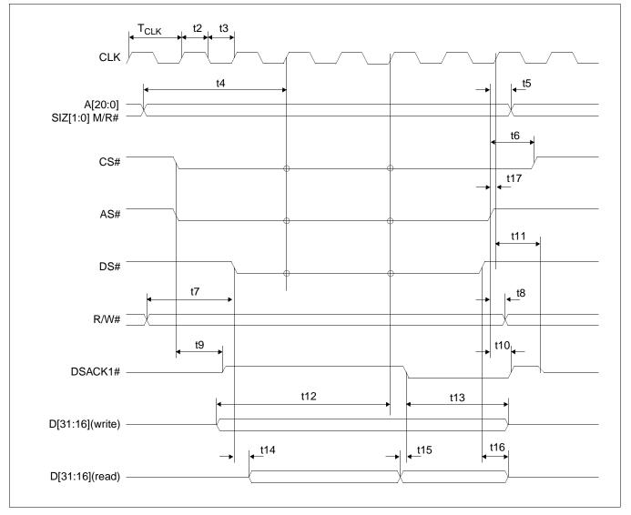
Figure 6-7: Motorola MC68K Bus 2 Interface Timing
