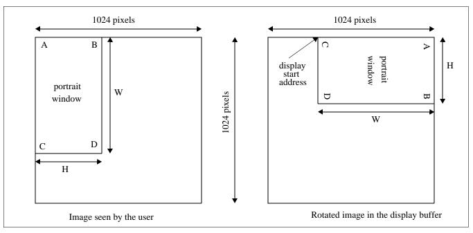
Figure 15-1: Relationship Between Screen Image and 90° Rotated Image in the Display Buffer
