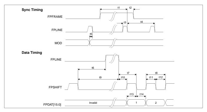
Figure 6-25: Single Color 16-Bit Panel A.C. Timing
