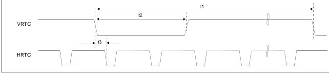
Figure 6-35: CRT A.C. Timing
