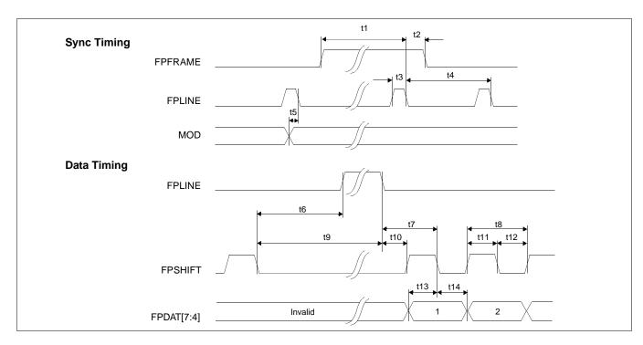
Figure 6-19: Single Color 4-Bit Panel A.C. Timing
