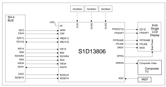
Figure 3-2: Typical System Diagram (Hitachi SH-4 Bus)
