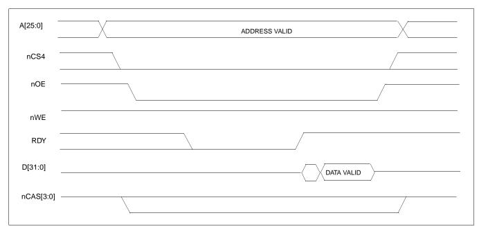
Figure 2-1: SA-1110 Variable-Latency IO Read Cycle
