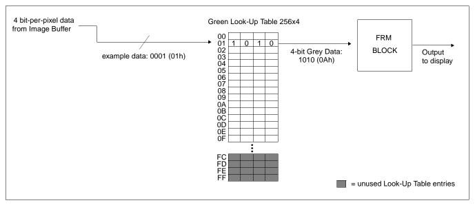
Figure 12-1: 4 Bit-Per-Pixel Monochrome Mode Data Output Path
