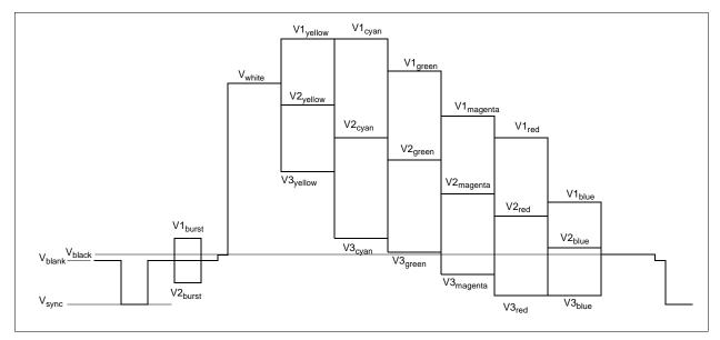
Figure 13-3: NTSC/PAL Composite Output Levels
