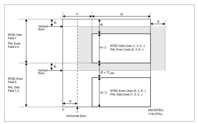
Figure 13-4: NTSC/PAL Image Positioning
