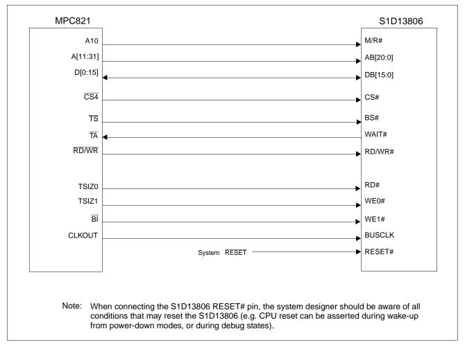
Figure 4-1: Typical Implementation of MPC821 to S1D13806 Interface
