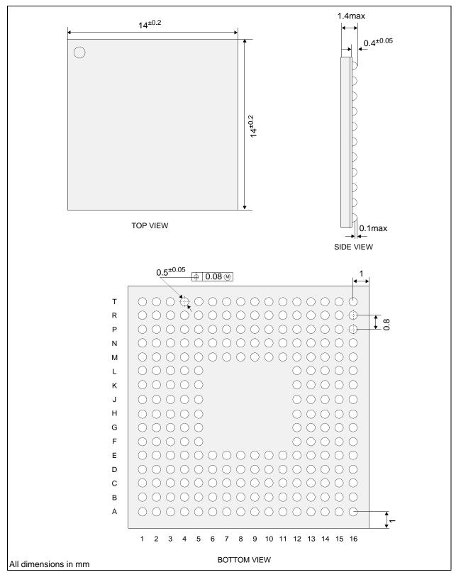
Figure 20-2: Mechanical Drawing 220-pin PFBGA
