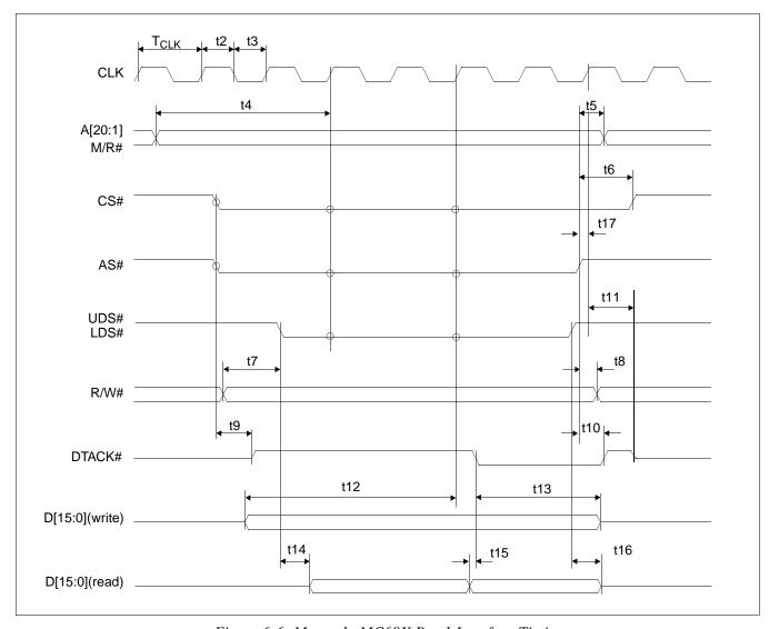
Figure 6-6: Motorola MC68K Bus 1 Interface Timing
