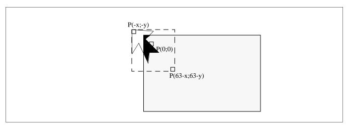
Figure 14-3: Clipped Cursor Positioning
