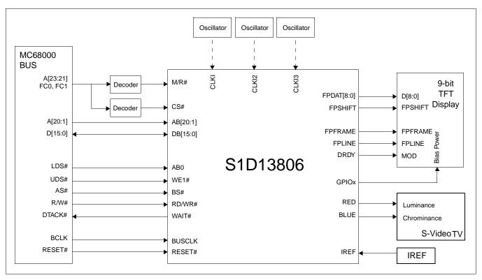
Figure 3-4: Typical System Diagram (MC68K Bus 1, Motorola 16-Bit 68000)
