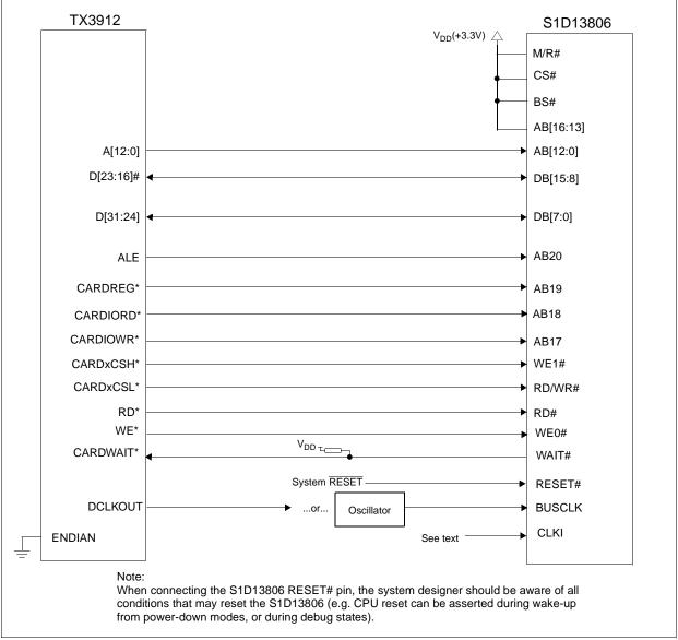
Figure 4-1: Typical Implementation of Direct Connection
