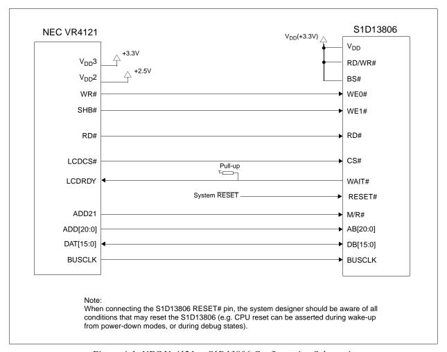
Figure 4-1: NEC VR4121 to S1D13806 Configuration Schematic
