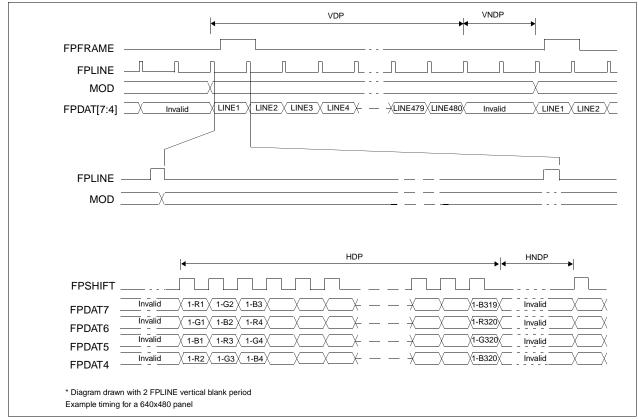
Figure 6-18: Single Color 4-Bit Panel Timing
