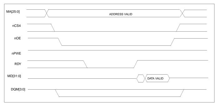
Figure 2-1 Cotulla Variable-Latency IO Read Cycle
