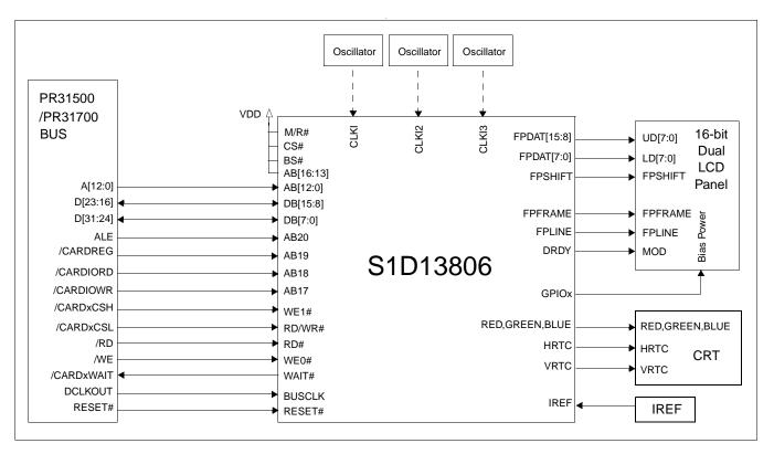
Figure 3-9: Typical System Diagram (Philips MIPS PR31500/PR31700 Bus)
