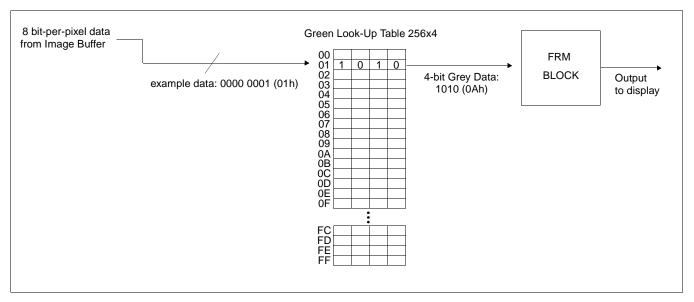
Figure 12-2: 8 Bit-Per-Pixel Monochrome Mode Data Output Path
