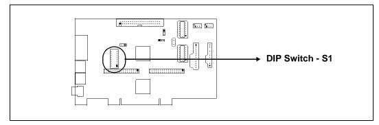
Figure 3-1: Configuration DIP Switch (S1) Location
