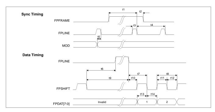
Figure 6-17: Single Monochrome 8-Bit Panel A.C. Timing
