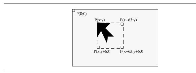
Figure 14-2: Unclipped Cursor Positioning
