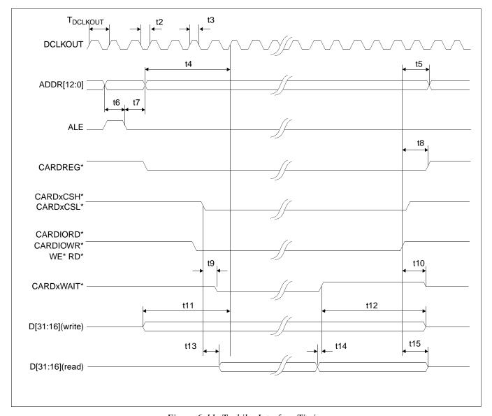
Figure 6-11: Toshiba Interface Timing
