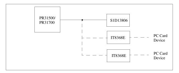
Figure 5-1: IT8368E Implementation Block Diagram
