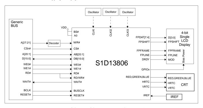
Figure 3-1: Typical System Diagram (Generic Bus)
