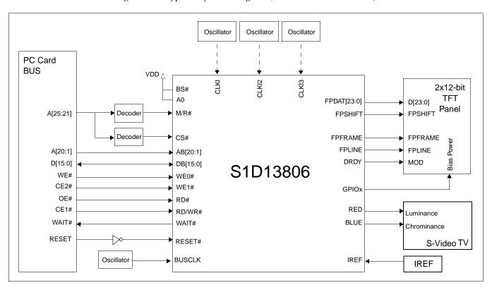
Figure 3-8: Typical System Diagram (PC Card Bus)
