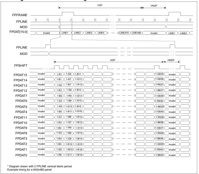
Figure 6-24: Single Color 16-Bit Panel Timing
