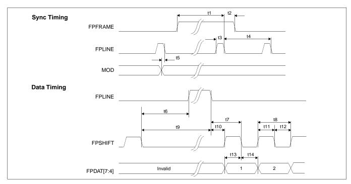
Figure 6-15: Single Monochrome 4-Bit Panel A.C. Timing
