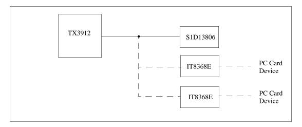
Figure 5-1: IT8368E Implementation Block Diagram
