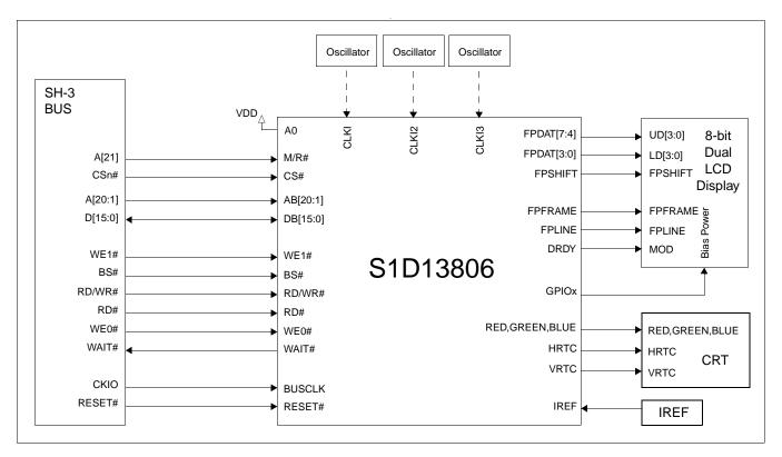
Figure 3-3: Typical System Diagram (Hitachi SH-3 Bus)
