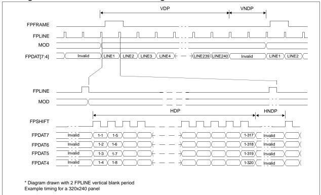
Figure 6-14: Single Monochrome 4-Bit Panel Timing
