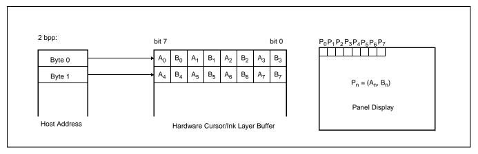
Figure 8-1: Hardware Cursor/Ink Layer Data Format
