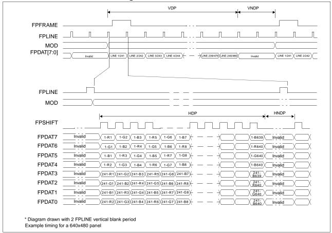
Figure 6-28: Dual Color 8-Bit Panel Timing
