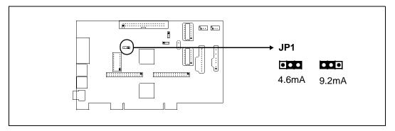
Figure 3-2: Configuration Jumper (JP1) Location
