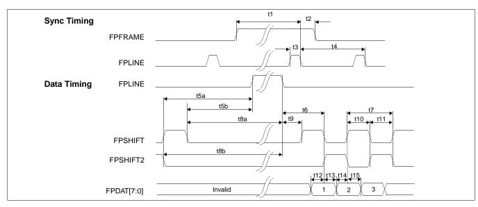
Figure 6-21: Single Color 8-Bit Panel A.C. Timing (Format 1)
