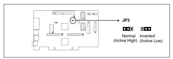
Figure 3-4: Configuration Jumper (JP3) Location
