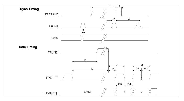
Figure 6-29: Dual Color 8-Bit Panel A.C. Timing
