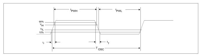
Figure 6-1: Clock Input Requirement
