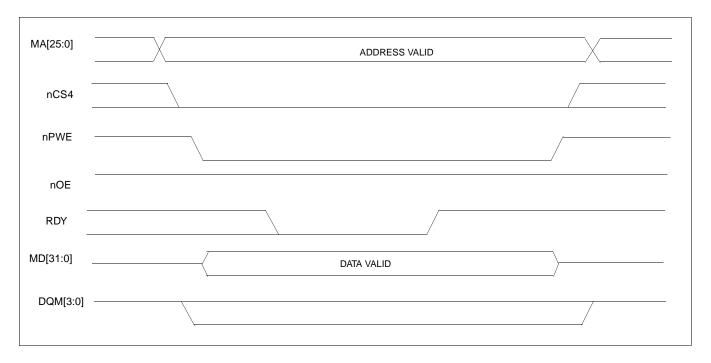
Figure 2-2 Cotulla Variable-Latency IO Write Cycle
