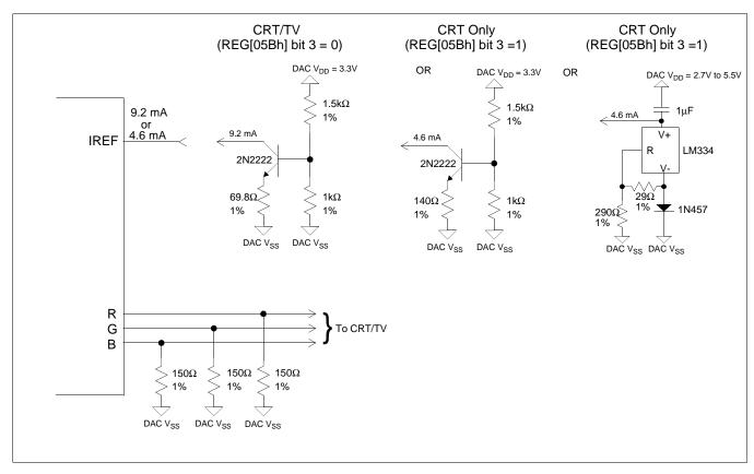
Figure 4-3: External Circuitry for CRT Interface
