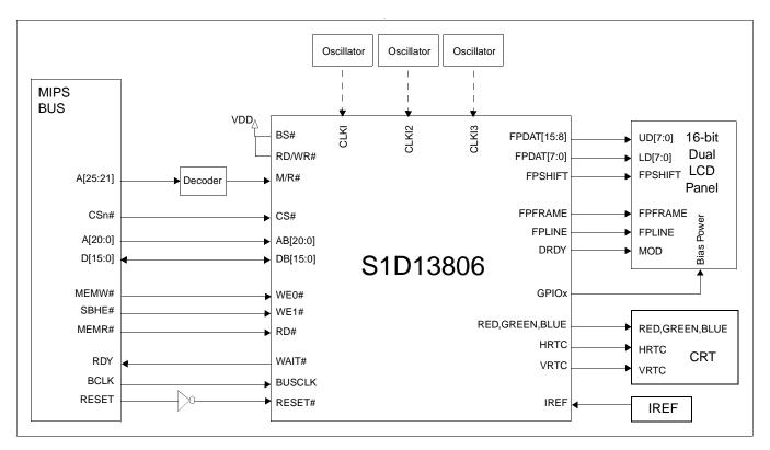
Figure 3-7: Typical System Diagram (NEC MIPS VR41xx Bus)
