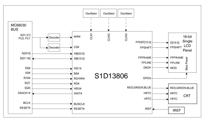
Figure 3-5: Typical System Diagram (MC68K Bus 2, Motorola 32-Bit 68030)
