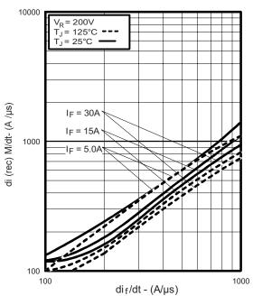
Fig. 8 - Typical dI<sub>(rec)M</sub>/dt vs. dI<sub>F</sub>/dt (Per Leg)
