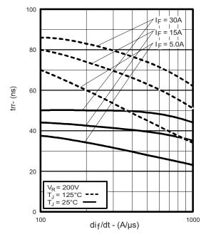
Fig. 5 - Typical Reverse Recovery Time vs. dI<sub>F</sub>/dt (Per Leg)
