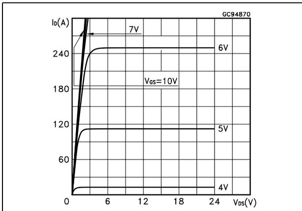
Figure 4. Transfer characteristics
