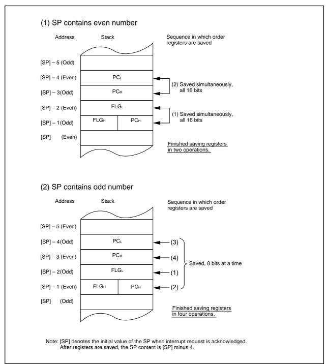
Figure 2.7.7. Operation of Saving Register
