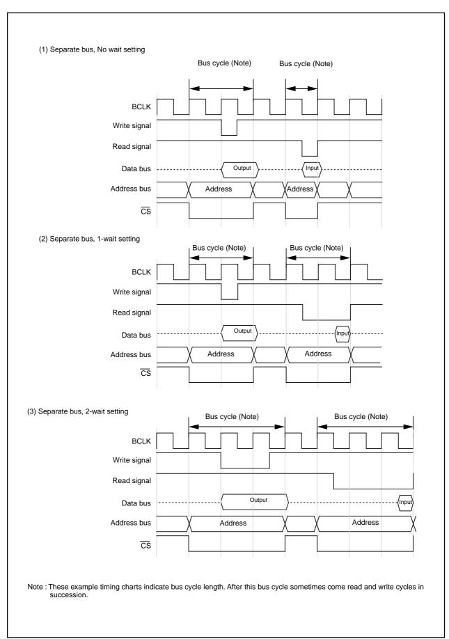
Figure 2.4.12. Typical Bus Timings Using Software Wait (1)
