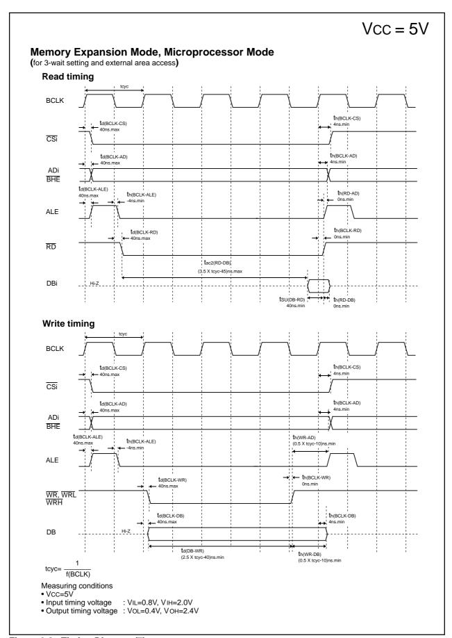
Figure 3.8. Timing Diagram (7)
