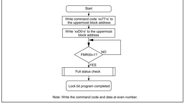
Figure 4.3.3. Lock Bit Program Command
