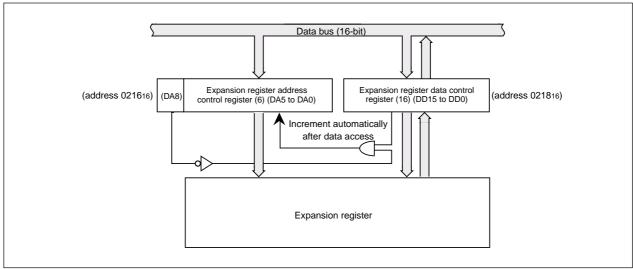
Figure 2.14.10 Expansion register access block diagram
