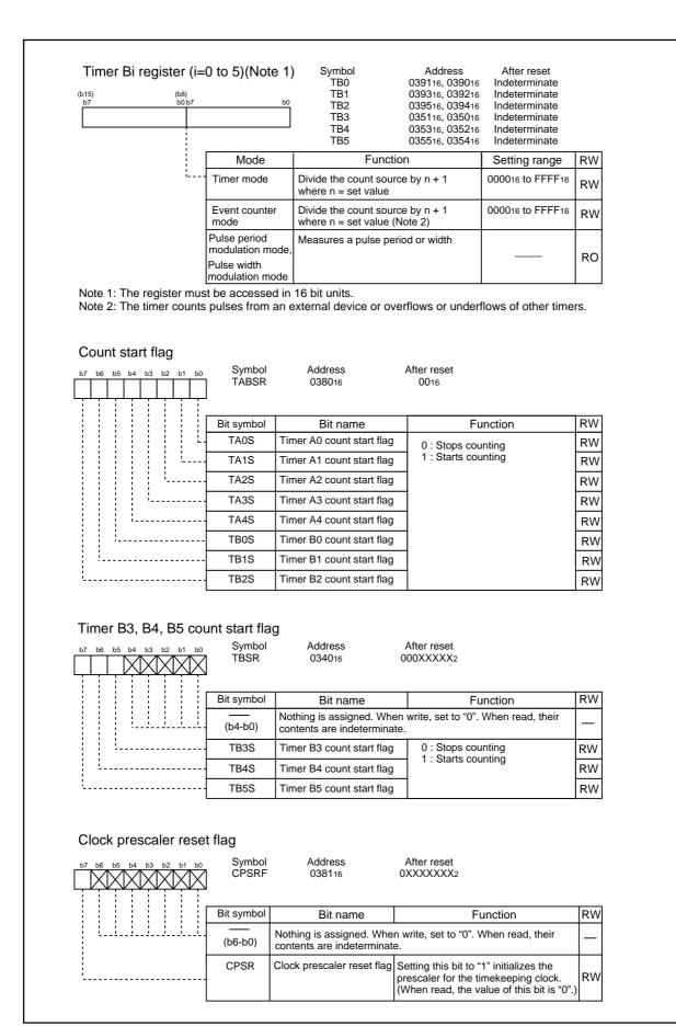
Figure 2.10.16. TB0 to TB5 Registers, TABSR Register, TBSR Register, CPSRF Register
