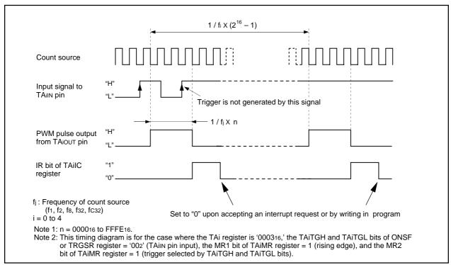
Figure 2.10.12. Example of 16-bit Pulse Width Modulator Operation
