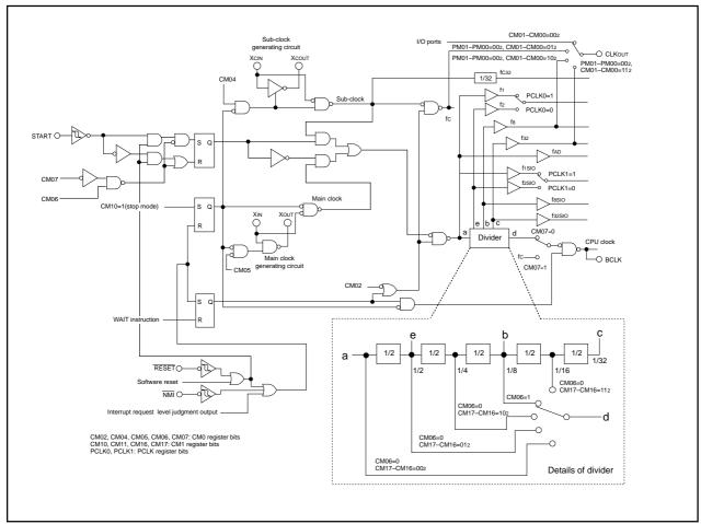
Figure 2.5.1. Clock Generation Circuit
