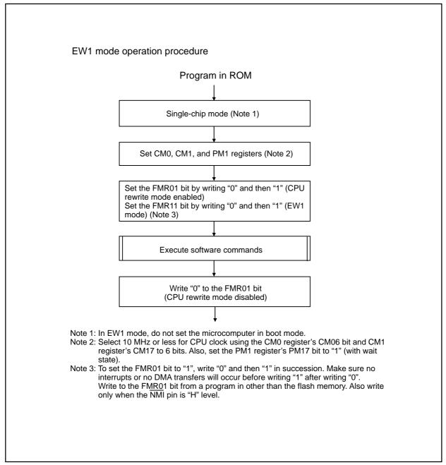
Figure 4.2.6. Setting and Resetting of EW1 Mode
