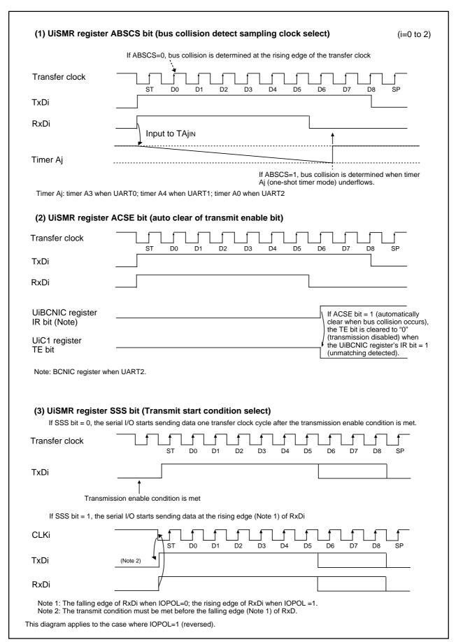
Figure 2.11.29. Bus Collision Detect Function-Related Bits
