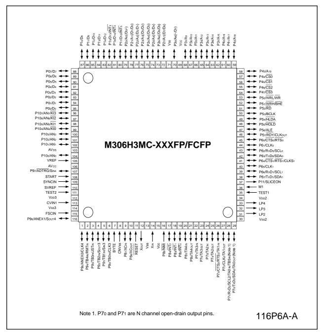
Figure 1.3.1 Pin configuration (top view)
