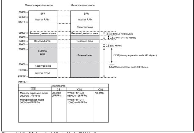
Figure 2.4.7. CS Area in 1 Mbyte Mode (PM13=1)
