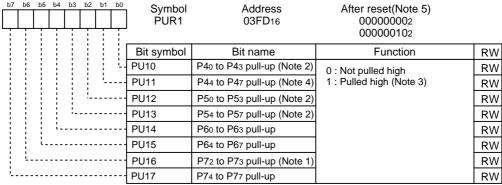
Note 1: The P70 and P71 pins do not have pull-ups.
