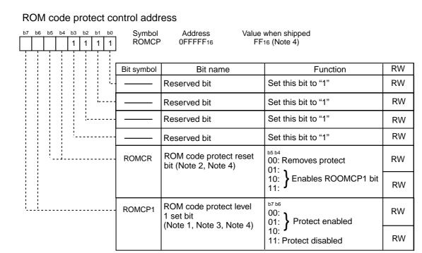
Note 1: If the ROMCR bits are set to other than '002' <u>and</u> the ROMCP1 bits are set to other than '112' (
