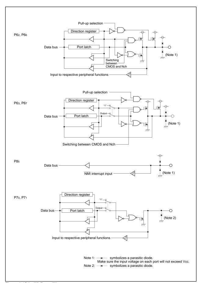
Figure 2.15.3. I/O Ports (3)
