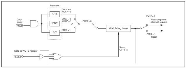
Figure 2.8.1. Watchdog Timer Block Diagram
