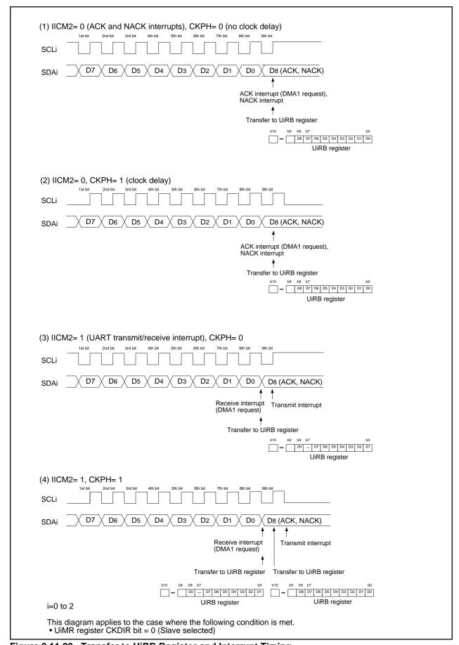
Figure 2.11.22. Transfer to UiRB Register and Interrupt Timing
