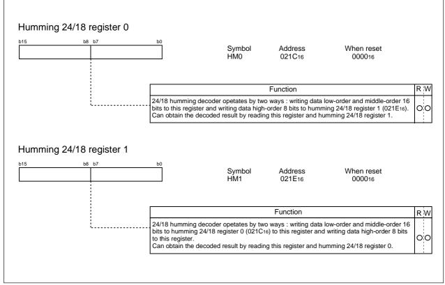
Figure 2.14.20 Humming 24/18 register composition
