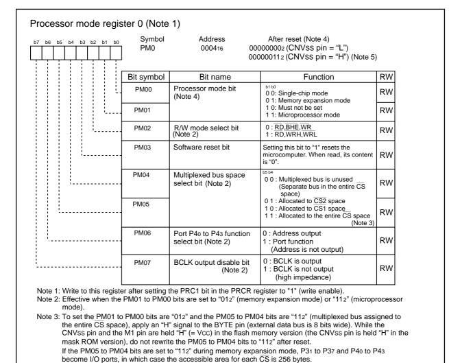
Note 4: The PM01 to PM00 bits do not change at software reset, watchdog timer reset and oscillation stop
