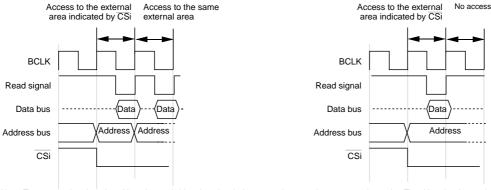
Note: These examples show the address bus and chip select signal when accessing areas in two successive cycles. The chip select bus cycle may be extended more than two cycles depending on a combination of these examples.
