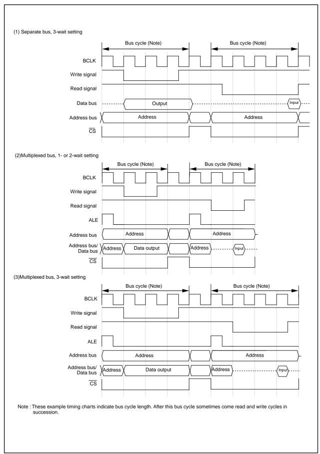
Figure 2.4.13. Typical Bus Timings Using Software Wait (2)
