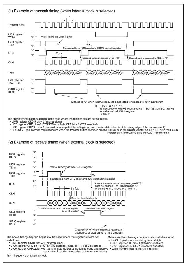
Figure 2.11.9. Transmit and Receive Operation
