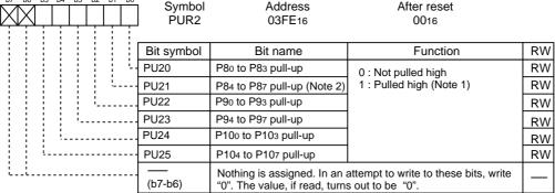
Note 1: The pin for which this bit is "1" (pulled high) and the direction bit is "0" (input mode) is pulled high. Note 2: The P85 pin does not have pull-up.
