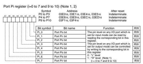
Note 1: Since P7 $_{0}$  and P7 $_{1}$  are N-channel open drain ports, the data is high-impedance.
