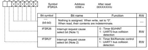
Note 1: Timer B3/HINT and UART0 bus collision detection share the vector and interrupt control register. When using the timer B3/HINT interrupt, clear the IFSR26 bit to "0" (timer B3/HINT). When using UART0 bus collision detection, set the IFSR26 bit to "1".
