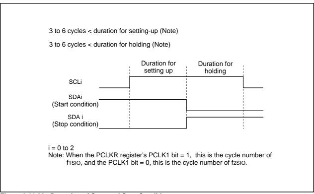
Figure 2.11.23. Detection of Start and Stop Condition
