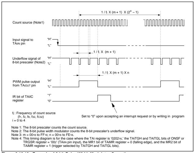
Figure 2.10.13. Example of 8-bit Pulse Width Modulator Operation
