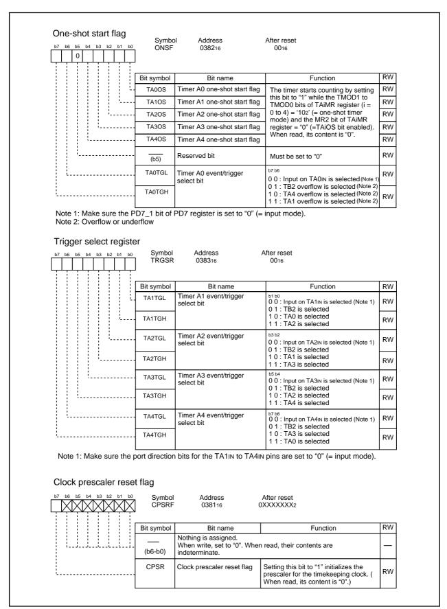
Figure 2.10.6. ONSF Register, TRGSR Register, and CPSRF Register
