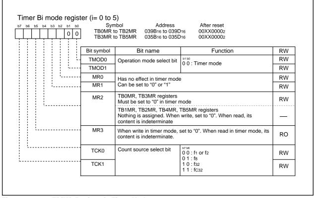
Figure 2.10.17. TBiMR Register in Timer Mode
