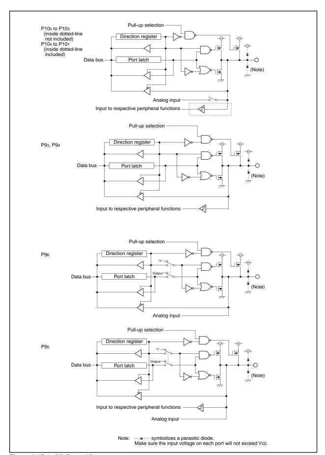
Figure 2.15.4. I/O Ports (4)
