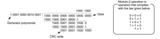
The value "0001 0001 1000 10012 (118916)" derived from the remainder "1001 0001 1000 10002 (918816)" by reversing its bit positions may be read from the CRCD register.
