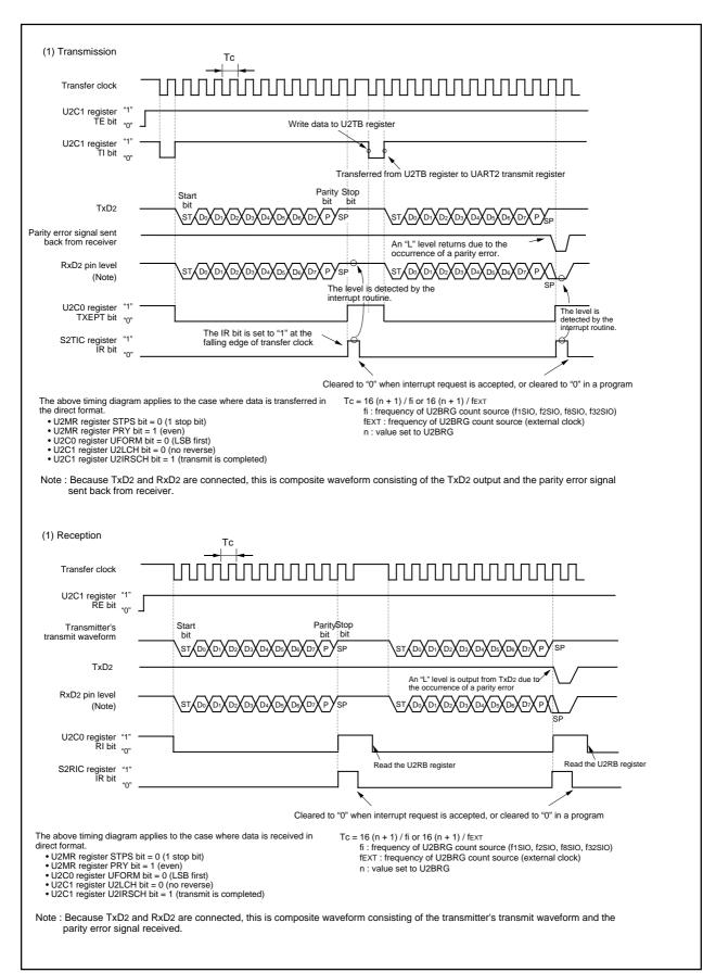
Figure 2.11.30. Transmit and Receive Timing in SIM Mode
