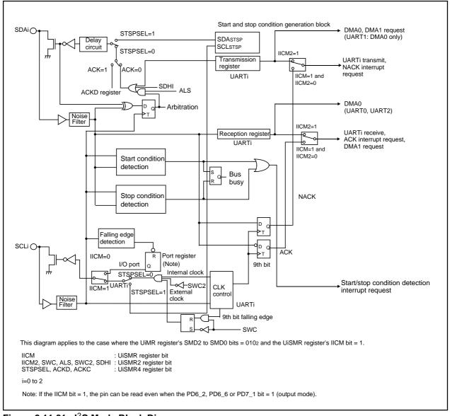
Figure 2.11.21. I<sup>2</sup>C Mode Block Diagram
