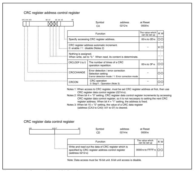
Figure 2.14.5 Composition of CRC register access related register
