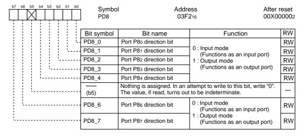
Figure 2.15.7. PD0 to PD10 Registers
