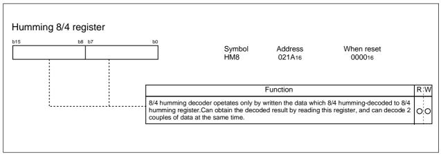
Figure 2.14.18 Humming 8/4 register composition
