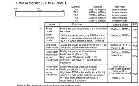
Note 1: The register must be accessed in 16 bit units.
