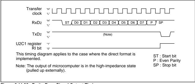
Figure 2.11.32. Parity Error Signal Output Timing
