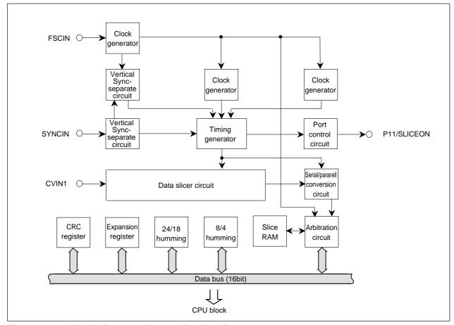
Figure 2.14.1 Block diagram of expansion function
