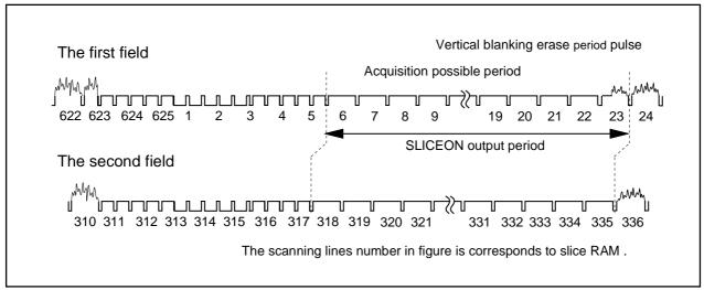
Figure 2.14.11 Acquisition timing
