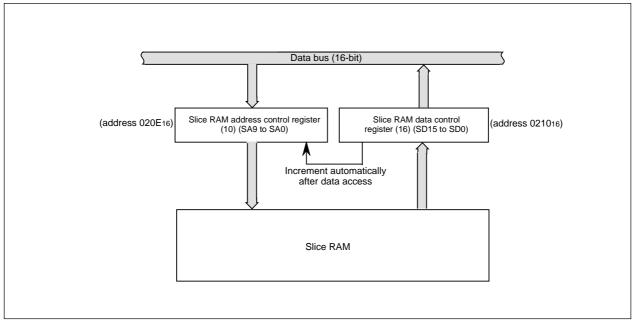
Figure 2.14.4 Slice RAM access block diagram
