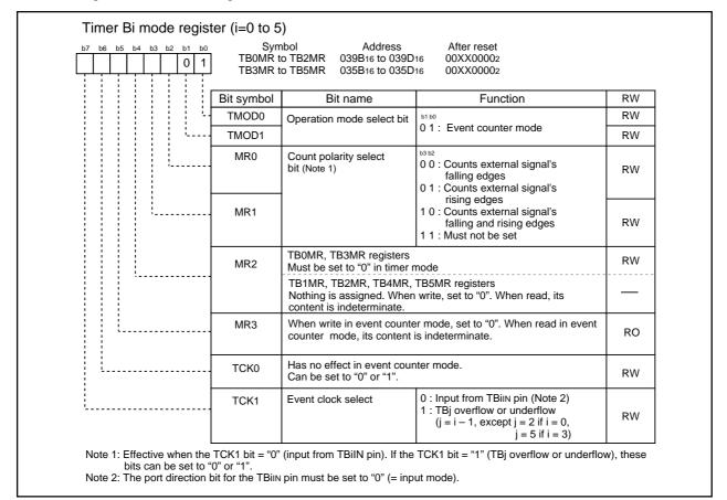
Figure 2.10.20. TBiMR Register in Event Counter Mode
