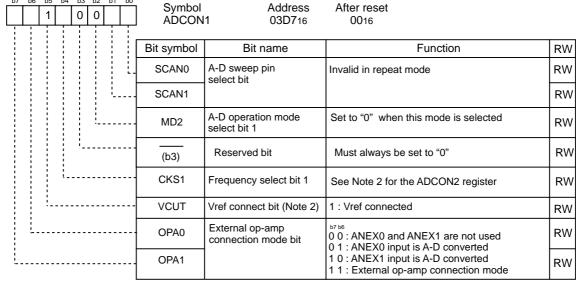
Note 1: If the ADCON1 register is rewritten during A-D conversion, the conversion result will be indeterminate.
