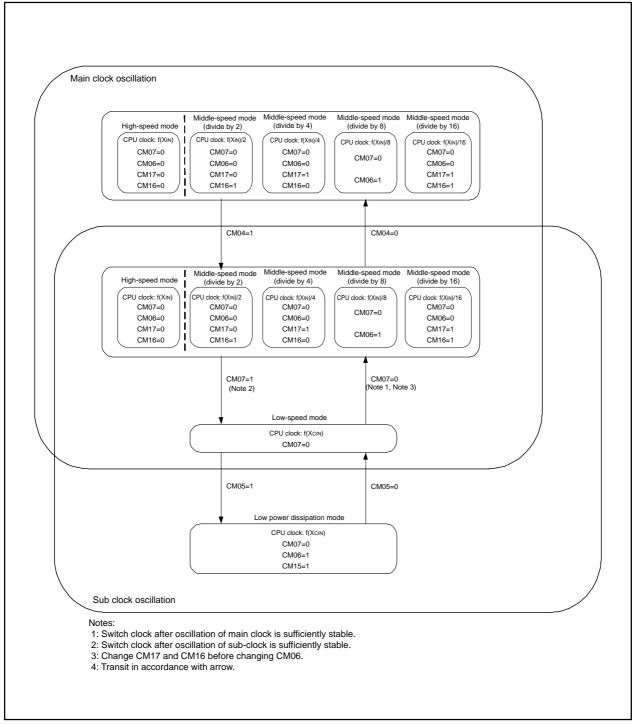
Figure 2.5.9. State Transition in Normal Mode
