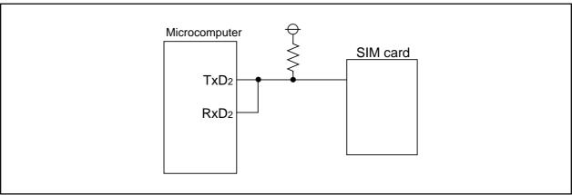
Figure 2.11.31. SIM Interface Connection
