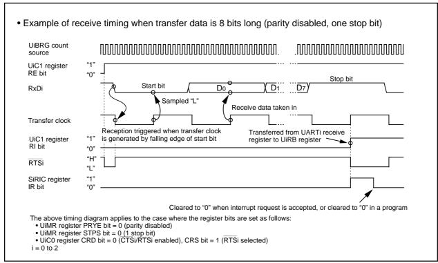
Figure 2.11.16. Receive Operation
