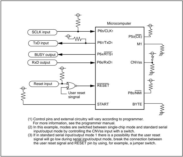
Figure 4.3.7. Circuit Application in Standard Serial I/O Mode 1
