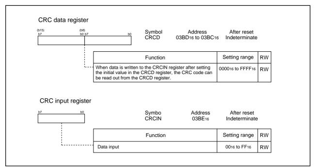
Figure 2.13.2. CRCD Register and CRCIN Register
