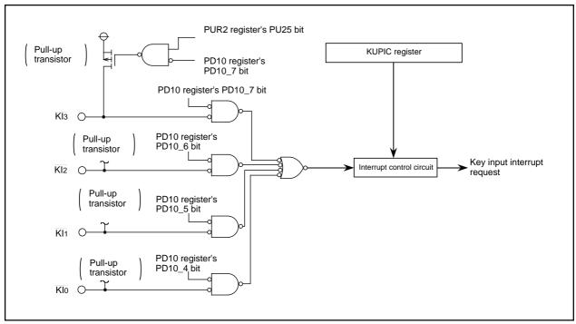
Figure 2.7.11. Key Input Interrupt
