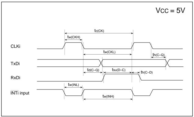
Figure 3.3. Timing Diagram (2)
