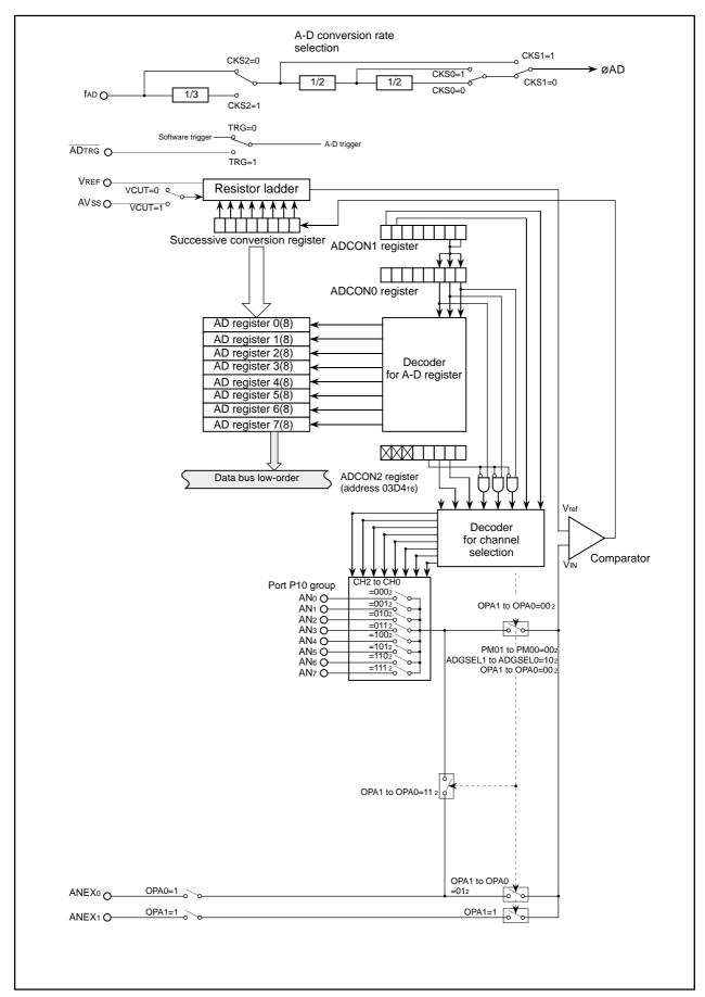
Figure 2.12.1. A-D Converter Block Diagram
