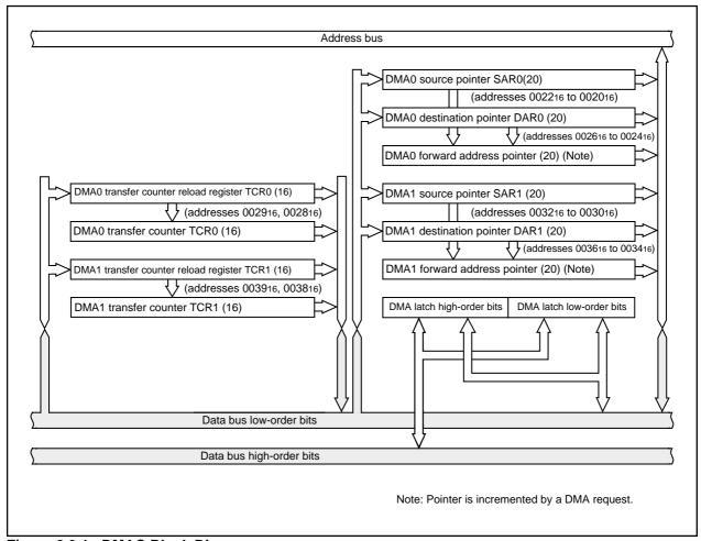
Figure 2.9.1. DMAC Block Diagram
