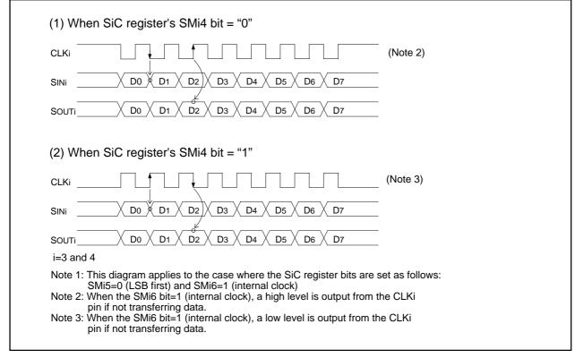
Figure 2.11.37. Polarity of Transfer Clock
