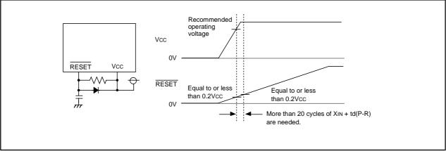
Figure 2.3.1. Example Reset Circuit
