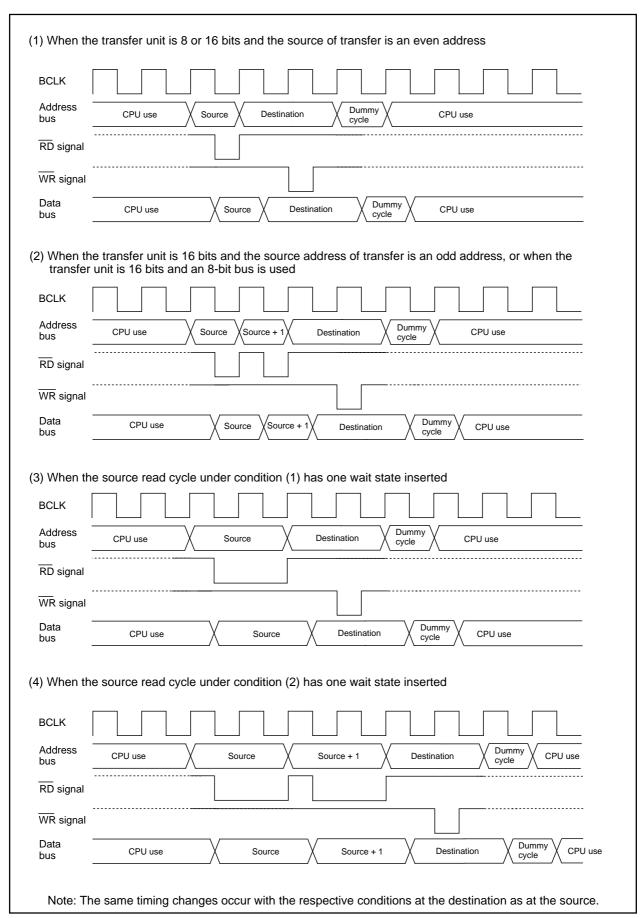
Figure 2.9.5. Transfer Cycles for Source Read
