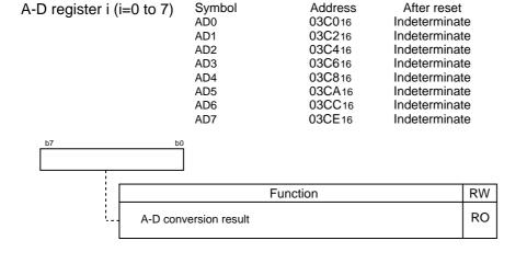
Figure 2.12.3. ADCON2 Register, and AD0 to AD7 Registers
