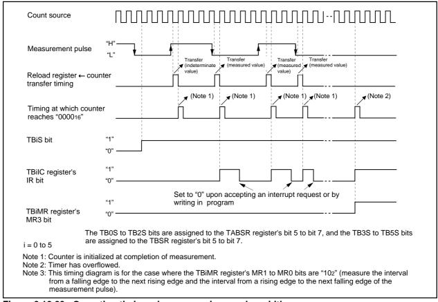
Figure 2.10.23. Operation timing when measuring a pulse width
