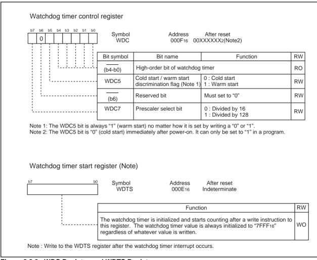
Figure 2.8.2. WDC Register and WDTS Register
