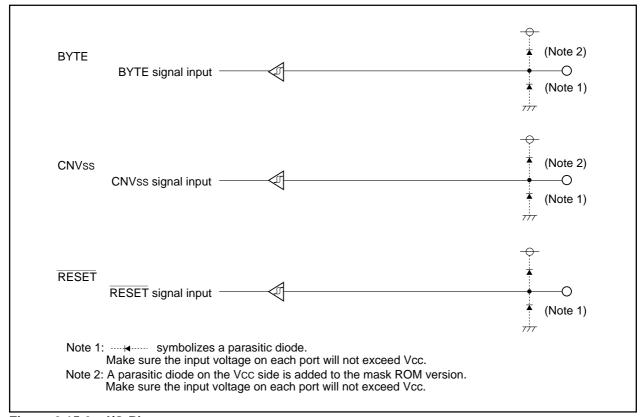
Figure 2.15.6. I/O Pins
