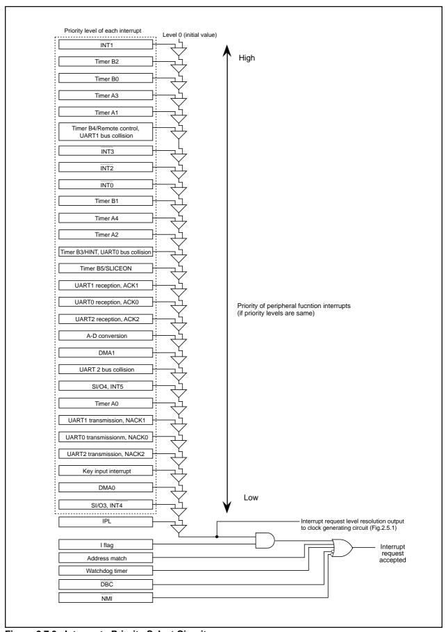
Figure 2.7.9. Interrupts Priority Select Circuit
