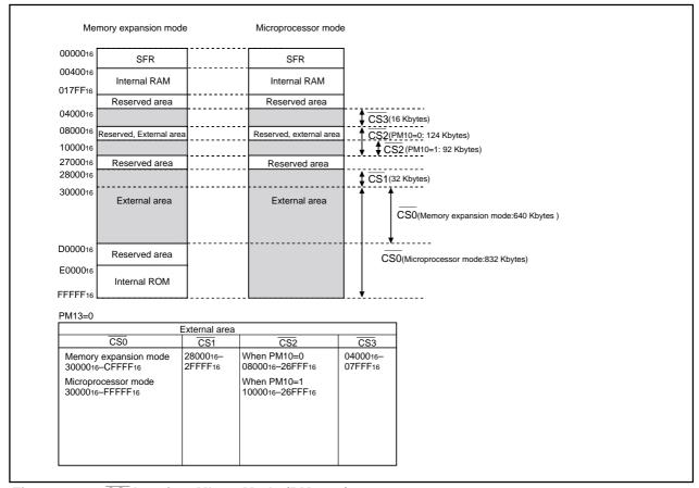
Figure 2.4.6. CS Area in 1 Mbyte Mode (PM13=0)
