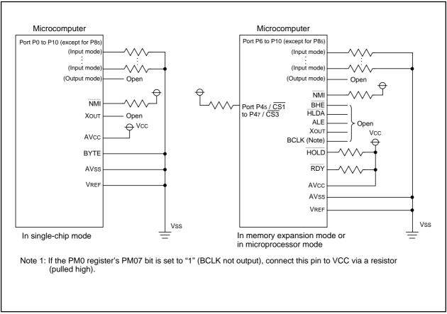
Figure 2.15.11. Unassigned Pins Handling
