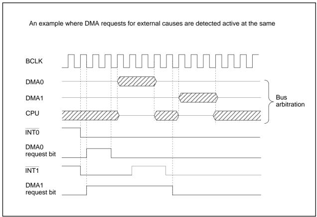
Figure 2.9.6. DMA Transfer by External Factors
