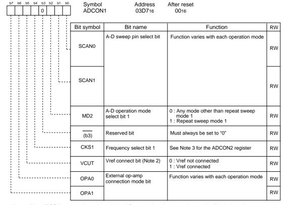
Note 1: If the ADCON1 register is rewritten during A-D conversion, the conversion result will be indeterminate.
