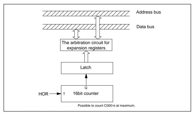
Figure 2.14.12 Block diagram of Synchronized detection circuit
