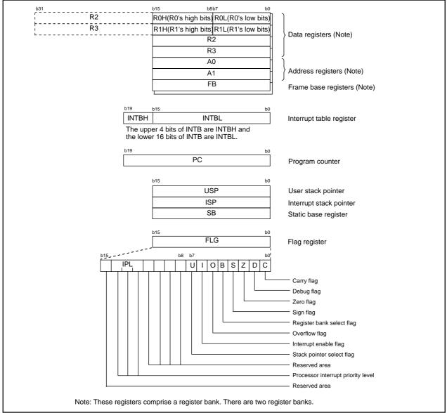
Figure 2.2.1. Central Processing Unit Register
