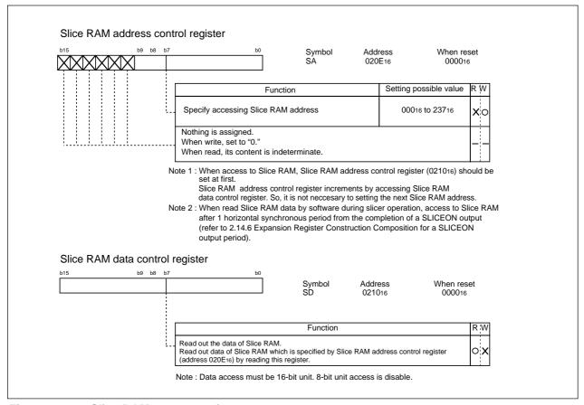
Figure 2.14.3 Slice RAM access registers
