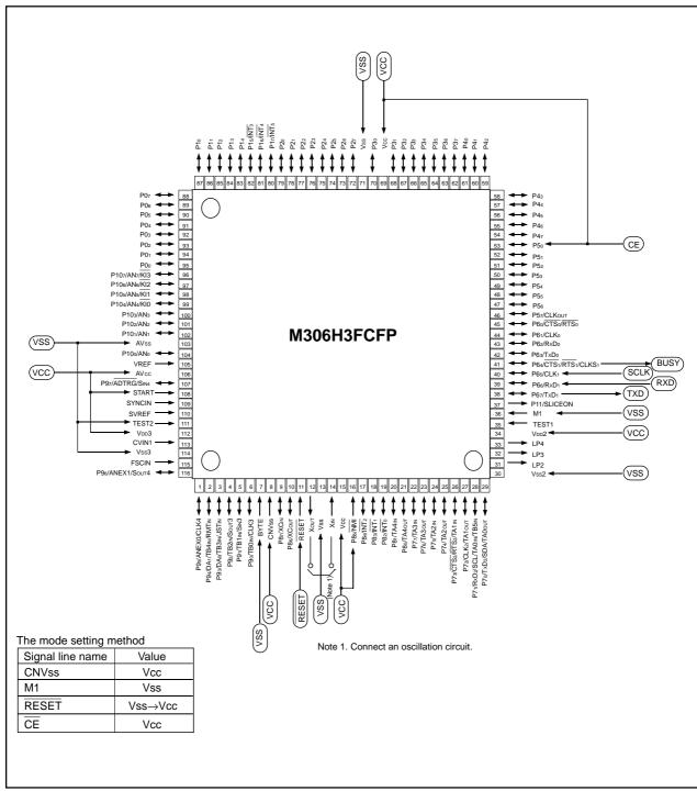
Figure 4.3.6. Pin Connections for Serial I/O Mode
