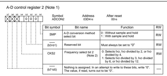
Note 1: If the ADCON2 register is rewritten during A-D conversion, the conversion result will be indeterminate.
