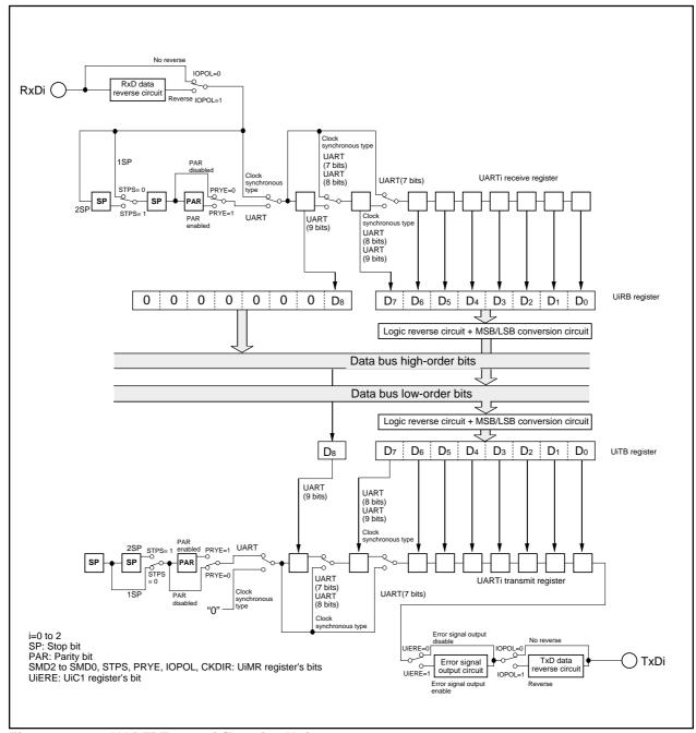
Figure 2.11.2. UARTi Transmit/Receive Unit
