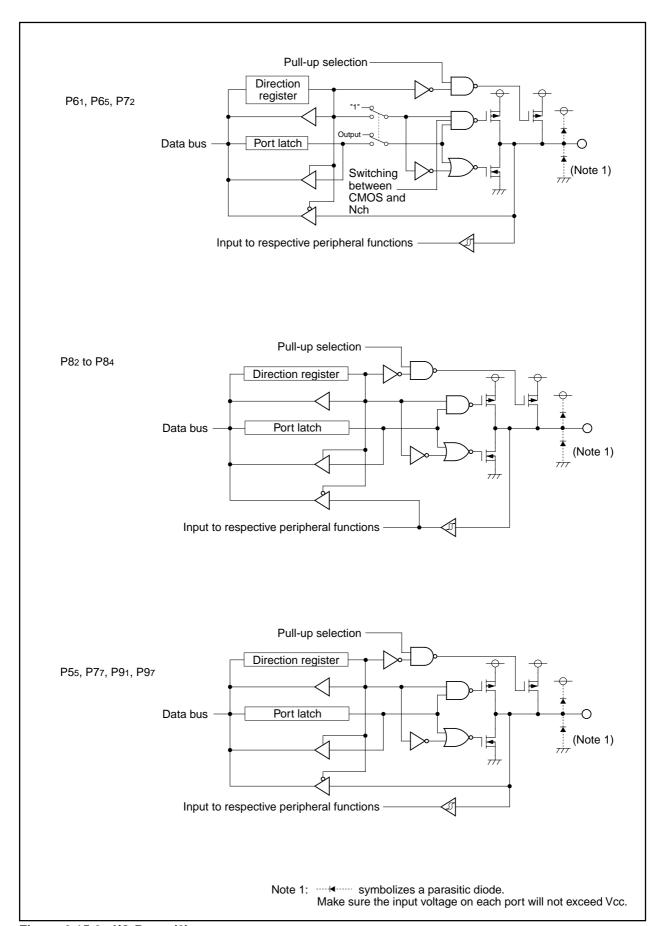
Figure 2.15.2. I/O Ports (2)
