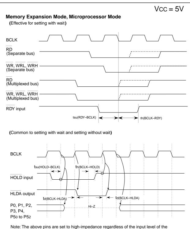
Note: The above pins are set to high-impedance regardless of the input level of the BYTE pin, PM06 bit in PM0 register and PM11 bit in PM1 register.
