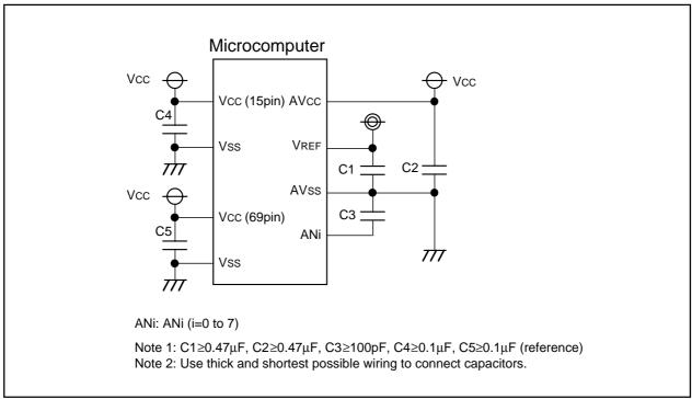
Figure 6.2. Use of capacitors to reduce noise
