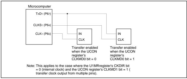
Figure 2.11.13. Transfer Clock Output From Multiple Pins
