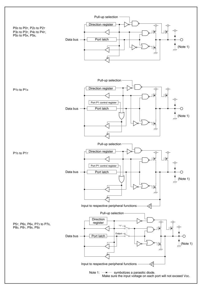
Figure 2.15.1. I/O Ports (1)
