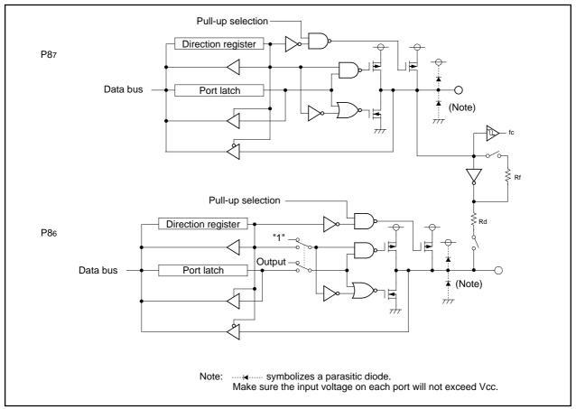
Figure 2.15.5. I/O Ports (5)
