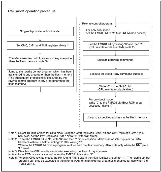
Figure 4.2.5. Setting and Tesetting of EW0 Mode
