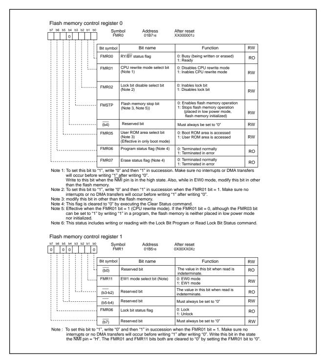
Figure 4.2.4. FIDR Register and FMR0 and FMR1 Registers
