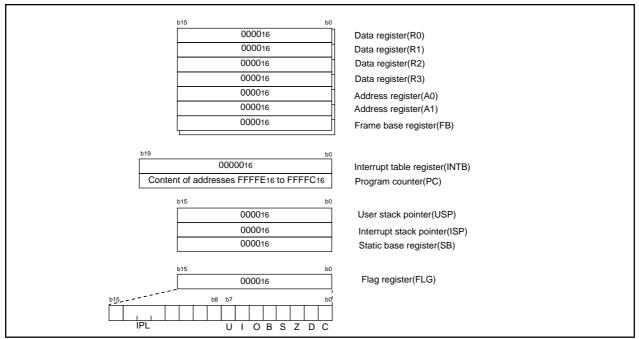
Figure 2.3.3. CPU Register Status After Rreset
