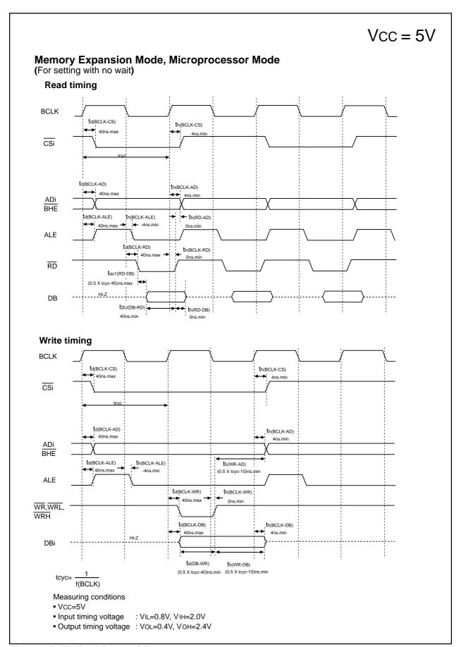
Figure 3.5. Timing Diagram (4)
