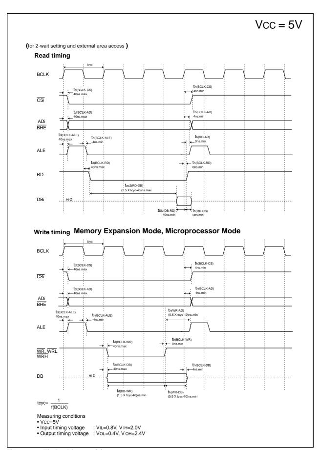
Figure 3.7. Timing Diagram (6)
