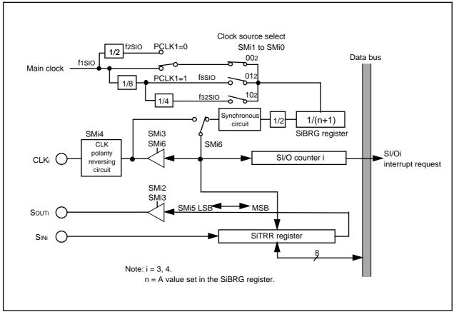
Figure 2.11.34. SI/O3 and SI/O4 Block Diagram
