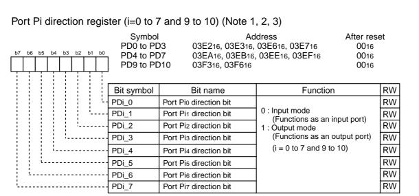
Note 1: Make sure the PD9 register is written to by the next instruction after setting the PRCR register's PRC2 bit to "1" (write enabled).
