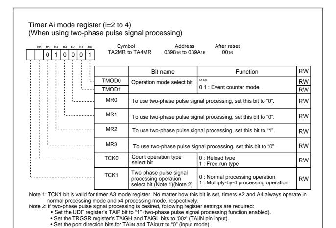
Figure 2.10.9. TA2MR to TA4MR Registers in Event Counter Mode (when using two-phase pulse signal processing with timer A2, A3 or A4)
