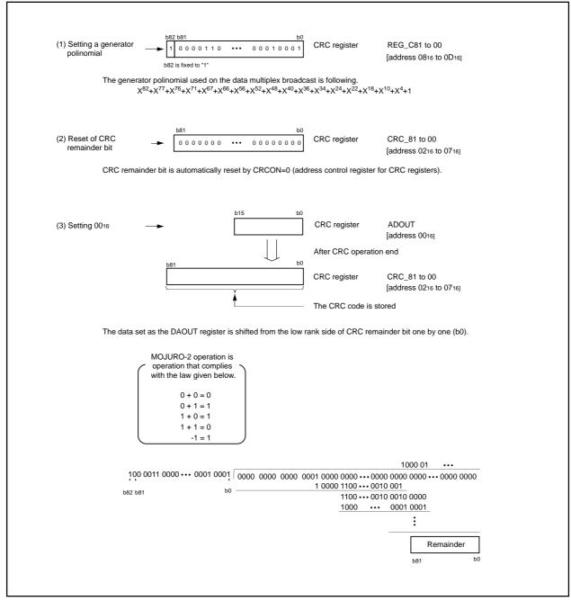
Figure 2.14.7 Example of operation of CRC operation circuit
