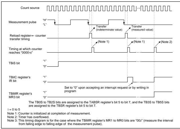
Figure 2.10.22. Operation timing when measuring a pulse period
