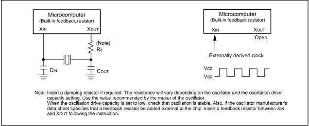
Figure 2.5.5. Examples of Main Clock Connection Circuit
