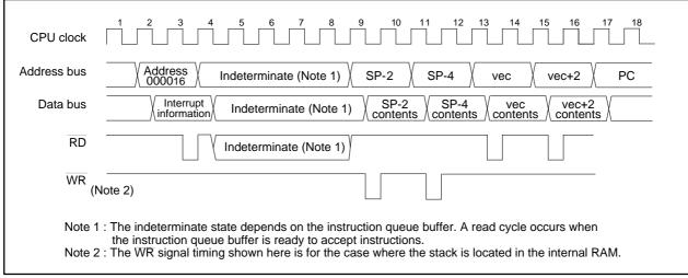
Figure 2.7.4. Time Required for Executing Interrupt Sequence
