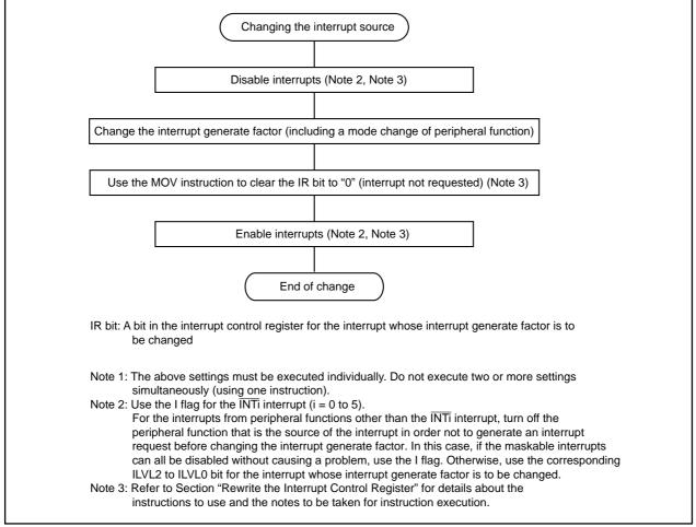
Figure 6.1. Procedure for Changing the Interrupt Generate Factor
