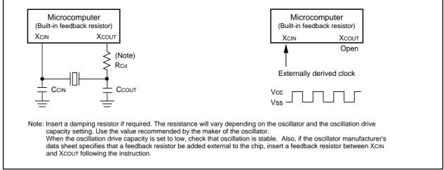
Figure 2.5.6. Examples of Sub Clock Connection Circuit
