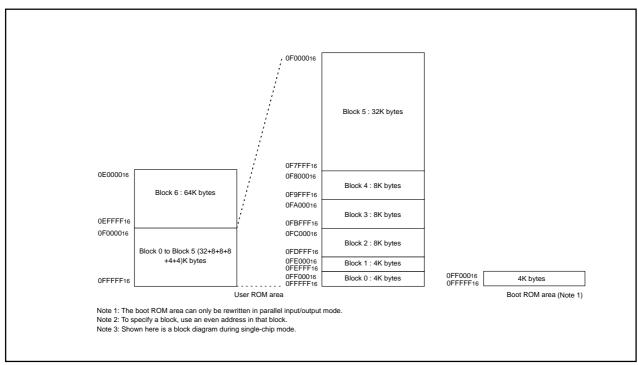
Figure 4.2.1. Flash Memory Block Diagram
