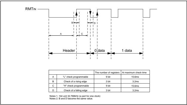
Figure 2.14.15 Example of waveform of pattern matching
