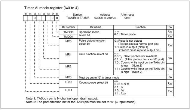
Figure 2.10.7. Timer Ai Mode Register in Timer Mode
