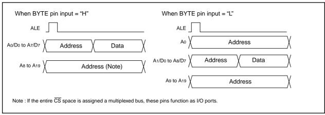
Figure 2.4.8. ALE Signal, Address Bus, Data Bus
