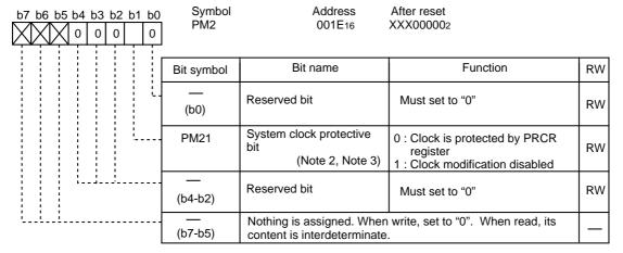
Note 1: Write to this register after setting the PRC1 bit of PRCR register to "1" (write enable).
