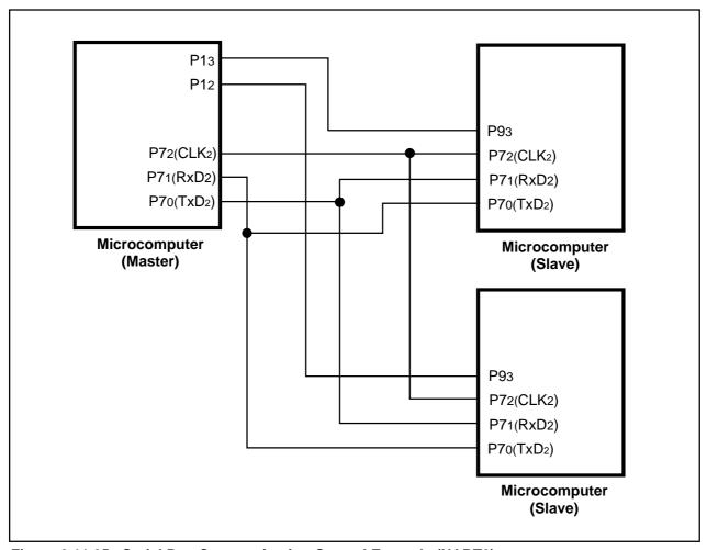
Figure 2.11.25. Serial Bus Communication Control Example (UART2)
