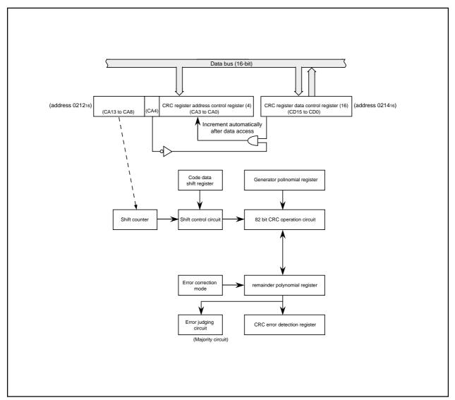
Figure 2.14.6 Access block diagram for CRC registers
