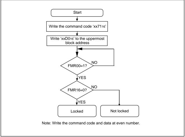
Figure 4.3.4. Read Lock Bit Status Command
