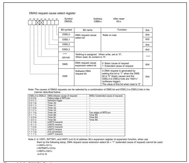
Figure 2.9.2. DM0SL Register
