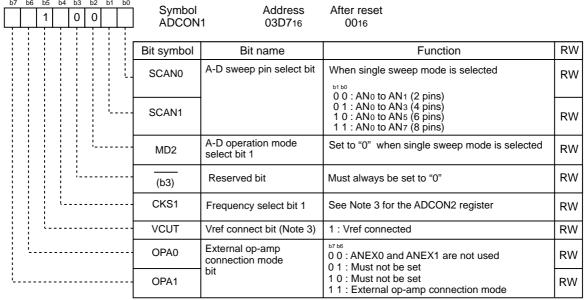
Note 1: If the ADCON1 register is rewritten during A-D conversion, the conversion result will be indeterminate. Note 2: If the VCUT bit is reset from "0" (Vref unconnected) to "1" (Vref connected), wait for 1 µs or more before starting A-D conversion.
