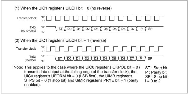
Figure 2.11.18. Serial Data Logic Switching
