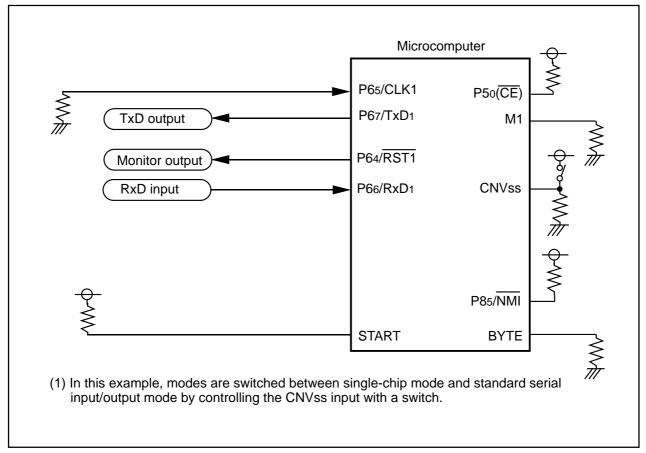
Figure 4.3.8. Circuit Application in Standard Serial I/o Mode 2
