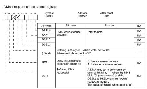
Note: The causes of DMA1 requests can be selected by a combination of DMS bit and DSEL3 to DSEL0 bits in the manner described below.
