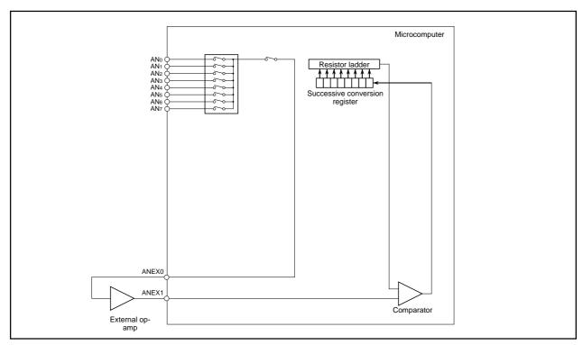
Figure 2.12.9. External Op-amp Connection
