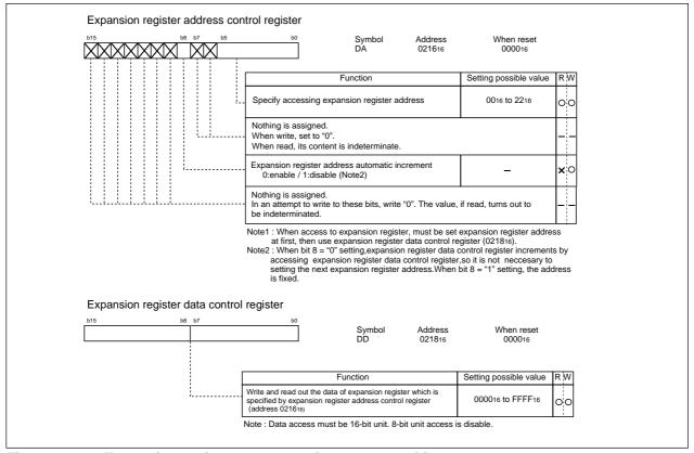
Figure 2.14.9 Expansion register access registers composition
