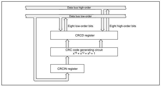
Figure 2.13.1. CRC Circuit Block Diagram
