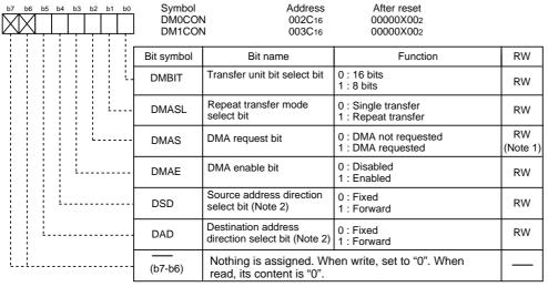
Note 1: The DMAS bit can be set to "0" by writing "0" in a program (This bit remains unchanged even if "1" is written). Note 2: At least one of the DAD and DSD bits must be "0" (address direction fixed).
