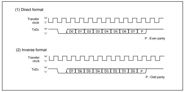
Figure 2.11.33. SIM Interface Format
