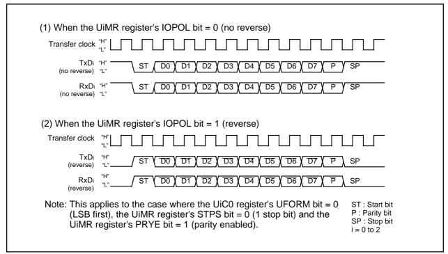
Figure 2.11.19. TxD and RxD I/O Polarity Inverse
