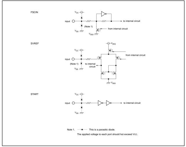
Figure 2.14.23 Pins for expansion memory (2)
