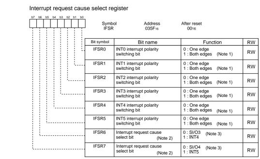
Note 1: When setting this bit to "1" (= both edges), make sure the INT0IC to INT5IC register's POL bit is set to "0" (= falling edge).
