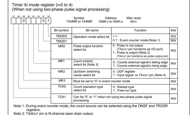
Figure 2.10.8. TAiMR Register in Event Counter Mode (when not using two-phase pulse signal processing)
