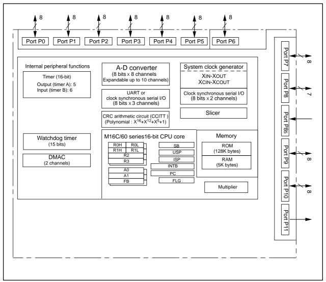
Figure 1.5.1 Block diagram
